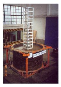
Figure 1-8 Photograph of a prototype model for the shaking table test. (Lu et al. 2004)
