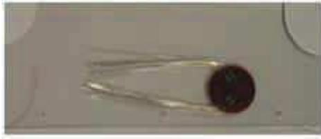
**Biaxial strain gauges (2mm):**
