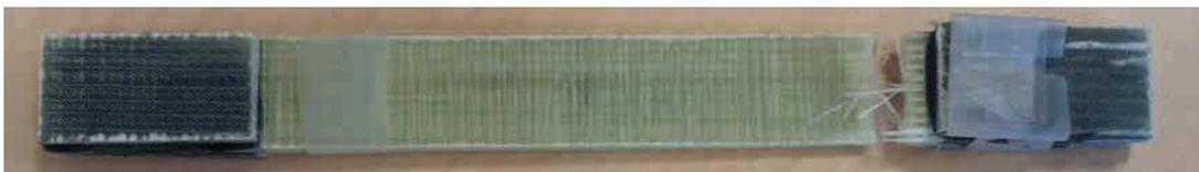
(a) Unidirectional specimen loaded at  $90^\circ$  to the fiber direction for determining " $E_t$ "
