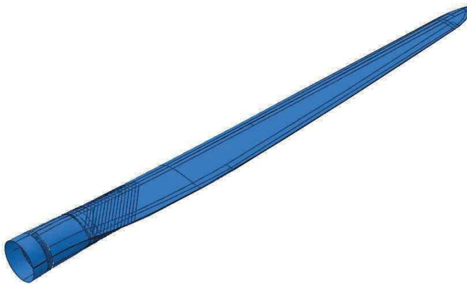
Figure 7-36: Imported and partitioned geometry in ABAQUS for FE analysis.
