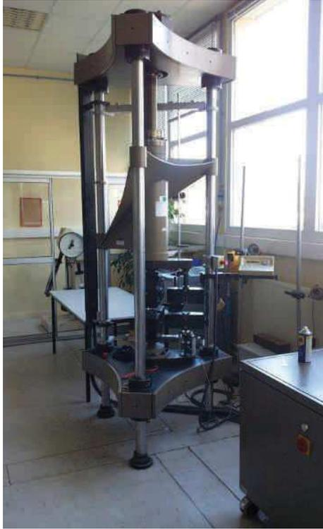
***UTS tri-column screw type tensile test machine (250kN):***
