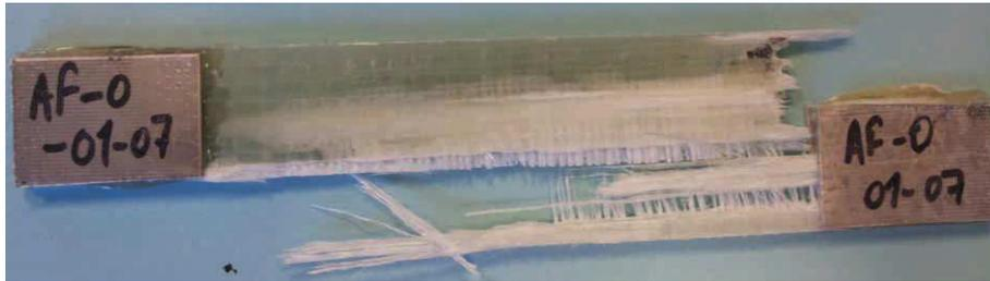
Figure 6-19: Failed 0° UD specimen showing fiber breakage and fiber pullout.
