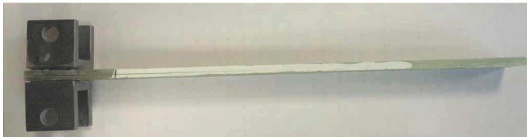
Figure 4-2: DCB specimen used for Mode I fracture resistance tests.
