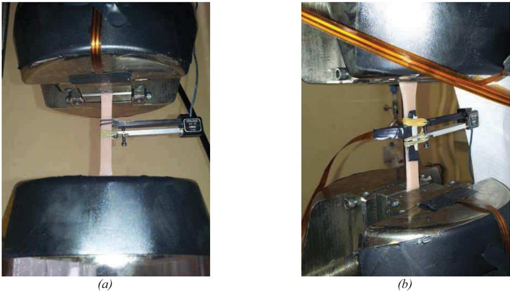
Figure 6-26: NORPOL Specimens instrumented with extensometers
