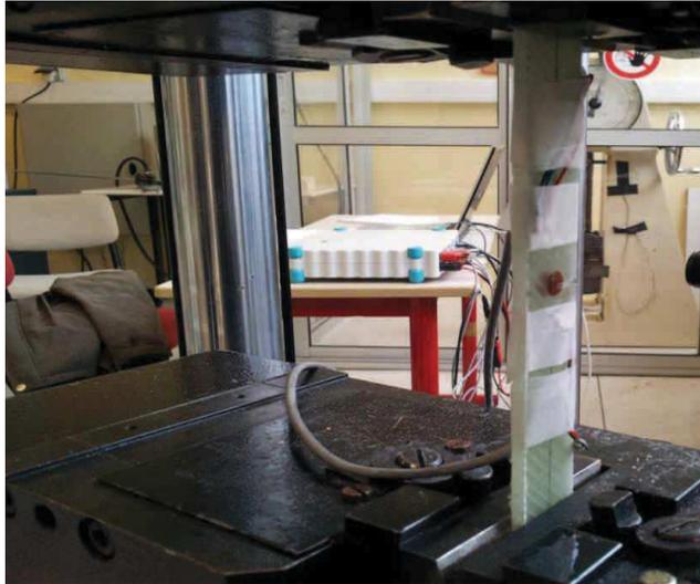
Figure 3-6: A composite specimen loaded into the UTS tensile test machine, instrumented with a biaxial strain gauge for the measurement of longitudinal and transverse strains.
