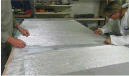
(a) Composite layers being laid out
