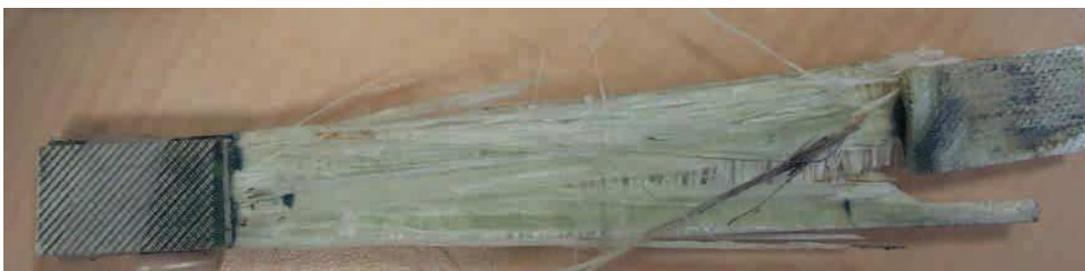
(c) Unidirectional specimen loaded at  $0^\circ$  to the fiber direction for determining " $E_l$ "
