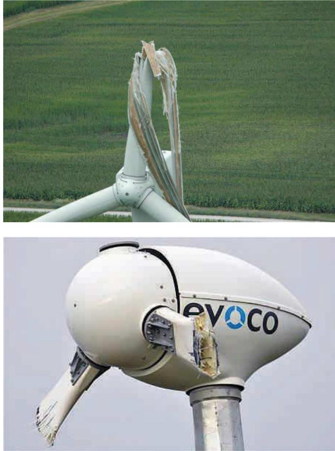
Figure 1-17: Some failed wind turbine blades during their service.
