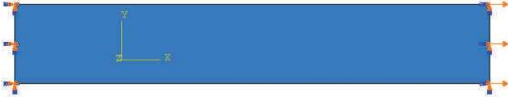
Figure 7-6: Boundary conditions of the finite element model; Left edge fixed, right end being pulled with the help of a fixed displacement.
