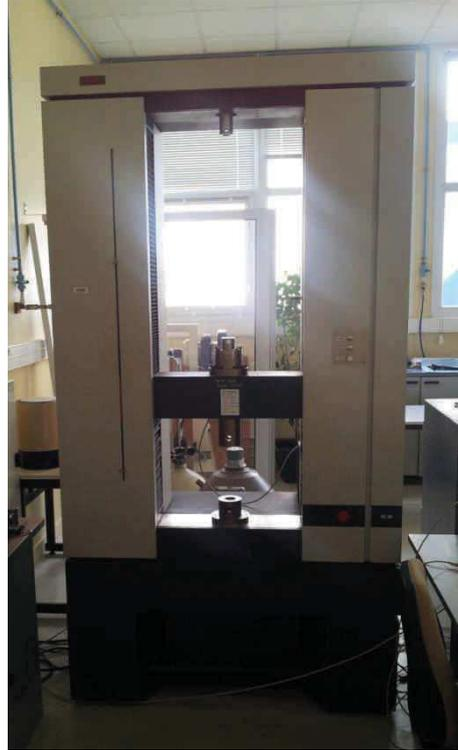
***Adamel bi-screw type tensile test machine (50kN):***
