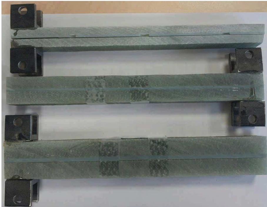
(c) Bonded composite beams
