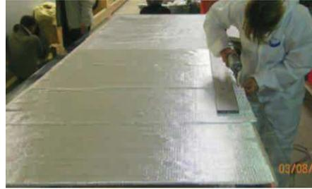
(b) Sizing of the layers after layup to +25mm of final size
