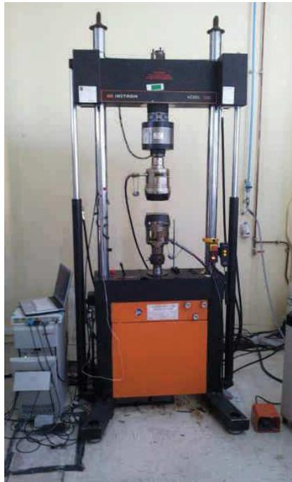
***Instron hydraulic fatigue test machine (150kN):***
