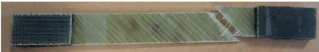
(b) Unidirectional specimen loaded at  $45^\circ$  to the fiber direction for determining " $G_{lt}$ "
