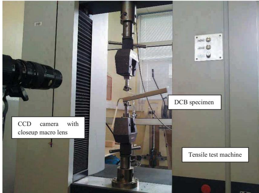
Figure 5-5: Experimental setup to calculate/measure the crack growth in DCB tests.
