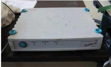
**Spider 8 data acquisition system (8 channel):**
