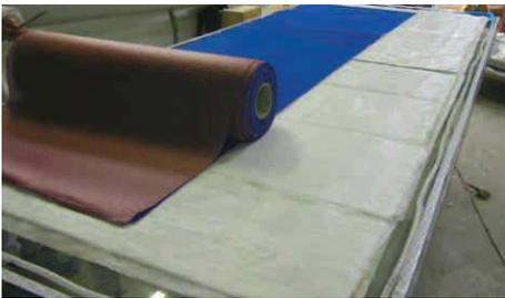
(c) Laying up of a breather cloth to drain the excess resin
