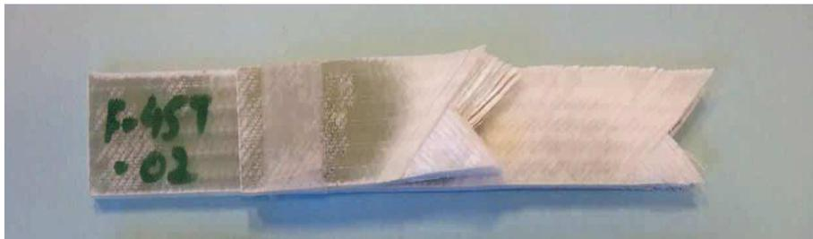
Figure 6-20: Failed 45° Biaxial specimen showing mostly delamination with some fiber sellout and breakage mode failure.
