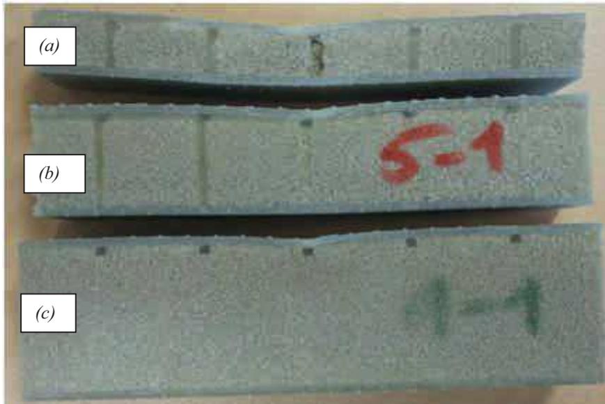
Figure 3-13: Sandwich specimens used for the characterization of the foam core (a) 10mm, (b) 20mm and (c) 30mm foam cores.
