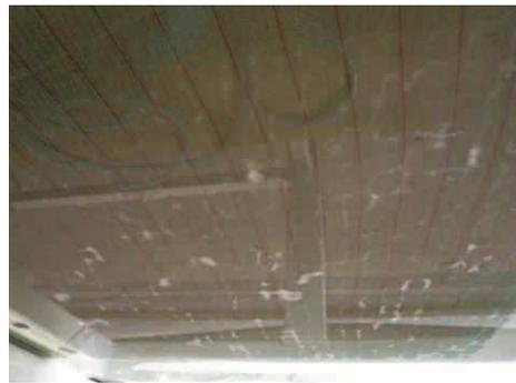
(d) Completion of infusion process as viewed from the bottom of the glass mold
