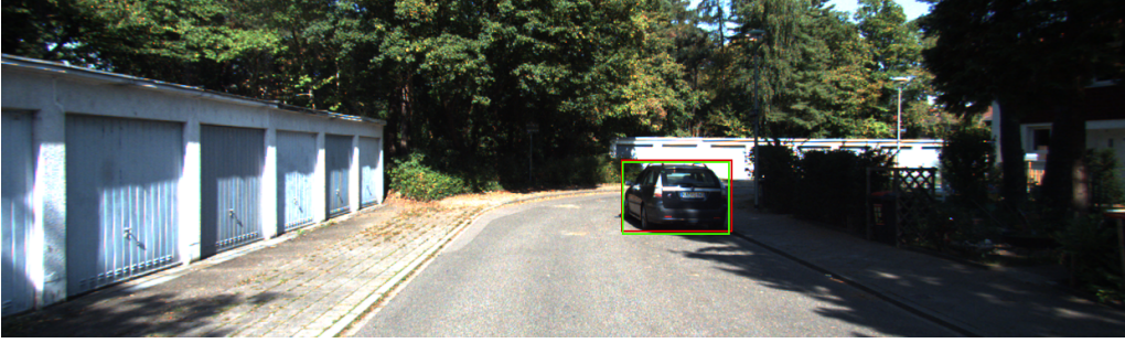
Figure 8.6: 2D detection on an optical image from the KITTI dataset using the YOLO9000 method trained on the COCO dataset (Lin et al., 2014). We can see how accurate the prediction is (in red) compared to the groundtruth (green).
