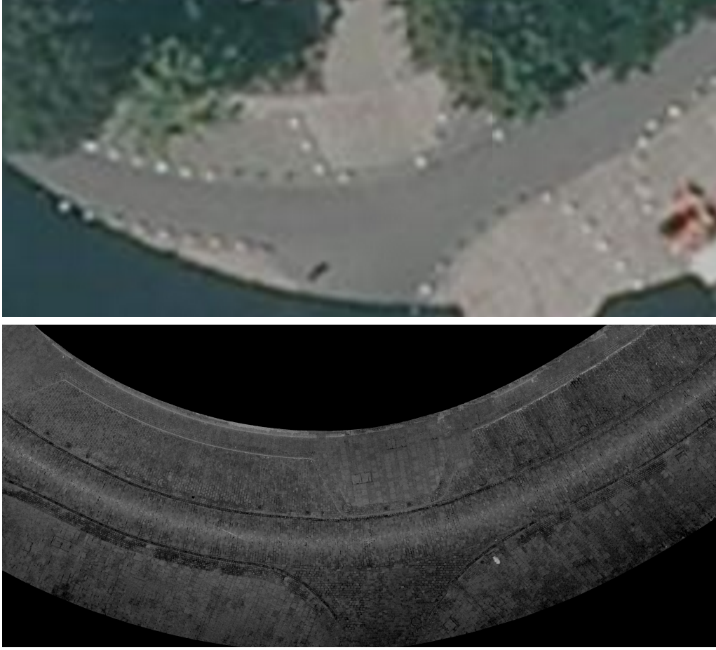
Figure 1.9: Comparison between aerial orthophotography with a standard resolution ( 10\text{cm}^2 per pixel) (top) and MLS orthoimage using our model at 1\text{cm}^2 per pixel (bottom). Traditional orthophotography provides limited resolution and suffers from occlusions brought by the coverage of trees and other structures whereas our model provides unobstructed, high resolution orthoimages. The aerial image comes from Geoportal.
