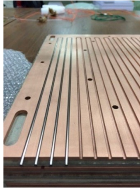
Figure 2.6: Machined copper plate.
