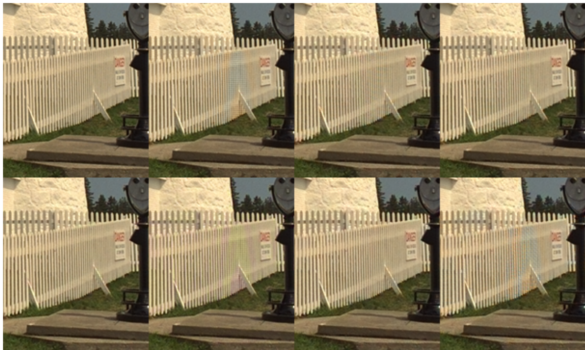
Figure 7-2: Lighthouse Image crop. Demosaiced using Neural Network method. (Top Row: Left to Right) Original, Bayer, Fuji, CNRS. (Bottom Row: Left to Right) 4x4 # 2, RGBW, Kodak 2.0, Sony RGBW.
