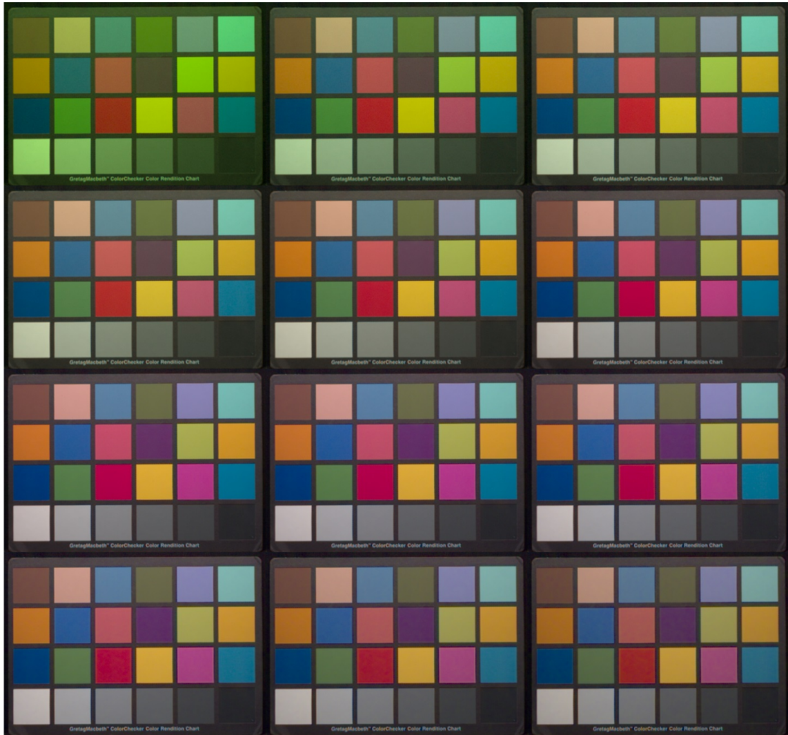
Figure 6-6: Effect of \lambda_\sigma on demosaicing for the Macbeth chart in Finlayson database for Bayer SFA. Left to Right, then Top to Bottom \lambda_\sigma goes [0.25, 0.5, 1, 2, 3, \dots, 10]
