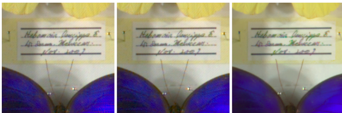
Figure 7-6: Demosaiced RAW Image from Monno5ch SFA. Left to Right: Ours NN, LMMSE, WGF. Notice Text is sharper with NN and LMMSE, there are less false colors however there are artifacts in flat regions.
