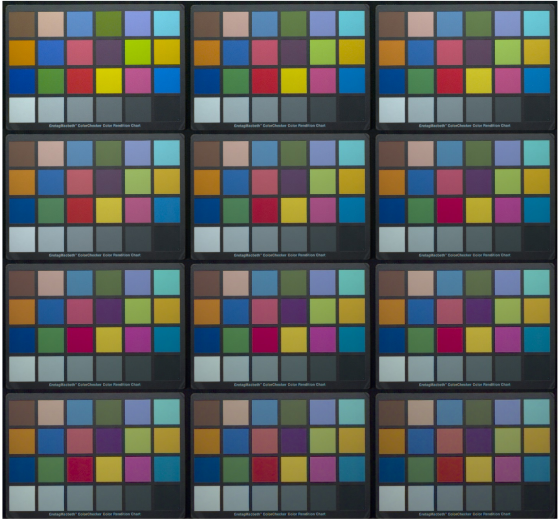
Figure 6-7: ] Effect of \lambda_\sigma on demosaicing for the Macbeth chart in Finlayson database for Bayer SFA. Output images are white-balanced by ratio of average Red, Green and Blue pixel values. Left to Right, then Top to Bottom \lambda_\sigma goes [0.25, 0.5, 1,2,3,...10]
