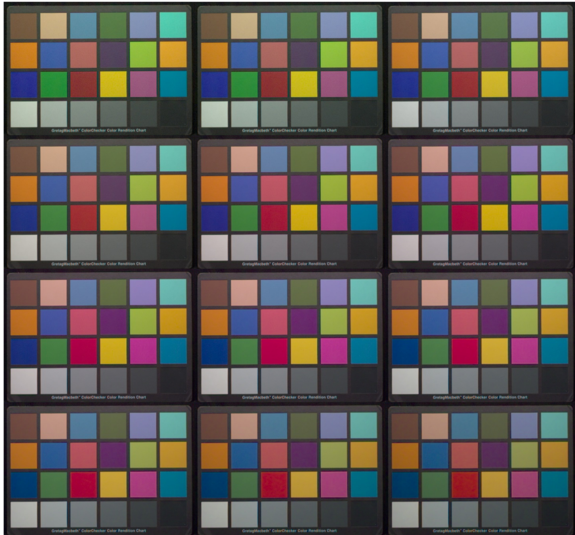
Figure 6-8: Effect of \lambda_\sigma on demosaicing for the Macbeth chart in Finlayson database for 2x2 SFA size, 4 filters. Left to Right, then Top to Bottom \lambda_\sigma goes [0.25, 0.5, 1, 2, 3, ..., 10]
