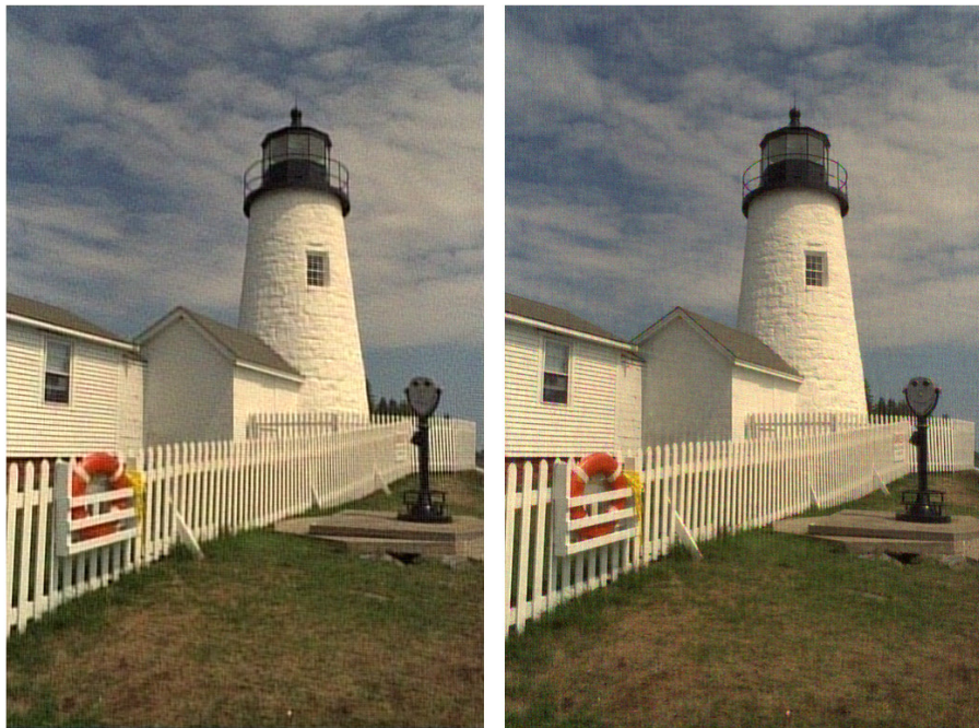
Figure 3-21: Left: Demosaiced Lighthouse image using KCS 7 . Right: Demosaiced using Group Sparse 7
