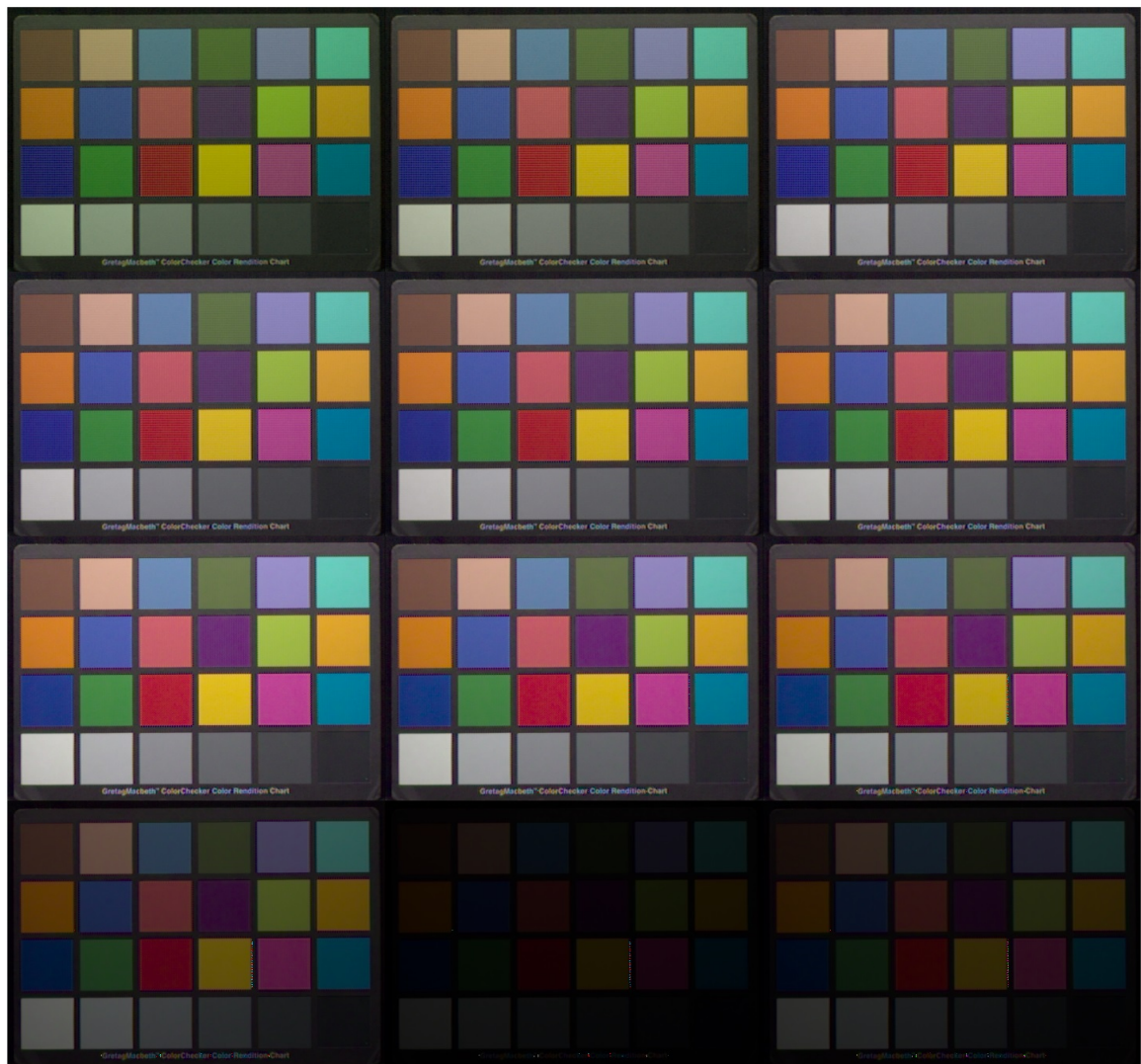
Figure 6-9: Effect of \lambda_\sigma on demosaicing for the Macbeth chart in Finlayson database for 3x3 SFA size, 9 filters. Left to Right, then Top to Bottom \lambda_\sigma goes [0.25, 0.5, 1,2,3,...10]
