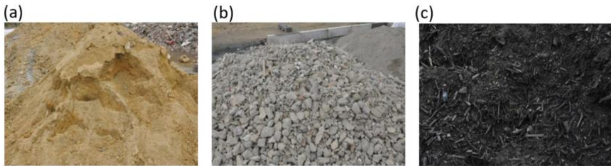
Figure 2: (a) Excavated deep horizons of soil (EDH); (b) crushed concrete (CC, 40-80 mm); (c) green waste compost (GWC).
