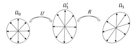
Figure 2.2: Local decomposition of the deformation tensor into stretch and rotation.
