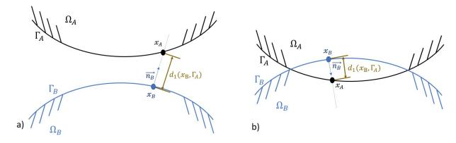
Figure 2.13: a) Body  $\mathcal{A}$  and body  $\mathcal{B}$  are close but not in contact. The  $d_1(x_B, \mathcal{A})$  measure define the gap between the bodies at point  $x_B$ . b) Body  $\mathcal{B}$  have penetrated the body  $\mathcal{A}$ . The  $d_1(x_B, \mathcal{A})$  measure gives the penetration at point  $x_B$ .
