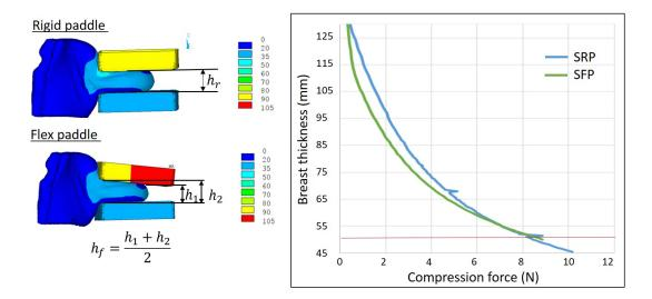
Figure 5.2: Breast flattening curve as function of the applied force for a Neo-Hookean strain energy function. SRP - standard rigid paddle, SFP -standard flex paddle
