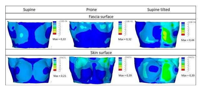
Figure 5.6: Strain distribution when using a Gent material model.
