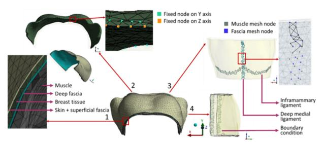
Figure 3.13: Components of the finite element mesh.
