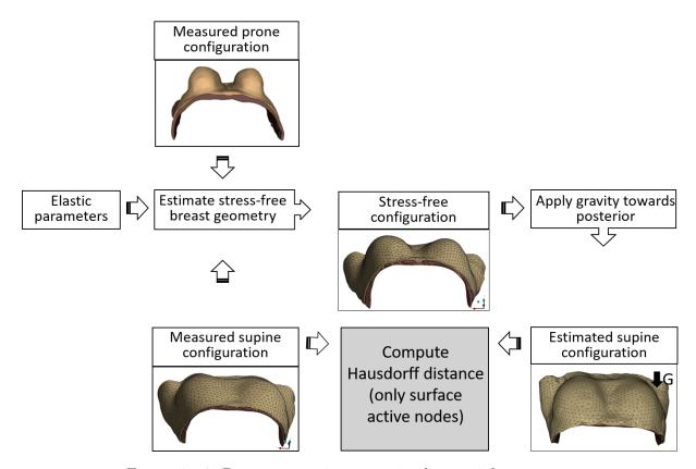
Figure 3.14: Process to estimate optimal material parameters
