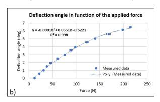
Figure 5.1: a) Experiment set-up, b) Deflection angle as function of the applied force
