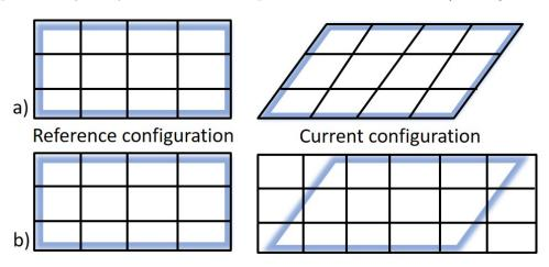
Figure 2.5: a) Lagrangian mesh formulation. b) Euler mesh formulation
