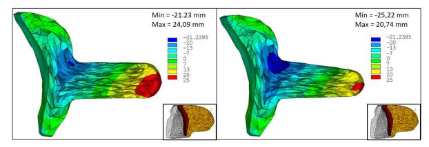
Figure 5.11: Node displacements on the direction parallel to the paddle (Oy axis). Left hand side - rigid paddle, right hand side flex paddle.
