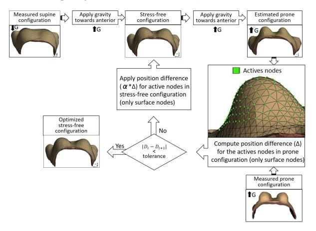
Figure 3.10: Fixed point type iterative algorithm for stress-free geometry approximation.  $D_i$  - mean node to node distance over the active nodes at iteration i, G - gravity force
