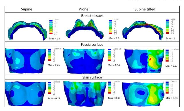
Figure 5.5: Strain distribution when using a Neo-Hookean material model.
