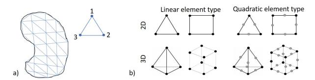
Figure 2.7: a) Discretization of a 2D domain with triangular finite element: Lagrangian mesh. b) Different types of finite elements
