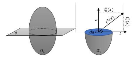
Figure 2.3: True stress vector  $t^n(x)$  at point x on the fictitious surface created by the cutting plane  $\beta$  of normal  $\overrightarrow{n}$  passing through the point x.
