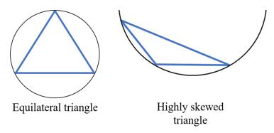
Figure 2.10: Example of triangles with different skewness with the corresponding circum radius.
