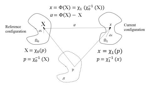
Figure 2.1: The position of a particle in the reference and current body configurations.
