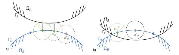
Figure 2.12: Contact status update using a pinball of radius r. Green nodes - updated nodes to closed contact status; gray nodes - updated nodes to open contact status; blue nodes - nodes which contact status need to be updated
