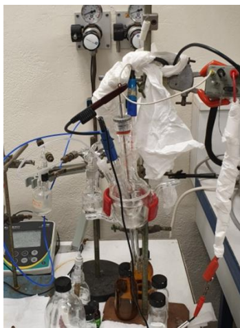
Figure 1.26 Electrochemistry setup available in Laboratoire de Chimie Physique, LCP, Paris-Sud University. The setup exhibits the electrochemical cell as well as the electrodes that were used during the electrochemistry experiments
