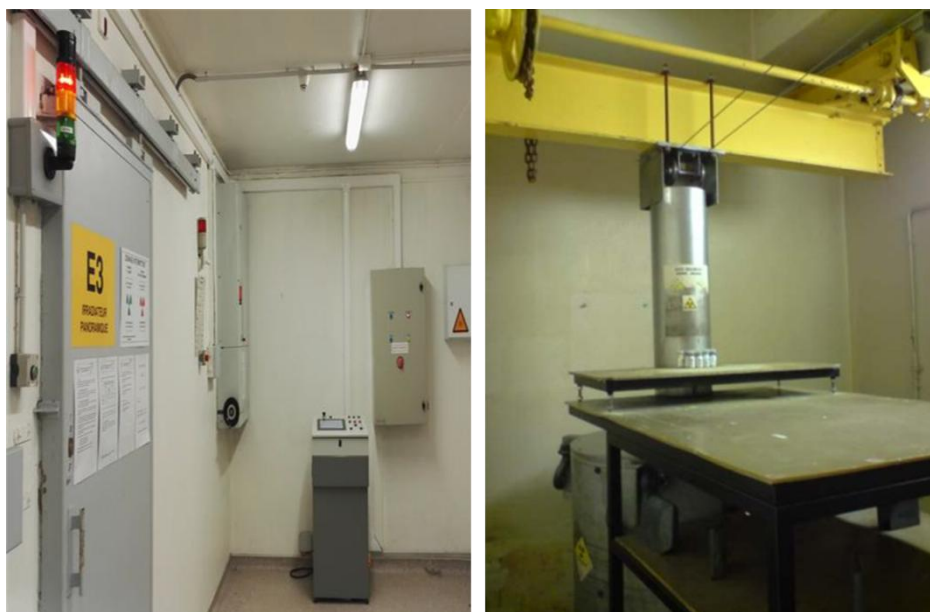
Figure 1.8 Photographs of ^{60}\text{Co} gamma source installation (LCP, Paris-Sud University). Control panel (left) and irradiation plate (right)
