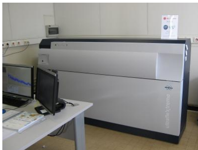
Figure 1.18 MALDI TOF TOF UltrafleXtreme, Bruker daltonic (Institut de Chimie des Substances Naturelles, CNRS, in Gif-Sur-Yvette)
