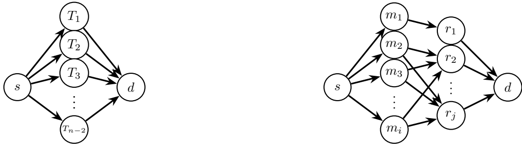
Figure 8.4: Example of simple (left) and single-stage (right) MapReduce workflows with i map tasks and j reduce tasks.
