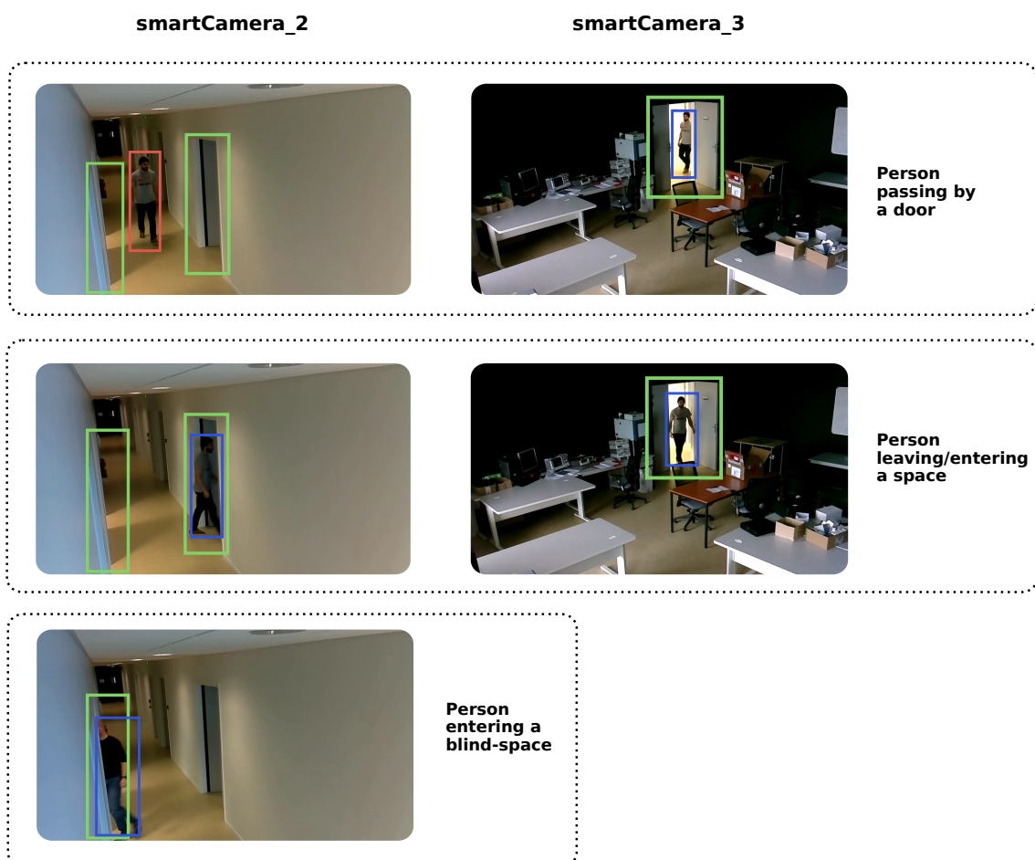
Figure 5.10 – Different scenarios of a person detected around a door. The green boxes represent Regions Of Interests (ROIs), while the blue and red boxes represent, respectively, detections made around and not around a ROI. In the first case, the person is just passing by the door (based on smartCamera_3 , because it is not being detected around the door in the smartCamera_2 ). In the second case, the detected person is leaving the space_1 (the space hosting smartCamera_2 ) and at the same time entering the space_3 . In the final case, the person is entering the space_6 , which does not have any cameras ( blind-space ) (see Fig. 5.1).
