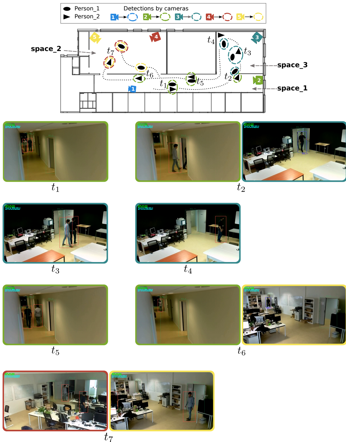
Figure 6.5 – Extract of video set 3, where two people are walking around three spaces, while being detected by a SCN. Seven timestamps of interest are being shown. The images information shown in the top-left corner is not relevant.
