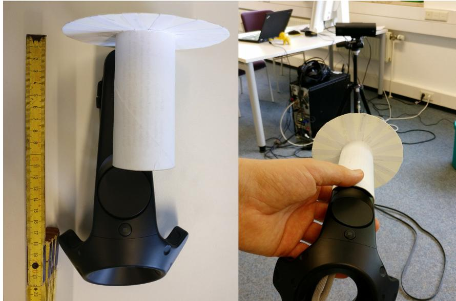
**Figure 3.9** Vive controller with mounted disc target.
