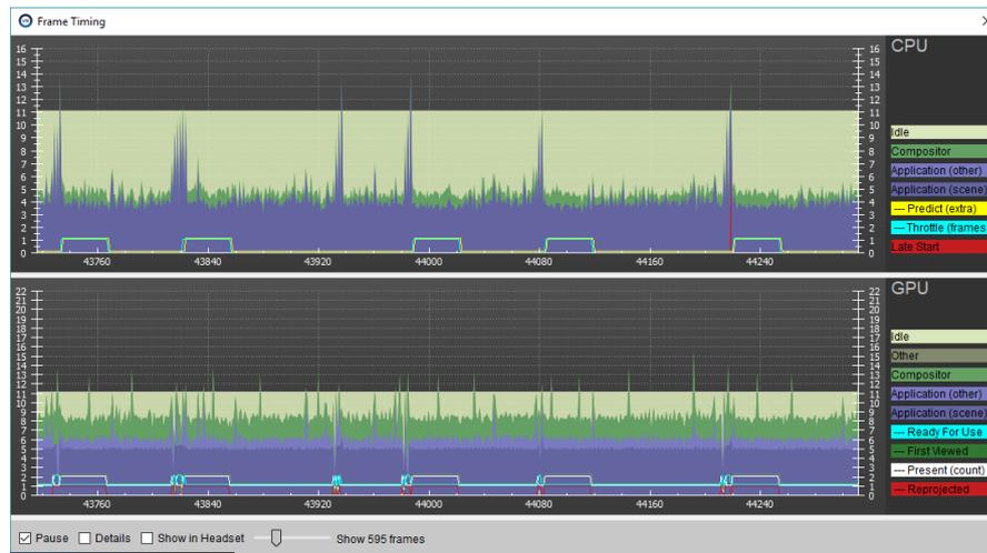
**Figure 3.7** The rendering times for a Kinect 2 point cloud using the native program library concept of Unity are on average less than 11ms.
