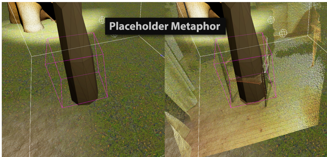
Figure 3.19 Visualization of the Placeholder Metaphor interacting with the detected obstacles. The point cloud is not visible in normal use.
