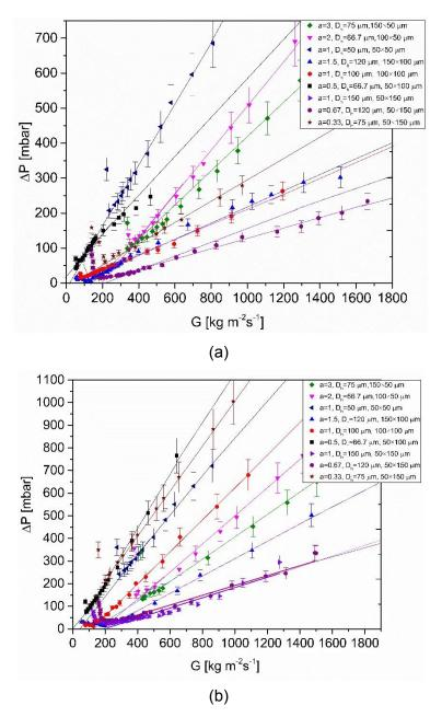
**Figure 4. 4** Pressure drop averaged over time as a function of mass flux at the constant heat fluxes of (a)  $q = 151 \text{ kW m}^{-2}$  and (b)  $185 \text{ kW m}^{-2}$  for both two-phase and single-phase flow conditions for all nine microchannel heats sinks.
