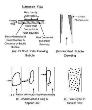
**Figure 2. 21** Dryout incipience caused by (a) the formation of a hotspot under a growing bubble, (b) near wall bubble crowding that reduces liquid film, (c) dryout under a slug and (d) liquid film dryout during annular flow at the outlet of the channel.
