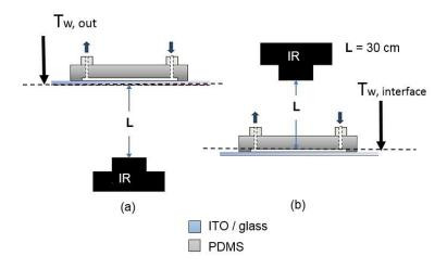
**Figure 3. 34** Two different types of temperature measurements using infrared thermography technique used in this study, where the camera examines the wall temperature (a) from ITO/glass side (channel base) and (b) from PDMS side, interfacial wall temperature measurements.
