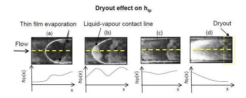
**Figure 5. 9** Sequence of optical images obtained with high-speed visualisation from the transparent ITO heater base. The two graphs below the images show the effect of partial thin film dryout on  $h_{tp}$ . The images were captured for G = 7.37 kg m<sup>-2</sup>s<sup>-1</sup> and q = 30.47 kW m<sup>-2</sup>.
