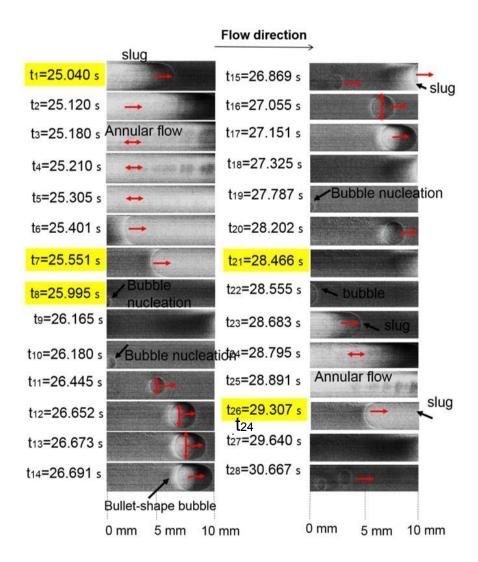
**Figure 6. 54** Flow patterns observed during flow boiling from PDMS in the test section from 0 to 10 mm. The optical images were correlated with the heat transfer coefficient presented in Figure 6.54 at the channel entrance for  $q = 43.8 \text{ kW m}^{-2}$ .
