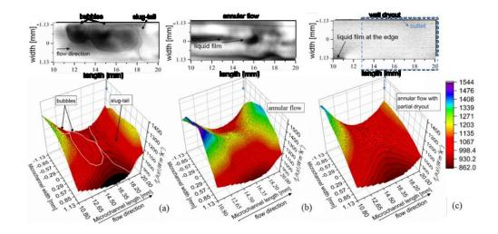
**Figure 5. 12** Local two–phase heat transfer coefficients ( $h_{tp}(x, y, t)$ ) calculated for different flow regimes with  $q = 42.28 \text{ kW m}^{-2}$  and  $G = 7.37 \text{ kg m}^{-2} \text{s}^{-1}$ . The three snapshots were captured from positions an axial distance of 10 to 20 mm from the inlet, where  $h_{tp}(x, y, t)$  was
