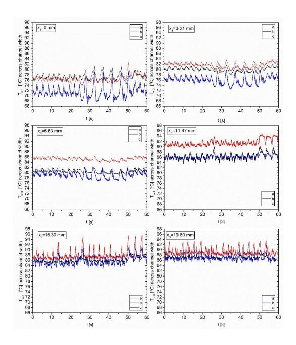
**Figure 6. 50** Wall temperature fluctuations measured at three positions (channel upper corner: centre of the channel width and other channel corner) across the channel width for G = 14.38 kg  $m^{-2}s^{-1}$  and q = 47.78 kW  $m^{-2}$ .
