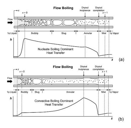
**Figure 2. 6** Schematics of flow regimes, with local variation of heat transfer coefficient in mini/microchannels with uniform circumferential heat flux for (a) nucleate boiling dominant heat transfer and (b) convective boiling dominant heat transfer [51].
