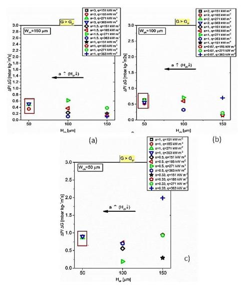
**Figure 4. 8** Channel height as a function of  $\Delta P/\Delta G$  for the three constant widths of (a)  $W_{ch}$  = 150  $\mu$ m (b) 100  $\mu$ m, (c) 50  $\mu$ m. for the case of  $G < G_{cr}$ , where  $G_{cr}$  is the value where the  $\Delta P/\Delta G$  slope changes.
