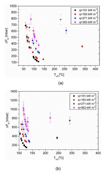
Figure 4. 20 Time averaged two-phase pressure drop as a function of wall temperature at T5 for the heat fluxes of 151 kW m<sup>-2</sup>, 183 kW m<sup>-2</sup>, 271 kW m<sup>-2</sup> and 363 kW m<sup>-2</sup> for  $\alpha = 2$  and  $D_h = 66.7 \mu m$  for (a)  $T_{inlet} = 25$  °C and (b)  $T_{inlet} = 81$ °C.
