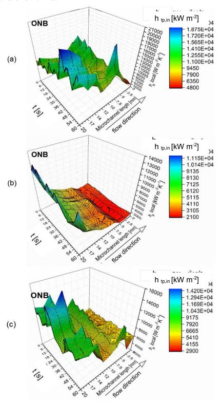
**Figure 6. 4** 3D plots of the local  $h_{tp,in}$  spatially averaged across the microchannel width at 9 equally spaced locations, as a function of time and channel length at ONB for (a) 36.87 kg m<sup>-2</sup> s<sup>-1</sup> and q = 35 kW m<sup>-2</sup>(b) 73.74 kg m<sup>-2</sup> s<sup>-1</sup> and q = 36.87 kW m<sup>-2</sup> and (c) G = 101.2 kg m<sup>-2</sup> s<sup>-1</sup> and q = 45.26 kW m<sup>-2</sup>.
