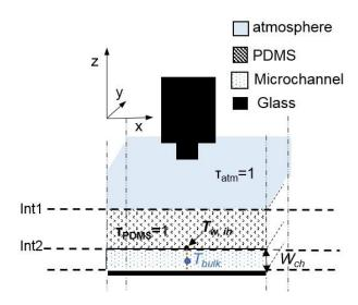
**Figure 3. 30** Schematic of the interfacial wall temperature measurement obtained from the PDMS side using an infrared camera.
