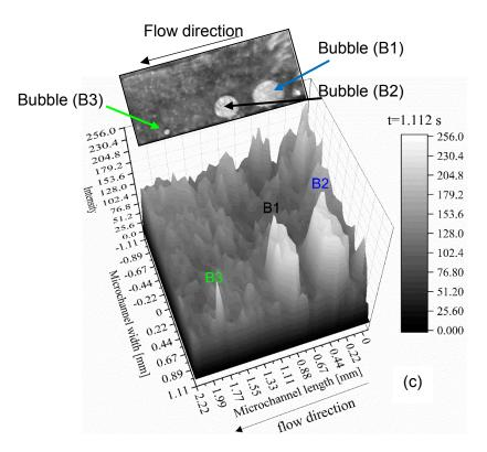
(c) 3D plot of pixel intensity as a function of channel width and length for the inlet during bubble growth near the sidewall corner. Flow direction is from the right to the left.
