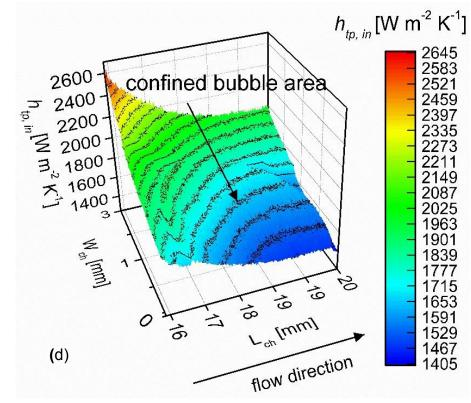
**Figure 6. 41** (a), (b),(c), (d) show patial variation of the interfacial two-phase heat transfer coefficients  $h_{tp}$ , of the microchannels during single bubble growth.
