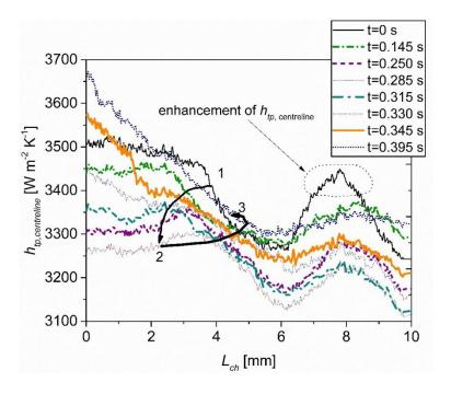
**Figure 6. 60** h(x) along the centreline for the inlet and middle of the microchannel as a function of time for a periodic instability for G = 36.87 kg m<sup>-2</sup>s<sup>-1</sup>and q = 119.9 kW m<sup>-2</sup>.
