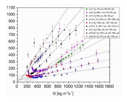
**Figure 4. 5** Pressure drop averaged over time as a function of mass flux at the constant heat flux of 271 kW m<sup>-2</sup> for both two-phase and single-phase flow conditions for all nine microchannel heat sink designs with characteristics presented in Table 3.1 of chapter 3. The inlet temperature is  $25 \, ^{\circ}\text{C} \pm 1 \, ^{\circ}\text{C}$ .
