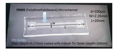
Figure 3. 19 PDMS microchannel, bonded to ITO coated glass.
