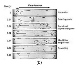
**Figure 2. 14** (a) Flow pattern map by Ong and Thome [46] and (b) flow patterns recorded during FC-72 boiling in a high aspect ratio rectangular channel with  $D_h = 1454 \mu m$ ,  $G = 22.4 kg m^{-2} s^{-1}$  and  $q = 8.13 kW m^{-2}$  from the study of Wang et al. [74].
