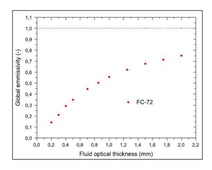
Figure A. 2 Emissivity of FC-72 as a function of the thickness from Brutin et al. [121]
