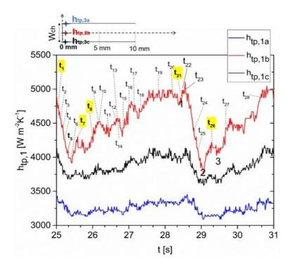
**Figure 6. 53** Local two-phase heat transfer coefficients were obtained at the channel entrance. The locations where  $h_{tp}$ , 1a,  $h_{tp}$ , 1b, and  $h_{tp}$ , 1c were calculated, are presented in the schematic on the top of the graph.
