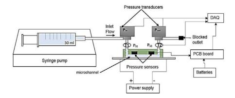
**Figure 3. 37** *Schematic drawing of the calibration setup.*
