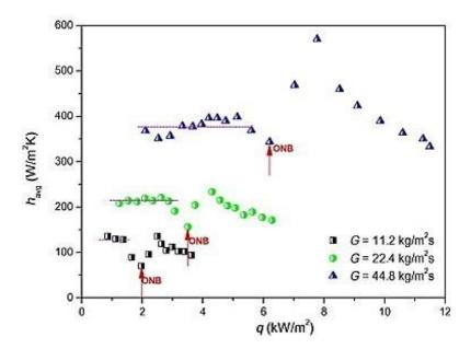
**Figure 2. 18** Heat transfer coefficient, time averaged as a function of heat flux for three mass fluxes of 11.22, 22.4 and 44.8 kg m<sup>-2</sup>s<sup>-1</sup> tested with FC-72 in a high aspect ratio microchannel with round corners and  $D_h = 550 \mu m$  [33].
