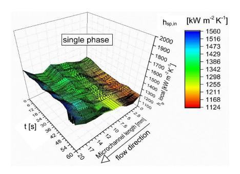
**Figure 6. 3** 3D plot of the local single-phase heat transfer coefficient ( $h_{sp.}$ ) spatially averaged across the channel with, as a function of time and channel length for G = 73.74 kg m<sup>-2</sup>s<sup>-1</sup> and q = 27.66 kW m<sup>-2</sup>.
