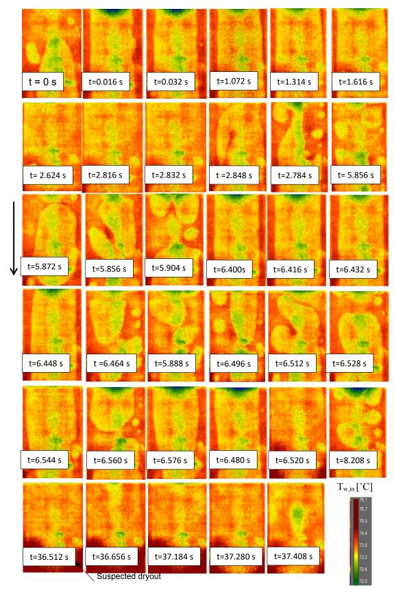
**Figure 6. 14** Image sequence that shows local flow patterns and temperature variation at the outlet, for  $G = 36.8 \text{ kg m}^{-2}\text{s}^{-1}$  and  $q = 57.13 \text{ kW m}^{-2}$ . The IR images were recorded at 200 Hz.
