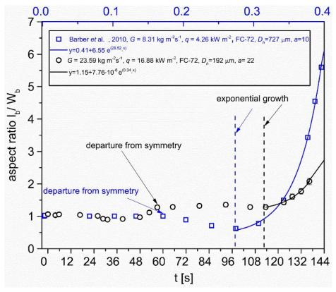
**Figure 6. 44** Aspect ratio of bubble as a function of time obtained with synchronised IR camera and high speed camera at 200 Hz and for  $G = 23.59 \text{ kg m}^2 \text{ s}^{-1}$  and  $q = 16.88 \text{ kW m}^{-2}$  using FC72 in the high aspect ratio (a = 22) PDMS microchannel (black colour). The results were compared from the results from the study of Barber et al.[134] for a microchannel with curved corners and higher hydraulic diameter.
