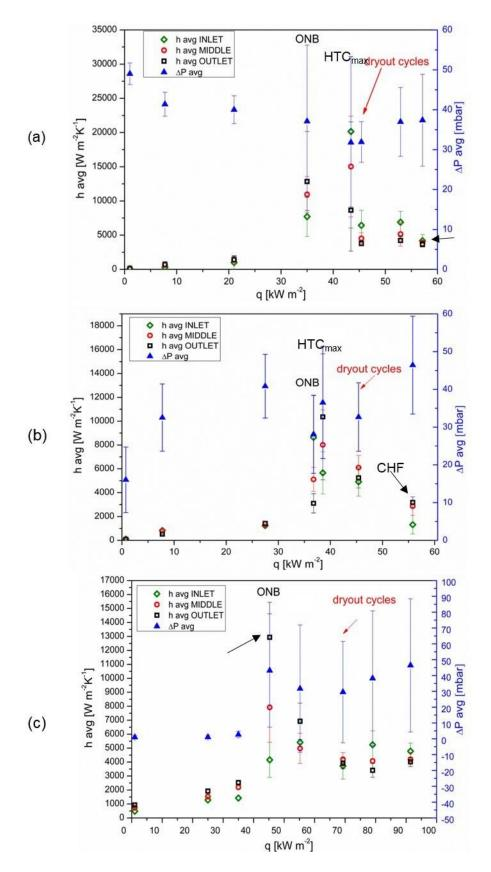
Figure 6. 2 Time averaged interfacial heat transfer coefficients for inlet, middle and outlet with increasing heat flux and time averaged pressure drop for the mass fluxes of
