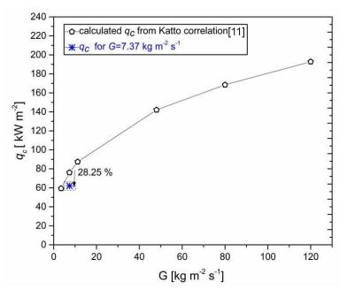
**Figure 5. 8** Comparison of the critical heat flux as a function of mass flux, from this study and previous experimental studies as well as the calculated critical heat flux obtained from Katto [11] correlation.
