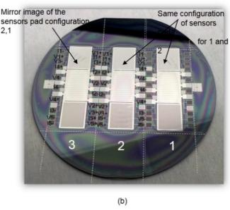
Figure 3. 6 Silicon wafer with microchannel heat sinks devices, from the front side (a) and the backside (b). The numbers 1, 2, 3 are used to distinguish the test devices with different microchannel widths of 150 μm (2), 100 μm (3) and 50 μm (1).
