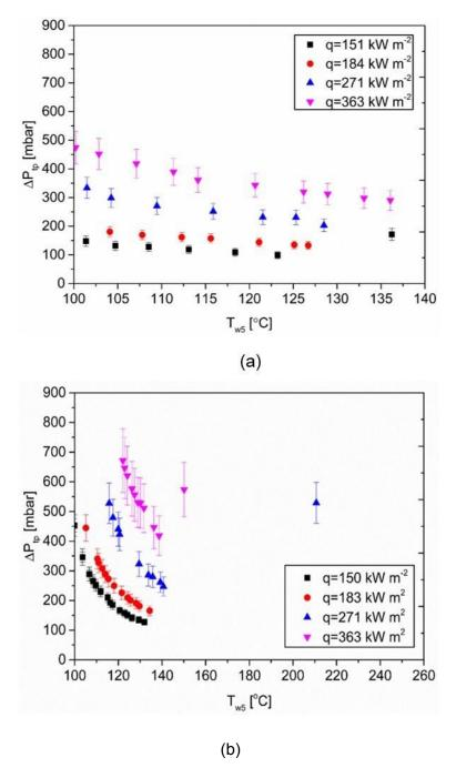
**Figure 4. 21** Averaged over time two-phase pressure drop as a function of wall temperature at T5 for the heat fluxes of 151 kW m<sup>-2</sup>, 183 kW m<sup>-2</sup>, 271 kW m<sup>-2</sup> and 363 kW m<sup>-2</sup> near the exit (location of T5) of (a) a = 3,  $D_h = 75 \mu m$  and (b) a = 2,  $D_h = 66.7 \mu m$  at  $T_{inlet} = 25$  °C.
