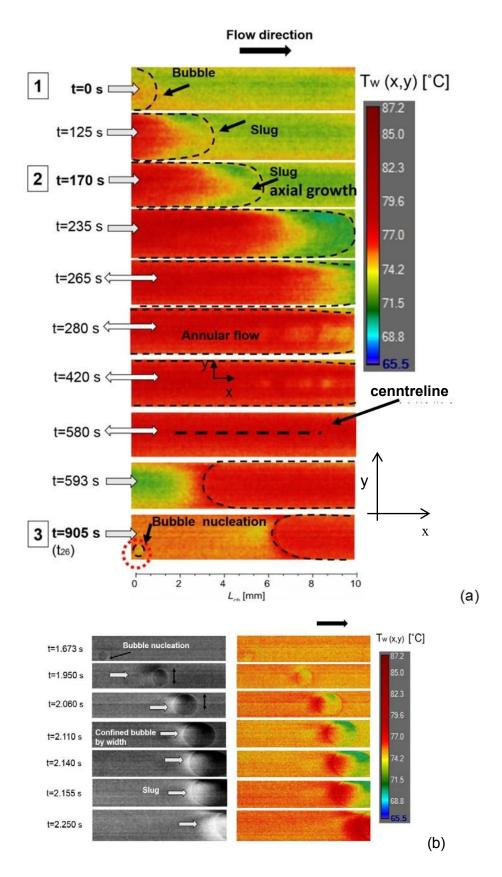
Figure 6. 56 Two-dimensional wall temperature measured with the IR camera from the ITO/glass base of the microchannel and reveals the occurrence of (a) high amplitude and (b)
