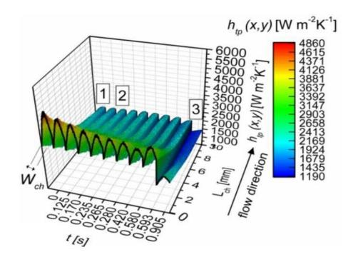
**Figure 6. 57** 3D plot of the two-dimensional two-phase flow boiling heat transfer distribution across microchannel for  $G = 14.78 \text{ kg m}^2\text{s}^{-1}$  and  $q = 43.80 \text{ kW m}^{-2}$  from 0 to 10 mm. The numbers 1, 2, 3 are related to the fluctuation cycle shown in Figure 6.64a.
