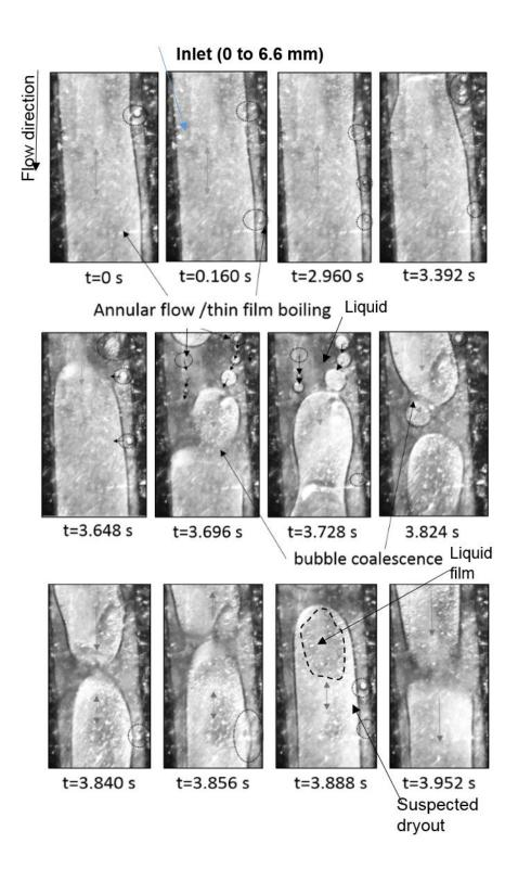
**Figure 6. 35** High-speed image sequences obtained from the transparent ITO heater base with for  $q = 38.54 \text{ kW m}^{-2}$  where the maximum heat transfer coefficient occurs at  $G = 73.74 \text{ kg m}^{-2}$  S-1.
