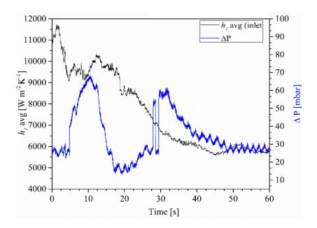
**Figure 6. 33** Local heat transfer coefficient measured at x=0 mm with simultaneous pressure drop for G=73.74 kg m<sup>-2</sup> s<sup>-1</sup> and q=38.52 kW m<sup>-2</sup>.
