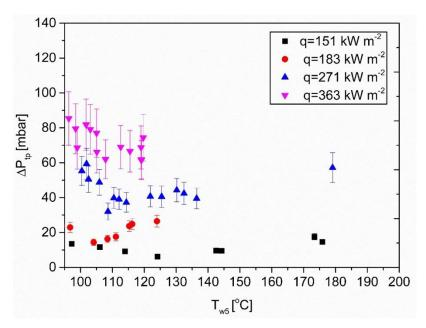
**Figure 4. 22.** Averaged over time two-phase pressure drop as a function of wall temperature at position 5 for the heat fluxes of 151 kW m<sup>-2</sup>, 183 kW m<sup>-2</sup>, 271 kW m<sup>-2</sup> and 363 kW m<sup>-2</sup> near the exit of a = 1.5,  $D_h = 120 \mu m$  microchannels at  $T_{inlet} = 25$  °C.
