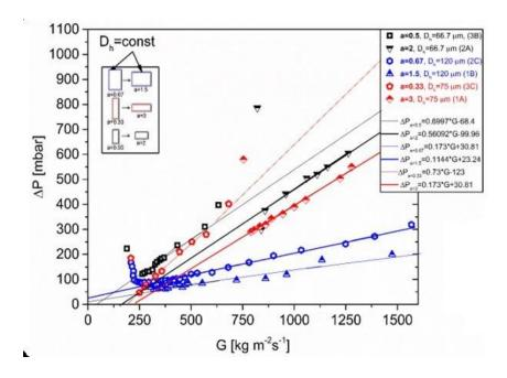
**Figure 4. 14** Pressure drop for single and two-phase flow conditions for a constant hydraulic diameter and changing aspect ratio as a function of mass flux for the heat flux of q = 363 kW  $m^{-2}$ , the inlet temperature of  $T_{inlet} = 25 \text{ °C}$ .
