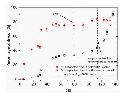
**Figure 6. 46** Dryout area percentage measured below the bubble and dryout are percentage of the channel as a function of time. The dryout area is confirmed by IR and flow visualisation images and was measure with Image J software.
