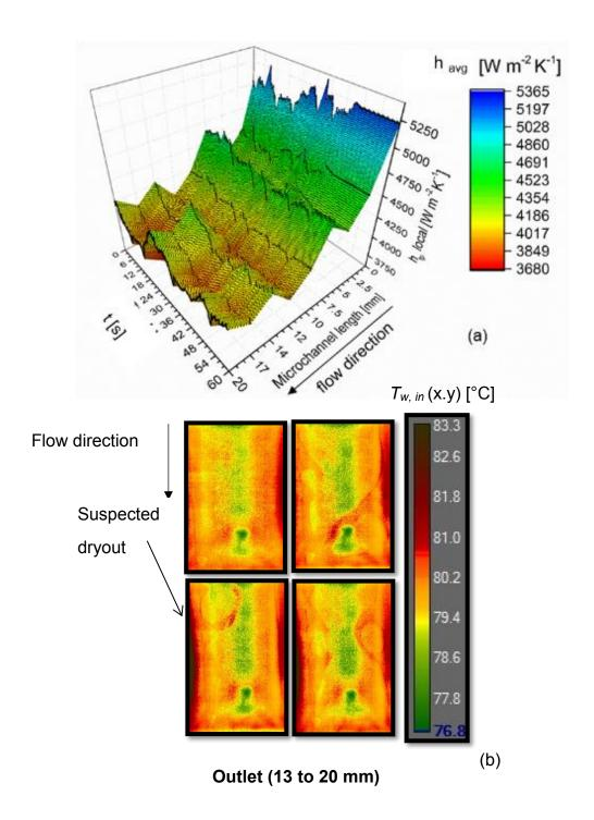
**Figure 6. 12** (a) 3D plot of local interfacial  $h_{tp,in}$  spatially averaged across the microchannel width at 9 equally spaced positions, as a function of time and channel length at q = 91.46 kW  $m^{-2}$  and  $G = 101.62 \text{ kg m}^{-2} \text{ s}^{-1}$  and (b) sequence of IR images that show the alternation between liquid flow with bubbles in the stream-wise direction and slug flow for the channel inlet from 13 to 20 mm length (outlet).
