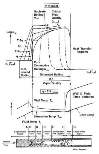
**Figure 2. 2** Illustration of forced convective boiling with qualitative temperature profile and heat transfer coefficient profile for a uniform heat flux boundary condition at a vertical tube used by Steiner and Taborek [48].
