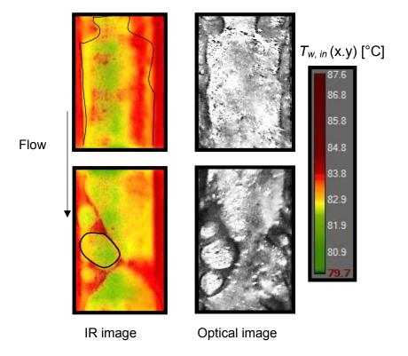
**Figure 6. 15** Correlation of simultaneous thermal images obtained from the transparent to infrared PDMS top with optical images obtained from the transparent ITO heater during slug-annular flow regime at  $G = 147.2 \text{ kg m}^{-2} \text{ s}^{-1}$  and  $q = 99.7 \text{ kW m}^{-2}$  at 200Hz.
