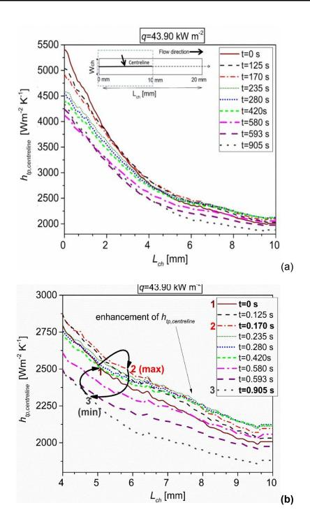
**Figure 6. 55** Local two-phase heat transfer coefficient profiles as a function of time along the channel centreline (from 0 to 10 mm) for  $G = 14.78 \text{ kg m}^{-2} \text{s}^{-1}$  and  $q = 43.80 \text{ kW m}^{-2}$  and (b) for the channel length from 4 to 10 mm. The cycle of the high amplitude fluctuation was represented with arrows related also to Figure 6.69.
