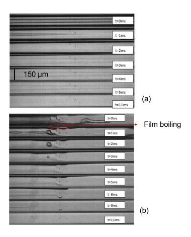
**Figure 4. 27**(a) Uniform thin film evaporation and (b) non uniform film evaporation at the inlet of the channels for G = 337.22 kg m<sup>-2</sup> s<sup>-1</sup> and q = 151 kWm<sup>-2</sup> at 1000 Hz with a = 3,  $D_h = 75 \mu m$  at location of sensor T5.
