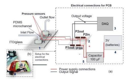
**Figure 3. 24** Analytical graph of the electrical connections of the pressure sensors with the circuit board.
