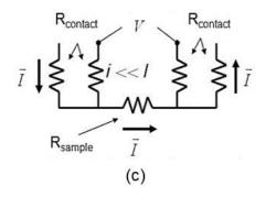
**Figure 3. 5** (a) Diagram of the temperature sensors from the backside of the microchannels, (b) position of temperature sensors from the front side of the microchannels heat sink and (c) schematic diagram of the four-point resistivity measurement by the temperature sensor.
