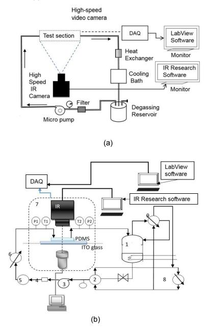
Figure 3. 35 Schematic drawing of (a) the wall temperature measurements from the ITO/glass base and (b) the flow loop used to facilitate wall temperature measurements PDMS side.
