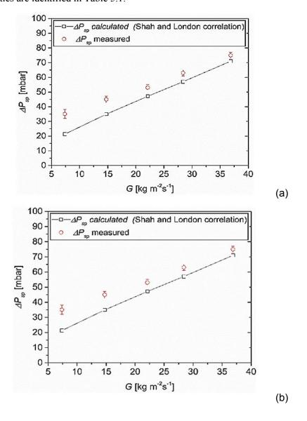
**Figure 5. 1**(a) Experimental and theoretical single-phase pressure drop in function of the mass flux. (b) Experimental and theoretical single-phase heat transfer coefficient in function of the heat flux.
