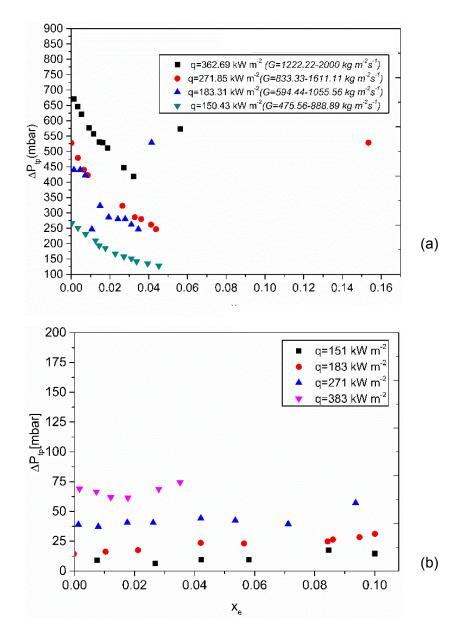
**Figure 4. 23.** Averaged over time two-phase pressure drop as a function of vapour quality at T5 for the heat fluxes of 151 kW m<sup>-2</sup>, 183 kW m<sup>-2</sup>, 271 kW m<sup>-2</sup> and 363 kW m<sup>-2</sup> near the exit of (a)  $\alpha = 3$ ,  $D_h = 75 \mu m$ ,  $T_{inlet} = 81 \, ^{\circ}\text{C}$  (b)  $\alpha = 1.5$ ,  $D_h = 120 \mu m$  microchannels at  $T_{inlet} = 25 \, ^{\circ}\text{C}$ .
