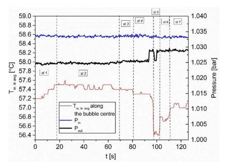
**Figure 6. 38**  $T_w$ , and pressure from the inlet  $(P_{in})$  and outlet  $(P_{out})$  of the microchannel as function of time during bubble growth shown in Figure 6.18.  $T_w$ , is spatially averaged along the line that crosses the bubble centre. The inner wall temperature measurements are obtained with the simultaneous pressure from the integrated pressure sensors inside the microchannel.
