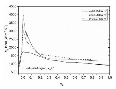
**Figure 5. 14** The relationship between local two-phase heat transfer coefficient and vapour quality for increasing heat fluxes at a constant mass flux of G = 7.37 kg m<sup>-2</sup>s<sup>-1</sup>.
