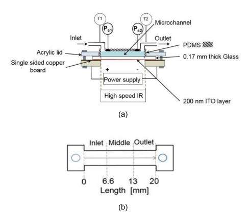
**Figure 3. 32** Schematic drawing of (a) housing with the PDMS microchannel which consists of a microchannel with integrated pressure sensors  $(P_{s1}, P_{s2})$  and its support (b) the three measurement sections along the microchannel.
