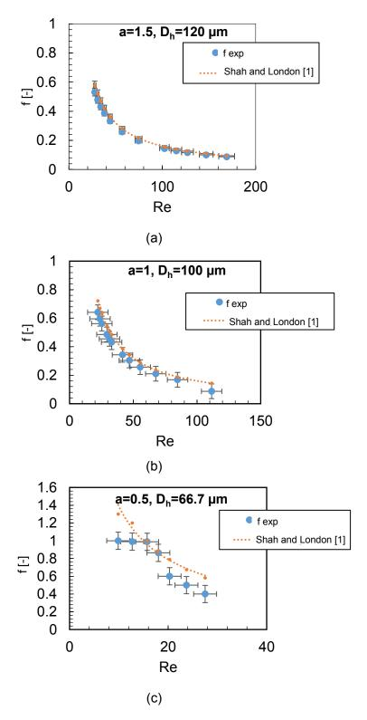
**Figure 4. 1** . Comparison of predicted friction factor with existing experimental results and existing correlation.
