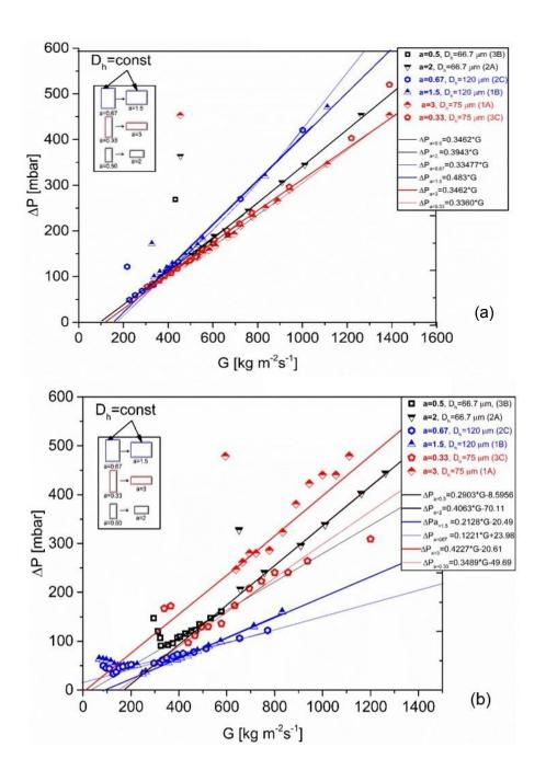
**Figure 4. 15** Pressure drop data for single and two-phase flow conditions for a constant hydraulic diameter and changing aspect ratio as a function of mass flux. For the heat fluxes of (a)  $q = 151 \text{ kW m}^{-2}$  and (b)  $q = 183 \text{ kW m}^{-2}$  at  $T_{inlet} = 81 \text{ °C}$ .
