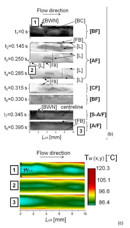
**Figure 6. 61** (a) 3D plot of high spatial and temporal resolution two-dimensional  $h_{tp}$  (x,y) as a function of time for a periodic cycle of instability for  $G = 36.87 \text{ kgm}^2\text{s}^{-1}$  and  $q = 119.9 \text{ kW m}^{-2}$  and (b) flow patterns observed with high-speed imaging (200 Hz) from t = 0 s to t = 0.395 s simultaneously with (c) the thermal images, for  $G = 36.87 \text{ kg m}^2\text{s}^{-1}$  and  $q = 119.47 \text{ kW m}^{-2}$ .
