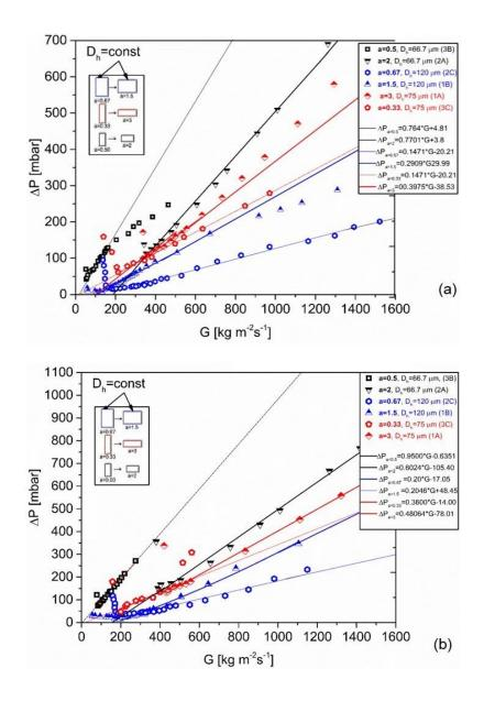
**Figure 4. 13** Pressure drop for single and two-phase flow conditions for a constant hydraulic diameter and changing aspect ratio as a function of mass flux for the heat fluxes of (a)  $q = 151 \text{ kW m}^{-2}$  and (b)  $q = 183 \text{ kW m}^{-2}$  for  $T_{in} = 25 \text{ °C}$ .
