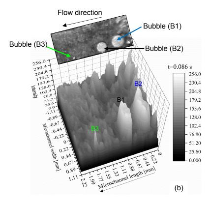
(b) 3D plot of pixel intensity as a function of channel width and length for the inlet after mergin, of the vapour bubbles near the sidewall corner. Flow direction is from the right to the left.
