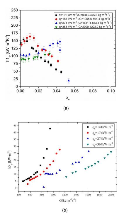
**Figure 4. 26** Local heat transfer coefficient as a function of vapour quality (a) at T1 and (b) at T5 as a function of mass flux at constant heat fluxes of 151 kW m<sup>-2</sup>K<sup>-1</sup>, 174 kW m<sup>-2</sup>K<sup>-1</sup>, 271 kW m<sup>-2</sup>K<sup>-1</sup> and 364 kW m<sup>-2</sup>K<sup>-1</sup> for  $\alpha = 3$  and  $D_h = 75$   $\mu$ m microchannels.
