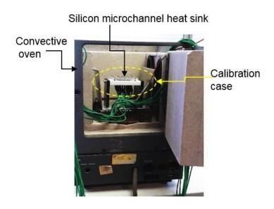
**Figure 3. 14** Convective oven used for the calibration of the thin film Ni temperature sensors integrated into the microchannels heat sink.
