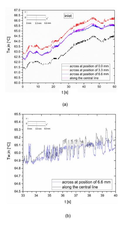
**Figure 6. 26** (a) Inner wall temperature fluctuations spatially averaged across the channel width at x=0 mm, 3.3 mm and 6.6 mm from the channel entrance and along the channel centreline at flowstream direction of the inlet for G=73.74 kg m<sup>-2</sup> s<sup>-1</sup> and q=38.54 kW m<sup>-2</sup> and (b) zoom in inner wall temperature fluctuations from 33 to 40 s.
