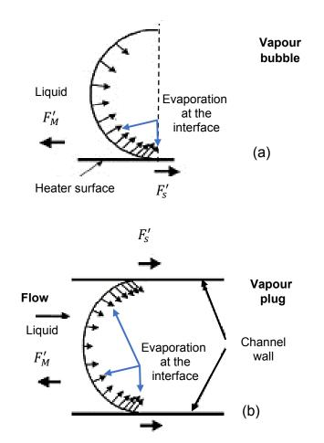
Figure 2. 7 (a) Evaporation momentum force acting on the evaporating interface of a growing bubble and (b) forces due to evaporation momentum and surface tension acting on a liquid-vapour interface of a bubble filling the microchannel cross-section [38].
