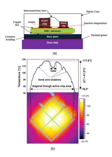
*Figure 1. 1* (a) Schematic drawing of typical IGMT module produced by Mitsubishi Electronic Corporation in 2015 and (b) temperature distribution across the diagonal of an IGMT chip.
