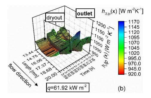
Figure 5. 6 Local two-phase heat transfer coefficient  $h_{tp}(x, t)$  along the microchannel centreline in the stream-wise direction with a time interval of 0.015 s for the outlet of the microchannel for (a)  $q = 30.97 \text{ kW m}^{-2}$  and  $q = 61.95 \text{ kW m}^{-2}$  (b).
