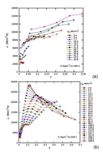
**Figure 2. 4** (a) Local flow boiling heat transfer coefficient versus local vapour quality for increasing base heat fluxes for G = 280.5 kg m<sup>-2</sup>s<sup>-1</sup> and (b) local flow boiling heat transfer coefficient versus local vapour quality for increasing base heat fluxes for G = 549.7 kg m<sup>-2</sup>s<sup>-1</sup>[50].
