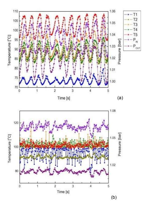
**Figure 2. 17** Simultaneous temperature and pressure fluctuations for two types of instabilities HALF (high amplitude low frequency) and LAHF (low amplitude –high frequency) for the same mass flux of 208 kg m<sup>-2</sup>s<sup>-1</sup>, at the inlet temperature of 71 °C for the 40 parallel rectangular silicon microchannels of  $D_h$ =192  $\mu$ m from the study of Bogojevic et al. [34] for (a)  $q = 210 \text{ kW m}^{-2}$  and (b)  $q = 376 \text{ kW m}^{-2}$ .
