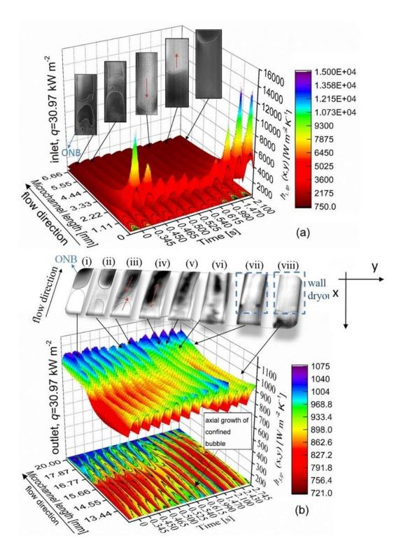
**Figure 5. 10** 2D maps of the local two-phase heat transfer coefficient  $h_{tp}(x, y, t)$  with time for, the inlet (a) and the outlet (b) of the microchannel heat sink for  $q = 30.97 \text{ kW m}^{-2}$ .
