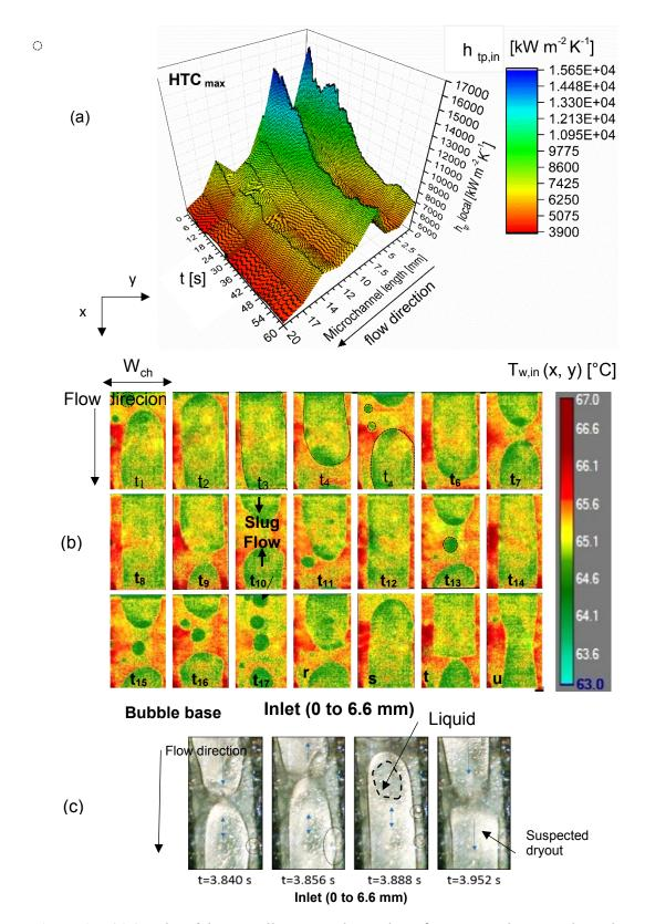
**Figure 6.** 7 (a) 3D plot of the spatially averaged two-phase  $h_{tp,in}$  across the microchannel width at 9 equally spaced positions along the microchannel domain, as a function of time and length at increased heat flux after ONB at the heat flux of q = 55.23 kW m<sup>-2</sup> and G = 110.62 kg m<sup>-2</sup> s<sup>-1</sup>.
