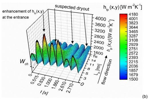
**Figure 6. 58** High spatial and temporal resolution 3D plots of the two-dimensional two-phase heat transfer coefficient h(x, y), (a) across the whole domain of the microchannel and (b) for the length of 0 to 16 mm for G = 14.78 kg m<sup>-2</sup>s<sup>-1</sup> and g = 47.78 kW m<sup>-2</sup>.
