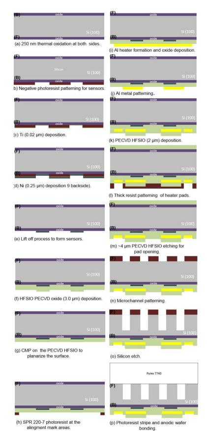
Figure 3. 4 Microfabrication steps of silicon microchannels heat sink.
