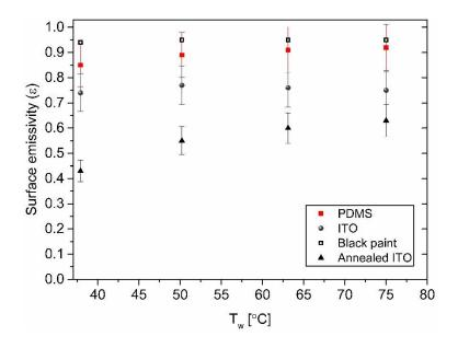
Figure 3. 29 Averaged surface emissivity of non-annealed ITO glass.
