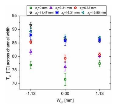
**Figure 6. 51** Averaged over time (with deviation) local temperatures at the three positions (a, b, c) across the channel for each positions from 1 to 6 along the channel length. Bubble nucleation started at x = 16.31mm, at the channel corner (a).
