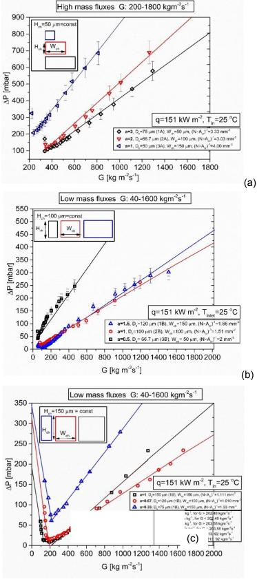
**Figure 4. 6** Pressure drop averaged over time as a function of mass flux at the constant heat flux of  $q = 151 \text{ kW m}^2$  for (a) constant height of 50  $\mu$ m and increasing widths of 50, 100 and
