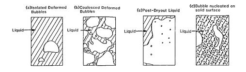
Figure 2. 22 Boiling phenomena in confined spaces [110].
