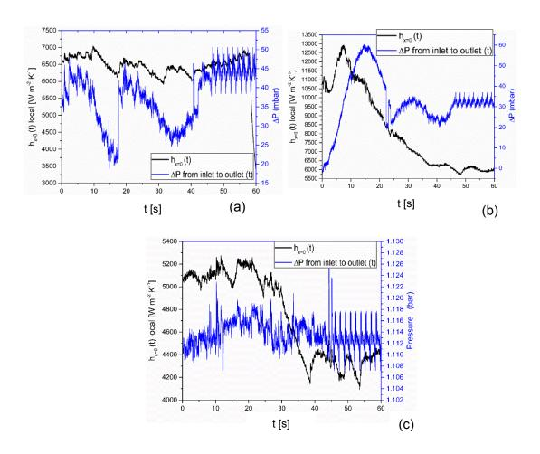
**Figure 6. 31** Local heat transfer coefficient fluctuations obtained at entrance (x = 0 mm and y = 0 mm) of the microchannel and simultaneous pressure drop fluctuations for (a) G = 36.87 kg m<sup>-2</sup> s<sup>-1</sup> and q = 45.50 kW m<sup>-2</sup>, (b) G = 36.87 kg m<sup>-2</sup> s<sup>-1</sup> and (c) q = 52.92 kW m<sup>-2</sup>.
