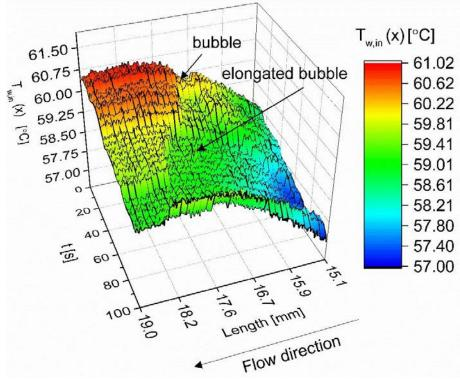
**Figure 6. 39** 3D plot of local inner wall temperature profile along microchannel during bubble growth vs time for  $G = 23.59 \text{ kg m}^{-2} \text{ s}^{-1}$  and  $q = 16.88 \text{ kW m}^{-2}$  using FC-72 in a PDMS
