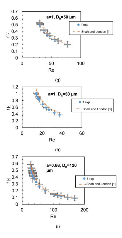
**Figure 4. 3** Comparison of predicted friction factor with existing experimental results and existing correlation.
