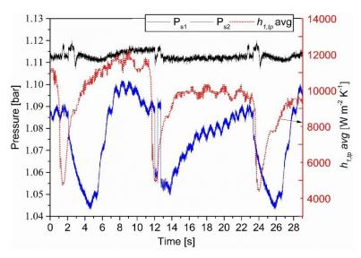
**Figure 5. 16** Two-phase pressure fluctuations at the inlet  $(Ps_1)$  and outlet  $(Ps_2)$  of the microchannel and the averaged locally two-phase hat transfer coefficient calculated at the channel inlet section for 29 s time interval at  $q = 30.97 \text{ kW m}^{-2}$  and  $G = 7.37 \text{ kg m}^{-2} \text{ s}^{-1}$ .
