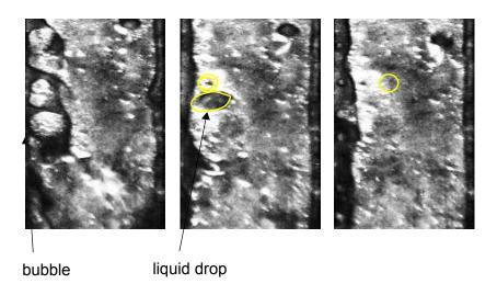
Figure 6. 17 Bubble burst mechanism for  $G = 147.2 \text{ kg m}^{-2} \text{ s}^{-1}$  and  $g = 99.7 \text{ kW m}^{-2}$ .
