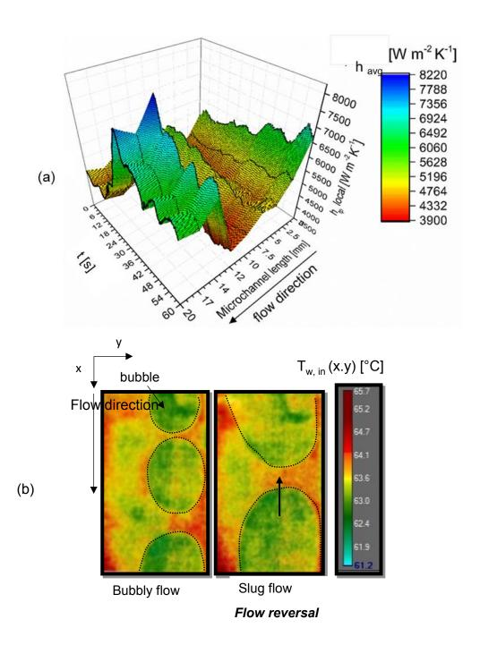
**Figure 6. 8** (a) 3D plot of the spatially averaged interfacial heat transfer  $(h_{tp,in})$  across the microchannel width at 9 equally spaced positions along the microchannel domain, as a function of time at the heat flux of q = 55.23 kW m<sup>-2</sup> after ONB at G = 110.62 kg m<sup>-2</sup> s<sup>-1</sup> and (b) a sequence of IR images that show the alternation between liquid flow with bubbles at the stream-wise direction and slug flow for the channel inlet from 0 to 6 mm length (inlet).
