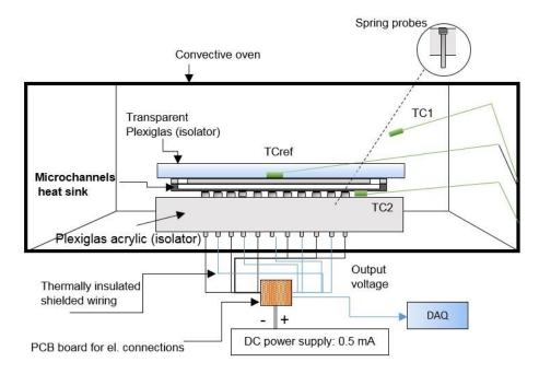
**Figure 3. 15** Side view of the calibration assembled device. The microchannels heat sink is mounted between two Plexiglas frames and the sensor pads are connected to the power supply and the data acquisition device. TC1, TC<sub>ref</sub>, TC2 are the three K-type thermocouples.
