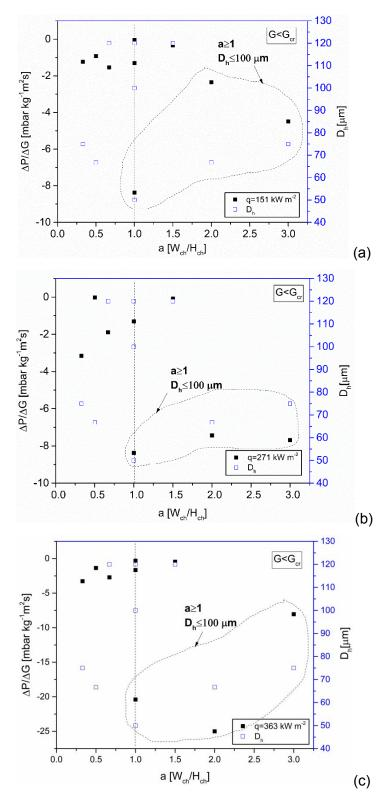
Figure 4. 12  $\Delta P/\Delta G$  slope and  $D_h$  for the two-phase region as a function of the aspect ratio of the microchannel cross section for (a)  $q = 151 \text{ kW m}^{-2}$  (b)  $q = 271 \text{ kW m}^{-2}$  and (c)  $q = 363 \text{ kW m}^{-2}$ .
