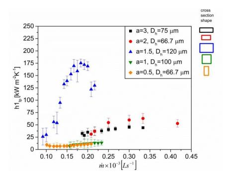
**Figure 4. 24** Local time averaged heat transfer coefficient calculated at location of sensor T1 as a function of mass flow rate at  $T_{inlet}$ = 81 °C, at q = 271 kW m<sup>-2</sup> for the designs with a = 3, 2, 1.5, 1 and 0.5 and  $D_h = 75$ , 66, 120, 100, 66.7  $\mu$ m.
