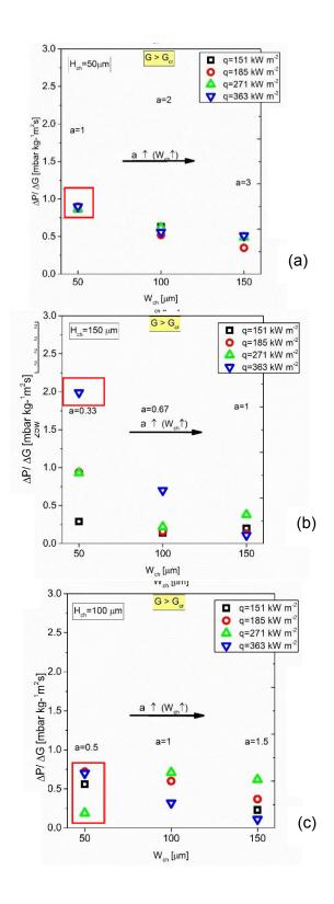
**Figure 4.** 7 Effect of increasing width for three constant heights of (a)  $H_{ch} = 50 \, \mu m$  (a=1, 2, 3 and  $D_h = 50 \, \mu m$ , 66.7  $\mu m$  and 75  $\mu m$ ) (b)  $H_{ch} = 100 \, \mu m$  (a = 1.5, 1, 0.5) and  $D_h = 120 \, \mu m$ , 100  $\mu m$  and 66.7 $\mu m$ ) and (c)  $H_{ch} = 150 \, \mu m$  (a = 1, 0.67, 0.33 and  $D_h = 150 \, \mu m$ , 120  $\mu m$  and 75 $\mu m$ .
