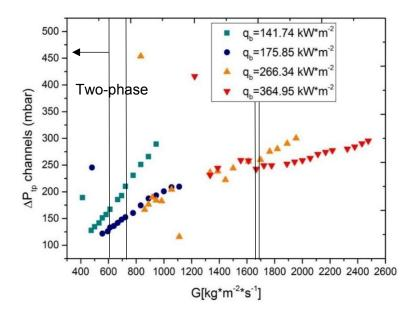
**Figure 4. 18** Two-phase pressure drop averaged over a time interval of 5 min as a function of mass flux for the heat fluxes of 141.74 kW m<sup>-2</sup>, 175.85 kW m<sup>-2</sup>, 266.34 kW m<sup>-2</sup> and 364.95 kW m<sup>-2</sup> measured for the design 2A with  $\alpha = 2$  at  $T_{intet} = 81$  °C.
