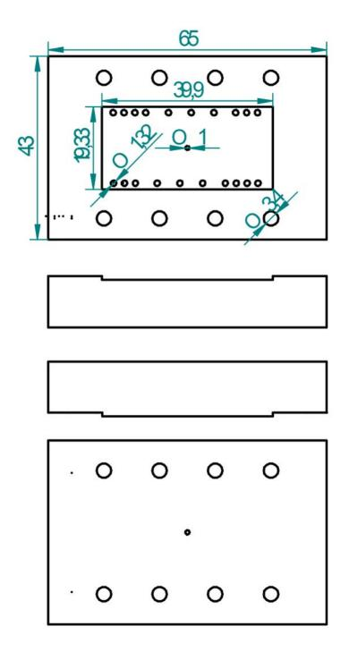
Figure A. 4 Case for oven calibration from polycarbonate.
