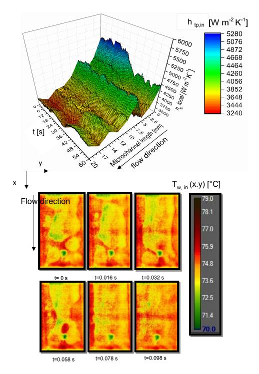
**Figure 6. 9** (a) 3D plot of the spatially averaged  $h_{tp,in}$  across the microchannel width at 9 equally spaced positions along the microchannel domain, as a function of time for  $q = 57.13 \text{ kW m}^{-2}$  and  $G = 36.87 \text{ kg m}^{-2} \text{ s}^{-1}$ . (b) Sequence of IR images that show the
