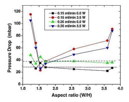
Figure 2. 12 Experimentally determined pressure drop across the microchannel versus aspect ratio (a), at the power of 3.5 W from the study of Singh et al. [78]. The theoretical single-phase pressure drop values are shown by dash-dot and dashed lines for the mass flow rates of 0.15 and 0.20 ml min<sup>-1</sup> respectively [78].
