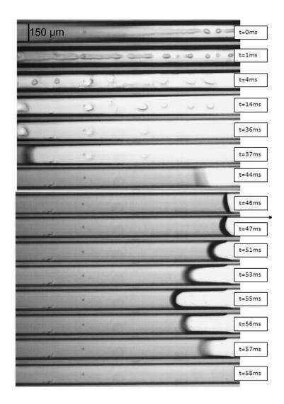
Figure 4. 28. Image sequence of periodic cycles of instabilities for a = 3,  $D_h = 75 \mu m$ , at the heat flux of 271 kW m<sup>-2</sup>,  $T_{inlet} = 25$  °C. The observed flow patterns were annular flow, mist flow and plug flow and were recorded at 5130 Hz. The width of the microchannels is 150  $\mu m$ .
