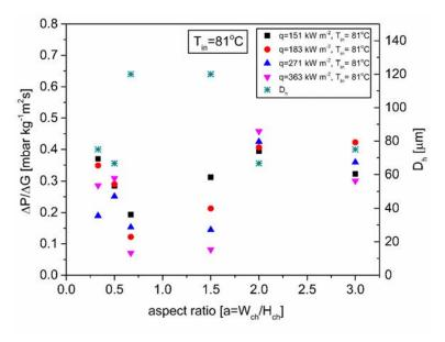
**Figure 4.** 17  $\Delta P/\Delta G$  as a function of aspect ratio and  $D_h$  for all heat fluxes for (a)  $T_{inlet} = 25$ °C and (b)  $T_{inlet} = 81$  °C.
