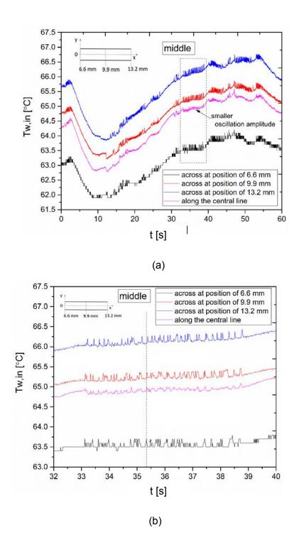
**Figure 6. 27** (a) Interfacial wall temperature fluctuations measured at x = 6.6 mm, 9.9 mm and 13.2 mm from the channel entrance. Spatially averaged across the microchannel and along the channel centreline for the middle of the microchannel for G = 73.74 kg m<sup>-2</sup> s<sup>-1</sup> and Q = 38.54 kW m<sup>-2</sup> for the time interval of 60 s and (b) zoom in the interfacial wall temperature fluctuations from 32 to 40 s.
