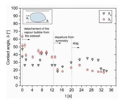
**Figure 6. 45** The advancing and receding contract angle between the bubble and the channel sidewall during single bubble growth observed to occur near a superheated layer adjacent to the sidewall of the microchannel. The contact angles were measured using Image J software from the high-speed images.
