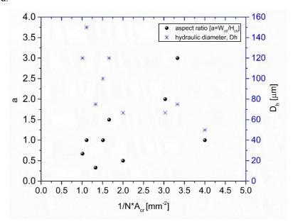
Figure 4. 9 Aspect ratio of the channel as a function of  $1/N A_{cr}$  and  $D_h$
