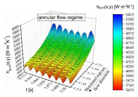
**Figure 6. 13** 3D plot of interfacial  $h_{tp,in}(x, y)$  as a function of time for  $G = 36.8 \text{ kg m}^{-2} \text{s}^{-1}$  and  $q = 57.13 \text{ kW m}^{-2}$ .
