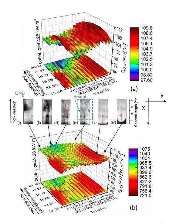
**Figure 5. 11** (a)  $T_w$ , (x, y, t) (b)  $h_{tp}$  (x, y, t) during a cycle of dryout at q = 42.48 kW·m<sup>-2</sup> at the channel outlet. The observed flow patterns were bubbly (i), slug (ii), annular (iii), annular dryout (iv), dryout (v) and liquid rewetting (vi).
