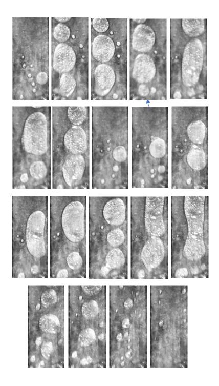
**Figure 6. 10** Image sequence of high-speed visualisations obtained from ITO/glass channel base for  $q = 55.23 \text{ kW m}^{-2}$  after ONB at  $G = 110.62 \text{ kg m}^{-2} \text{ s}^{-1}$ .
