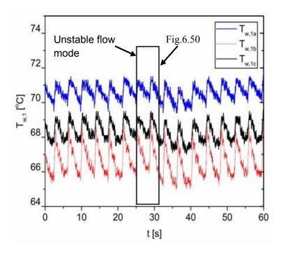
Figure 6. 49 Local wall temperature measurements were obtained at the channel entrance as a function of time during two-phase flow boiling for  $G = 14.78 \text{ kg m}^{-2} \text{s}^{-1}$  and  $q = 43.80 \text{ kW m}^{-2}$ . The measurements were obtained at three locations across the channel width  $(T_{w,1}: \text{left channel edge}, T_{w,b1}: \text{centre}, T_{w,c1}: \text{other channel edge})$  at the channel entrance (position 1).
