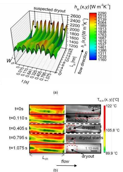
**Figure 6. 59** (a) 3D plot of the two-dimensional  $h_{tp}(x, y)$  as a function of time and channel length for  $G = 14.78 \text{ kg}^{-2}\text{s}^{-1}$  and  $q = 92.3 \text{ kW m}^{-2}$  and (b) correlation between thermal images obtained from the IR camera and optical images from the high-speed camera at the outlet.
