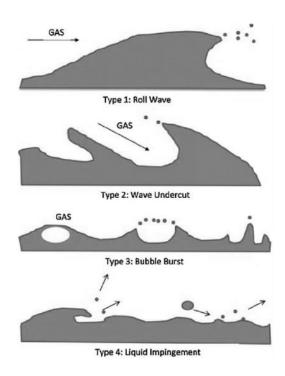
Figure 2. 16 Different droplet entrainment mechanisms [91].
