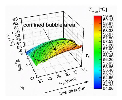
**Figure 6. 40** (a),(b),(c),(d) show 3D plots of inner wall temperature  $(T_w)$  distribution across the channel during single bubble growth. Wall temperature is presented as a function of channel width and channel length. The range of the temperature of the bubble  $(T_b)$  is noted on the scale of each graph. The bubble was fully confined by the channel width in (d) where the highest temperature drop was measured to occur along the channel length.
