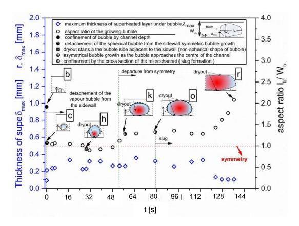
Figure 6. 43 Aspect ratio of a single bubble growing in a microchannel during flow boiling conditions presented as a function of time (from high-speed images). In the same Figure, the superheated layer width (from IR images) observed to grow adjacent to the wall is plotted as a function of time.
