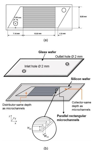
**Figure 3. 1** (a) Geometry of the inlet and outlet manifold and (b) split view of the microchannel heat sink device.
