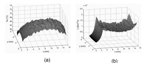
Figure 2. 25 Chip wall temperature and heat transfer coefficient distributions ( $T_{in}$ =30.8 °C,  $\Delta P$ =30.41 kPa, G=110.1 kg m<sup>-2</sup>s<sup>-1</sup>, q=141.92 kW m<sup>-2</sup>,  $\chi_e$ =0.5268, Re=65.2). Results from the study of Jinliang et al. [115]..
