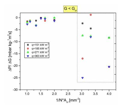
**Figure 4. 10**  $\Delta P/\Delta G$  was plotted as a function of  $1/NA_{CT}$  where  $NA_{CT}$  is the product of the number of the microchannels N and  $r_{CT}$  the cross sectional area of the channels.
