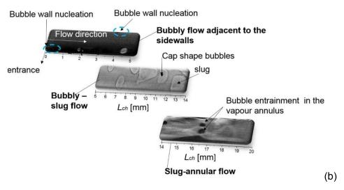
**Figure 6. 62** High spatial and temporal resolution 2D plot of h(x, y, t) as a function of time for  $G = 298 \text{ kg m}^{-2} \text{ s}^{-1}$  and  $q = 179.2 \text{ kW m}^{-2}$  and (b) flow visualisation from high –speed camera results for the inlet, middle and outlet of the microchannel at t = 0.288 s.
