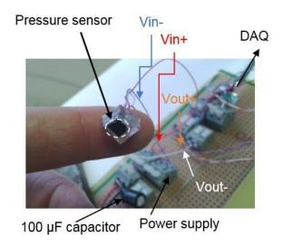
Figure 3. 22 Pressure sensor and electrical connections.
