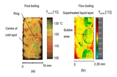
Figure 6. 1. (a) 2D wall temperature measurements obtained with liquid crystal thermography method by Kenning (1992) [106] for pool boiling. The photograph shows the crystal layer on the rear of the plate. The nucleation sites are related to the centres of cold spots and the rings. (b) Two-dimensional IR image obtained during flow boiling from the transparent to infrared PDMS side of the microchannel using IR thermography with FC-72 dielectric
