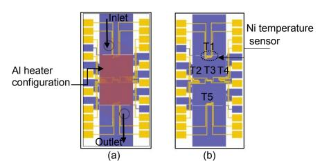
Figure 3. 3 Layout of masks used in microfabrication of silicon microchannel heat sinks. (a)
