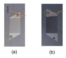
**Figure 3. 8** Holes in the inlet and outlet manifolds of the silicon microchannel heat sinks using a (a) drilling technique (b) powder blasting technique.
