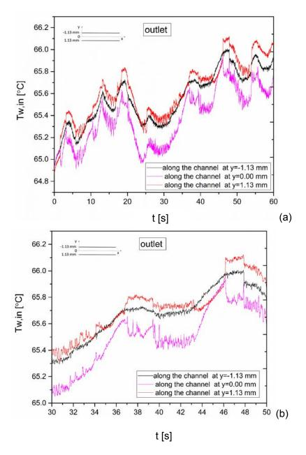
**Figure 6. 29** (a) Inner wall temperature fluctuations measured at three positions (at the corners: -1.13 mm, 1.13 mm and 0 mm centre) across the microchannel of the outlet for  $G = 73.74 \text{ kg m}^{-2} \text{ s}^{-1}$  and  $Q = 38.52 \text{ kW m}^{-2}$  and  $Q = 38.52 \text{ kW m}^{-2}$
