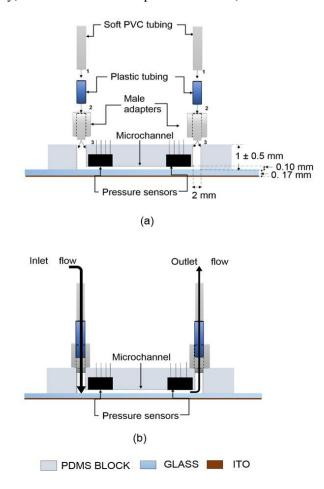
Figure 3. 31 PDMS device (a) before the microfluidic connections and (b) after the microfluidic connections have been done.
