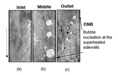
**Figure 6. 5** Optical images recorded at 200 Hz from the optically transparent ITO/glass channel base for the.(a) inlet (b) middle and (c)outlet for  $G = 101.2 \text{ kg m}^{-2} \text{ s}^{-1}$  and  $q = 45.26 \text{ kW m}^{-2}$  (ONB). The arrow on the left shows the liquid flow direction.
