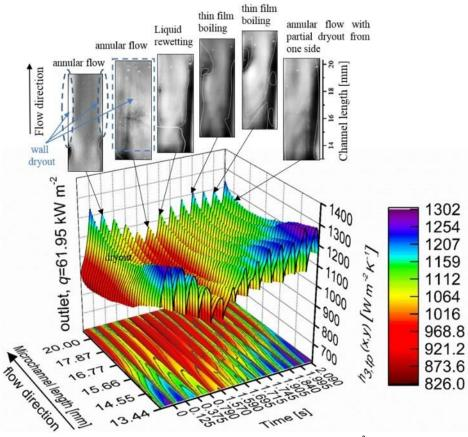
**Figure 5.** 13  $h_{tp}(x, y, t)$  during a cycle of dryout at q = 61.95 kW·m<sup>-2</sup> at the channel outlet (3).
