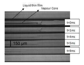
Flow visualisation obtained with high-speed camera at 1000 Hz that shows evaporation at the inlet of the channels at G = 337.22 kg m<sup>-2</sup> s<sup>-1</sup> and q = 151 kWm<sup>-2</sup> for the design of  $\alpha = 3$ ,  $D_h = 75 \mu m$  at location of sensor T5.
