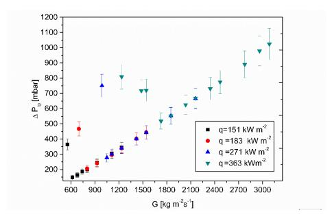
Figure 4. 19 Two-phase pressure drop averaged over the time interval of 5 min as a function of mass flux for the heat fluxes of 145.31 kW m<sup>-2</sup>, 178.16 kW m<sup>-2</sup>, 273.97 kW m<sup>-2</sup> and 384.77 kW m<sup>-2</sup> for the design 2A with a = 2 at  $T_{inlet} = 25$  °C.
