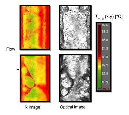
**Figure 6. 16** (a) Thermal image recorded with IR camera from PDMS side and (b) simultaneous optical image recorded from the transparent ITO/glass heater base during annular flow regime for  $G = 147.2 \text{ kg m}^{-2} \text{ s}^{-1}$  and  $q = 99.7 \text{ kW m}^{-2}$ . Annular flow regime with local instability induced by bubble burst mechanism.  $T_{w} > 84 \text{ °C}$  under the dispersed drop.
