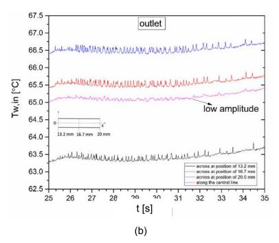
Figure 6. 28 (a) Inner wall temperature fluctuations measured at three positions (13.2 mm, 16.2 mm and 20 mm) across the microchannel and along the channel central line for the outlet of the microchannel for G = 73.74 kg m<sup>-2</sup> s<sup>-1</sup> and q = 38.52 kW m<sup>-2</sup> for a time interval of 60 s (b) interfacial wall temperature fluctuations from 25 to 35 s.
