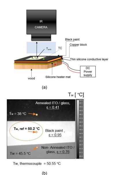
Figure 3. 28 (a) Setup for calibration of surface emissivity and (b) thermal image from the IR used to measure the emissivity of ITO coated glass and annealed ITO coated glass in reference to the emissivity of the black paint.
