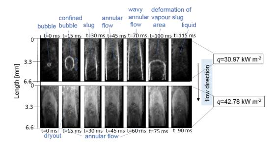
**Figure 5. 3** Typical flow regimes at the inlet of the investigated high aspect ratio rectangular microchannel. Sequence of optical images from the heater side of the inlet for  $G = 7.37 \text{ kg m}^{-2} \text{s}^{-1}$  and  $q = 30.97 \text{ kW m}^{-2}$  and  $42.78 \text{ kW m}^{-2}$ . The images were cropped to show the section where the temperature measurements were carried out.
