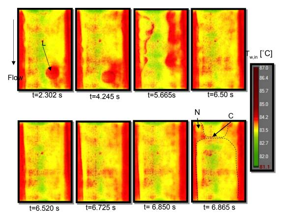
L: liquid V: vapour N: nucleation of bubbles D: dryout C:Collision
