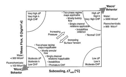
**Figure 2.** 3 Overall performance trends of small diameter (50  $\mu$ m <  $D_h$  < 1000  $\mu$ m) two-phase microchannel heat sinks, produced by Lee and Mudawar [49].
