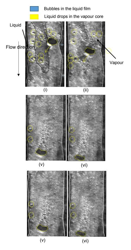
**Figure 6. 18** Annular flow regime with dispersed droplet for  $G = 147.2 \text{ kg m}^{-2} \text{ s}^{-1}$  and  $q = 99.7 \text{ kW m}^{-2}$ .
