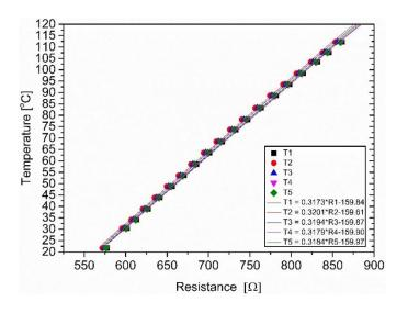
Figure 3. 16 Calibration curve of temperature sensors.
