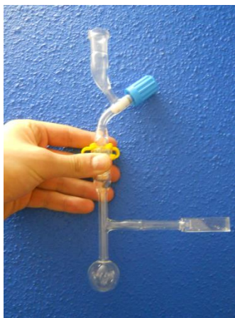
Figure A6: designed cuvette for freeze pump procedure.
