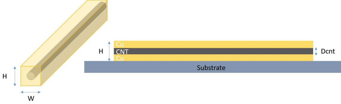
Figure 4.14: Cu-CNT composite unit cell geometry sketch.
