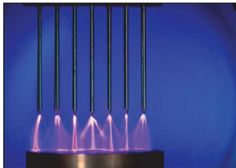
Figure 1.4: Example of a Corona reactor [7]
