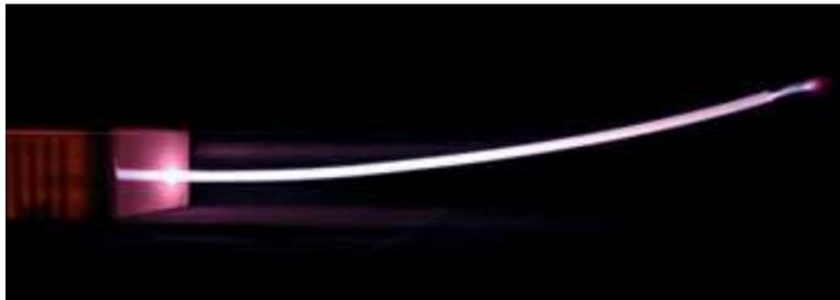
Figure 1.8: Plasma jet propagating inside a flexible tube of about 1m length before to be launched in the ambient air. Such device can be used, for instance, for endoscopic plasma treatment : Example of direct plasma application [26]
