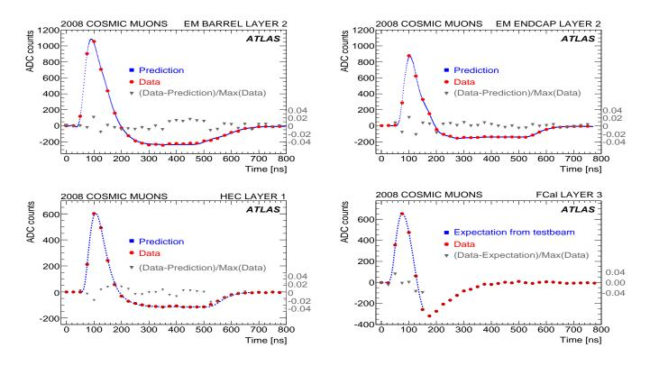
**Fig. 13.** Typical pulse shapes, recorded during the cosmic ray campaign, for a given cell in the second layer for the barrel (top left) and the endcap (top right) of the EM calorimeter, as well as in the first layer of the HEC (bottom left) and in the third layer of the FCal (bottom right). The relative difference between data and prediction is indicated by triangles on the right scale.
