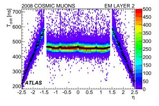
Fig. 16. Drift time measurement in the cells of the EM calorimeter second layer with E > 1 GeV for the 2008 cosmic muon run. The dots correspond to drift time values averaged in  $\phi$ .
