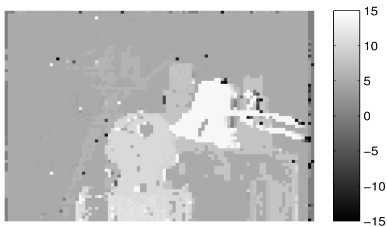
Figure 3.21: Disparity map using the MMA algorithm (33.89dB; 0.14bpp) with \lambda = 1.8 .
