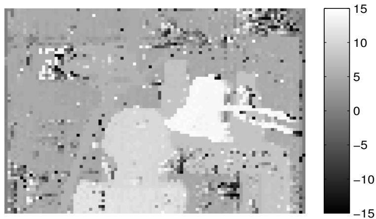
Figure 3.20: Disparity map using BMA (34.12dB; 0.27bpp).
