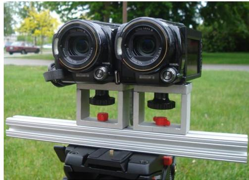
Figure 2.2: Stereoscopic camera
