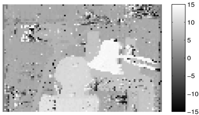
Figure 3.20: Disparity map using BMA (34.12dB; 0.27bpp).
