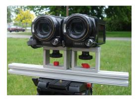
Figure 2.2: Stereoscopic camera
