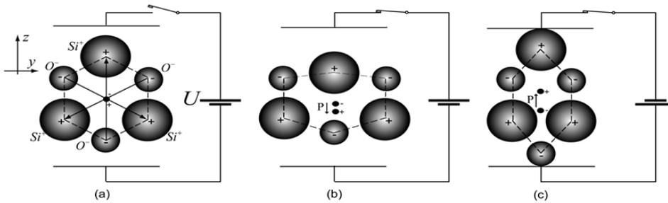
Figure 2.8: Inverse piezoelectricity effect at molecular level [153].
