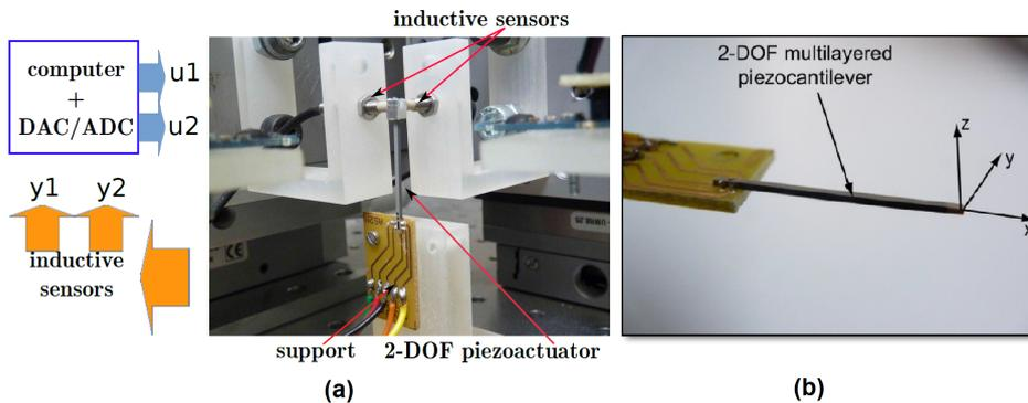
Figure 6.1: (a) The experimental setup diagram (b) The 2-DOF piezocantilever.
