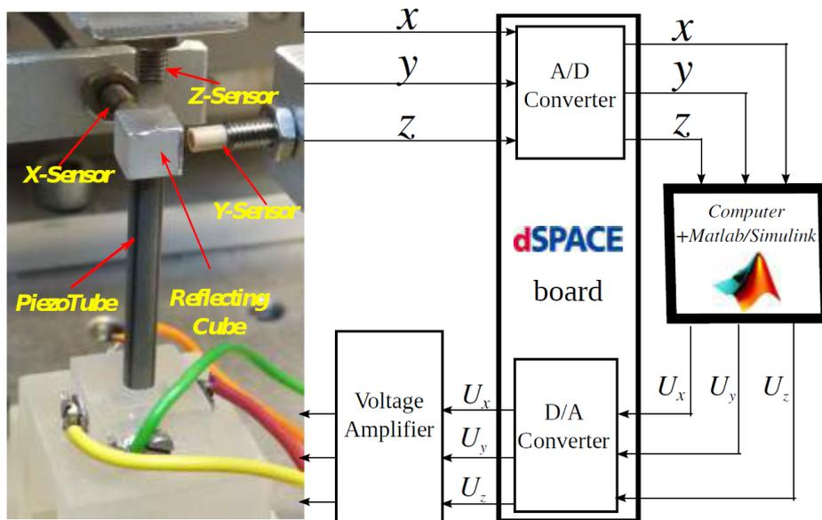
Figure 6.6: The PT230 experimental setup.
