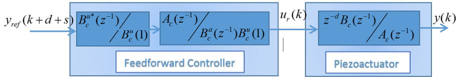
Figure 3.5: Feedforward controller for zero phase error tracking.
