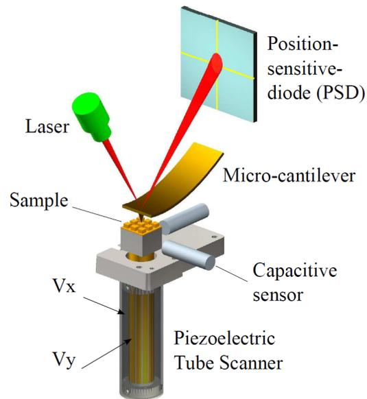
Figure 5.4: Schematic of an AFM [44].
