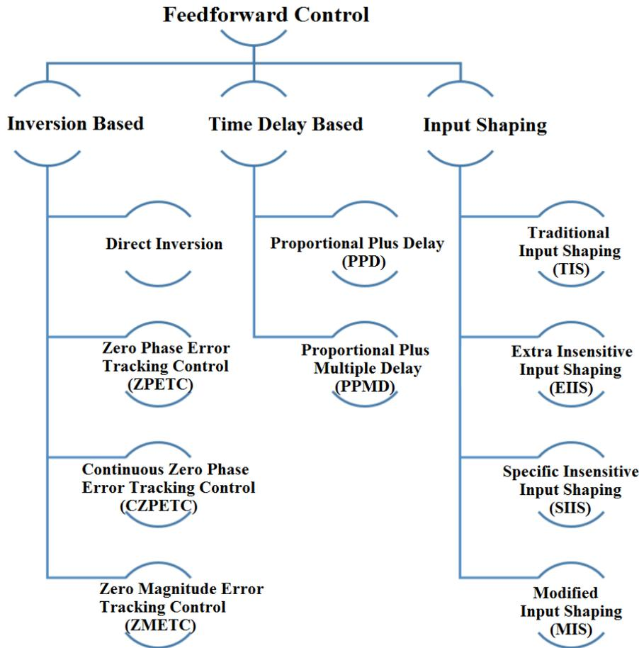
Figure 3.2: Classification of some feedforward control schemes.
