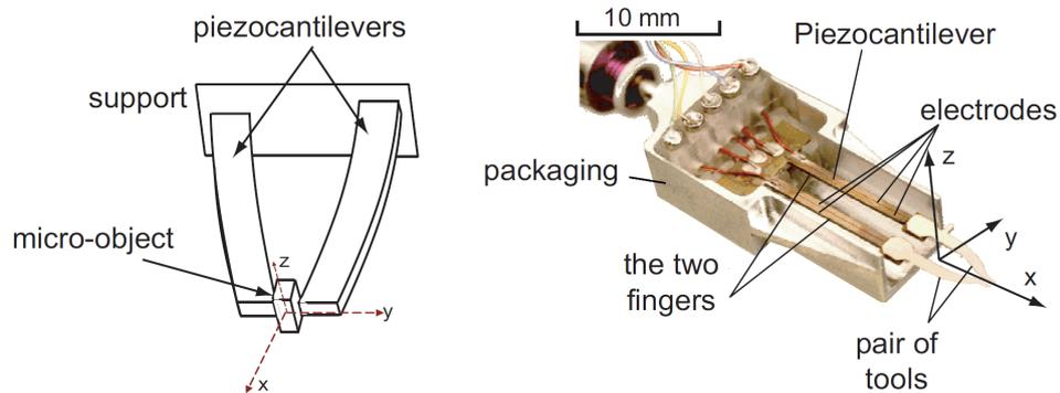
Figure 5.5: The 4-DOF Microgripper with 2-DOF piezocantilevers [150].
