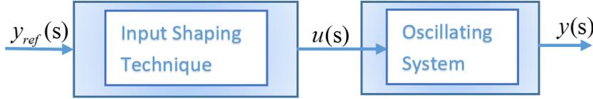
Figure 3.9: Block diagram of a feedforward control of oscillation by an input shaping technique.
