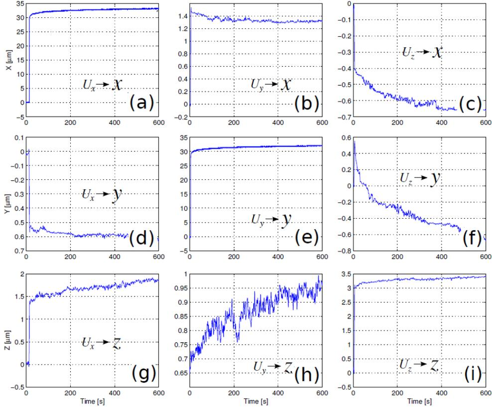
Figure 6.8: Creep characterization over a period of 600s.
