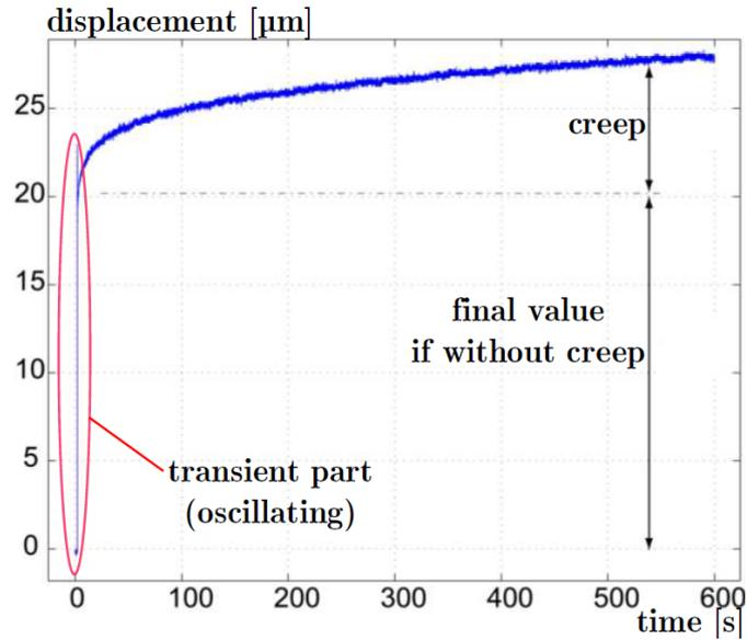
Figure 2.10: Example of creep in piezoelectric cantilever
