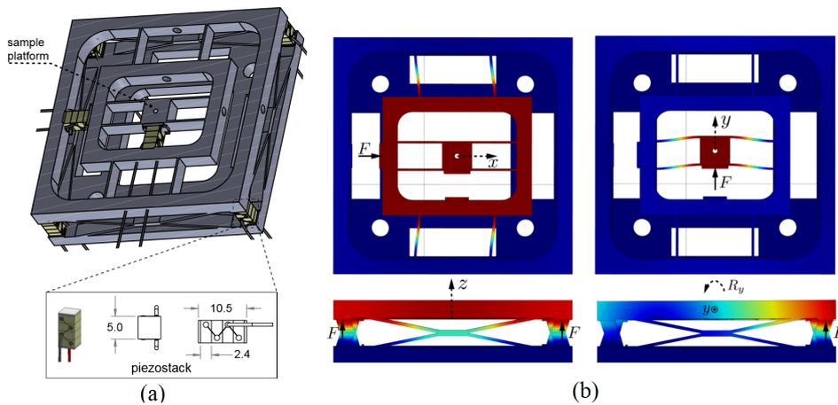
Figure 5.6: (a) 5-DOF piezoelectric positioner CAD model (b) Structure deformations [149].
