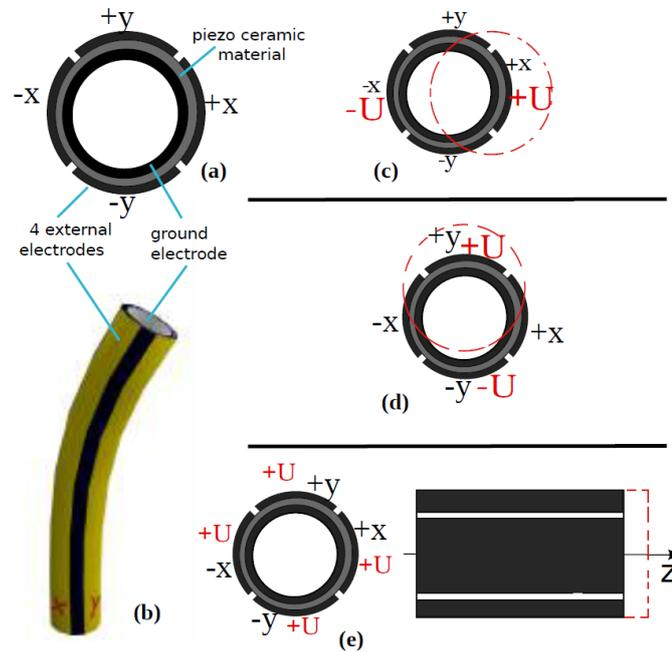
Figure 6.5: Piezoelectric tube structure and operation:(a) Top view, showing four external electrodes and an internal ground electrode, separated by piezoelectric material; (b) A perspective view of the piezoelectric tube; (c) deflection along X axis; (d) deflection along Y axis, and (e) elongation along Z axis.
