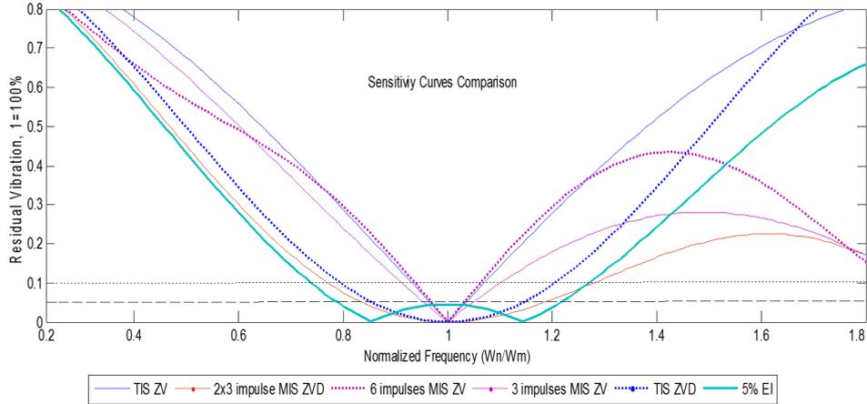
Figure 4.12: TIS, MIS, EI sensitivity curves comparison - Simulation.
