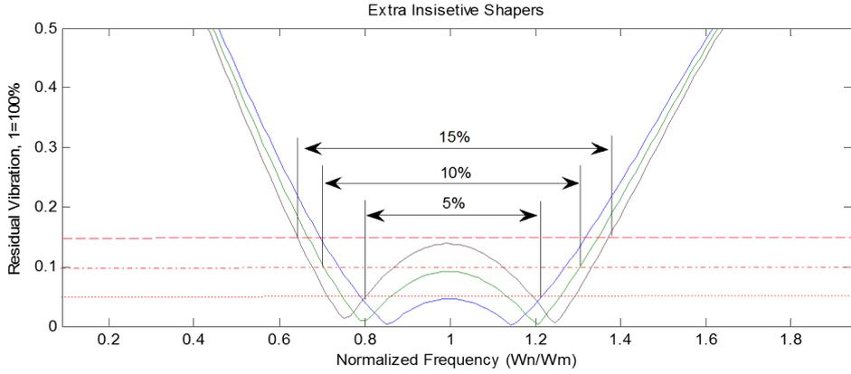
Figure 4.3: EI shapers sensitivity curves - Simulation.
