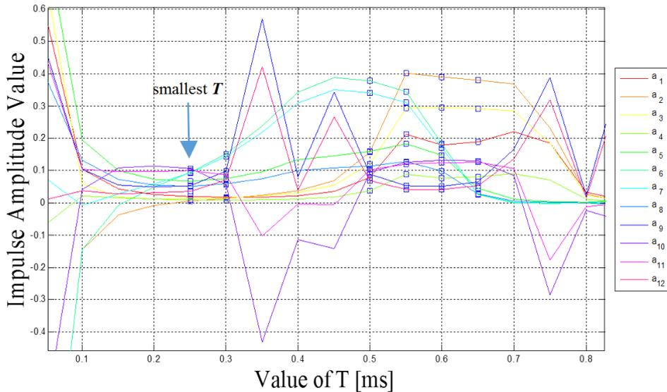
Figure 5.3: Shapers impulse amplitudes versus  $T$  for a system with three inputs and four impulses per shaper.
