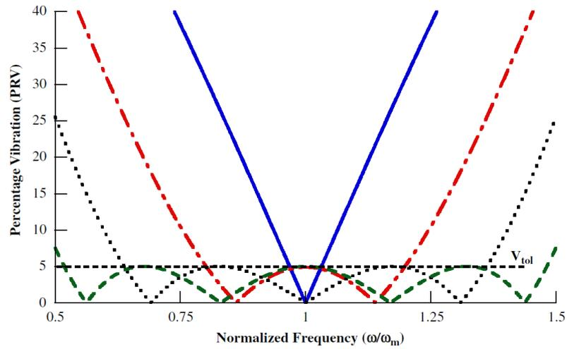
Figure 4.4: Sensitivity curves for extra insensitive method shapers, ---- zero vibrations, -.-.- extra insensitive, .... two-hump extra insensitive, - - - - three-hump extra insensitive [58].
