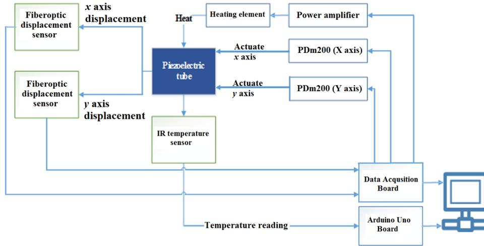
Figure 6.13: Schematic of the experimental setup working flow.
