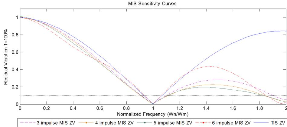
Figure 4.9: MIS ZV shapers sensitivity curves - Simulation.
