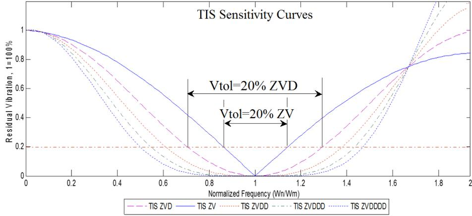
Figure 4.1: TIS Sensitivity Curves - Simulation.
