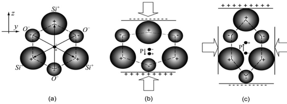
Figure 2.7: Direct piezoelectricity effect at molecular level [153].
