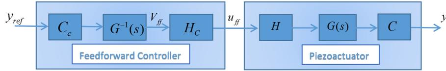
Figure 3.3: An inversion-based feedforward method to compensate for dynamics  $G$ , creep  $C$  and hysteresis  $H$  in piezoactuators.
