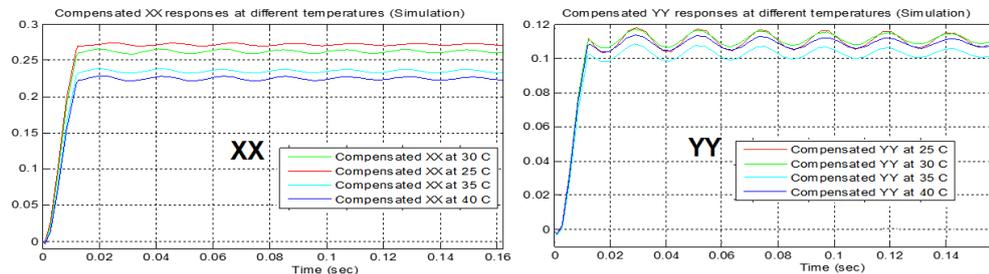
Figure 6.27: XX and YY Compensated responses at different temperatures (Simulation).
