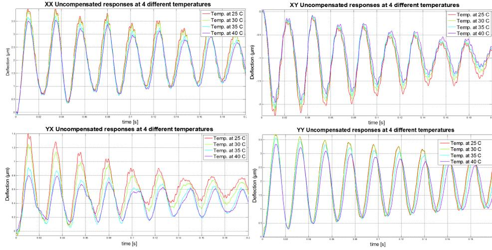
Figure 6.14: Uncompensated XX, XY, YX and YY responses at 4 different temperatures (Experimental).
