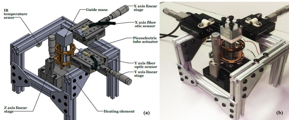
Figure 6.11: (a) The setup CAD drawing (b) The actual piezoelectric tube setup.
