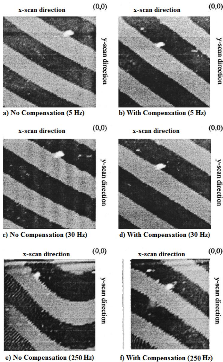
Figure 2.14: High speed compensation of piezoactuator dynamics [73].
