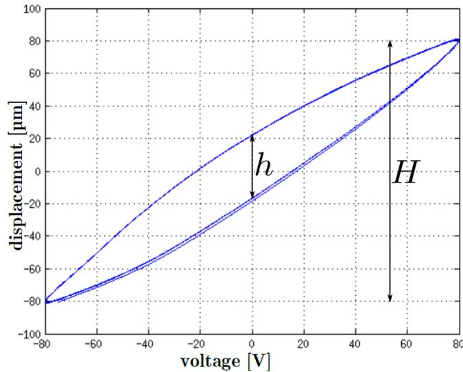
Figure 2.11: Example of Hysteresis in piezoelectric cantilever.
