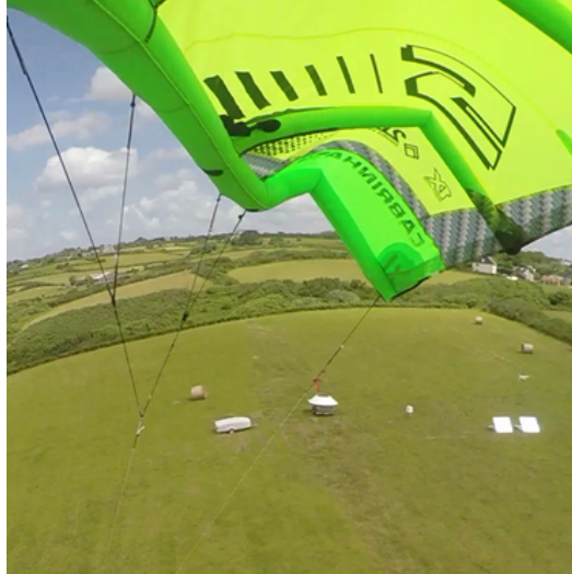
Figure 5.2 – Buckling of a LEI kite during flight. Picture taken during experimental tests of Behrel Behrel (2017)
