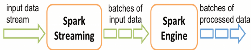
FIGURE 2.6: Workflow Spark Streaming
