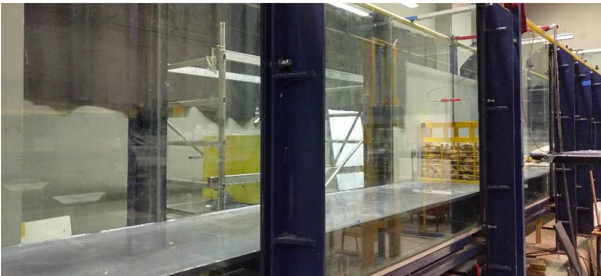
Figure 4.4: False floor and breakwater model, Istres & Banyuls
