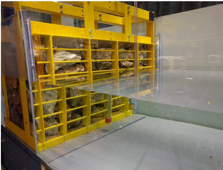
Figure 4.6: Oblique and top view of the cage, B=24cm, Istres & Banyuls
