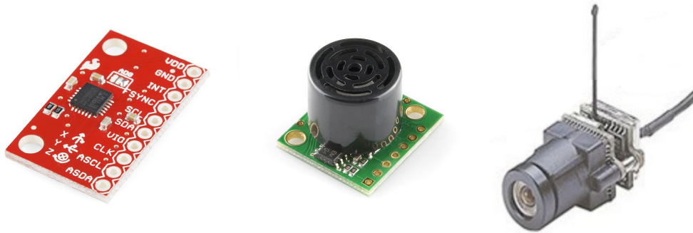
Figure 2.4 – Sensors used for NON-A blimp prototype: IMU MPU-6050 (left), US range finder LV-MaxSonar-EZ1 (middle), wireless camera ALM-2451G (right)
