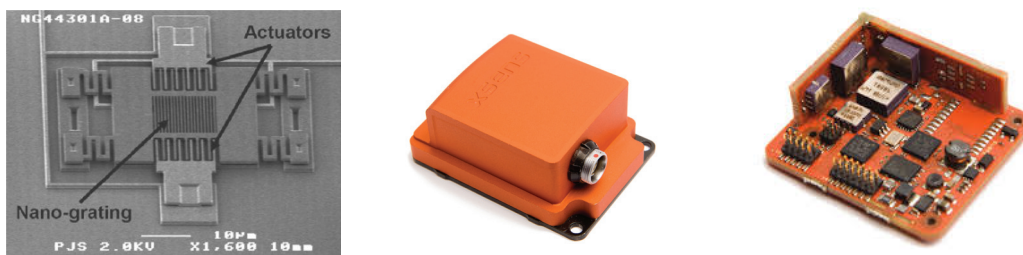
Figure 1.7 – An example MEMS accelerometer produced by Sandia National Laboratories (left), A commercial IMU produced by Xsens (middle) and the inside of IMU (right)
