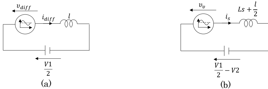
Fig 74. (a) Average model of the subsystem i_{diff} , (b) Average model of the subsystem i_s
