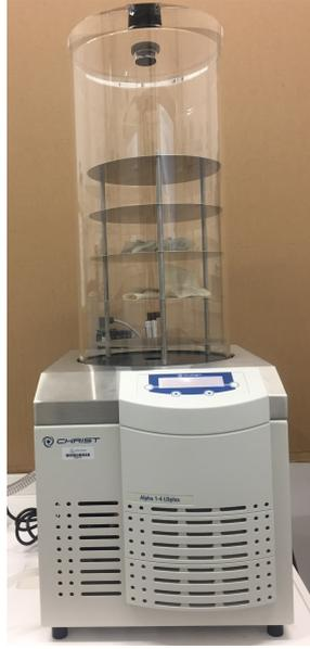
Figure 2.11 – Freeze-dryer used in the study
