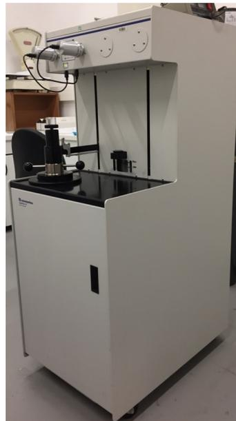
Figure 2.14 – Mercury intrusion porosimetry device
