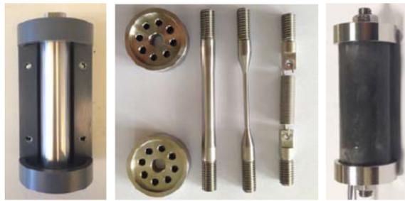
Figure 4.20 – PVC mould and three types of restraints [282].
