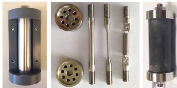
Figure 4.20 – PVC mould and three types of restraints [282].
