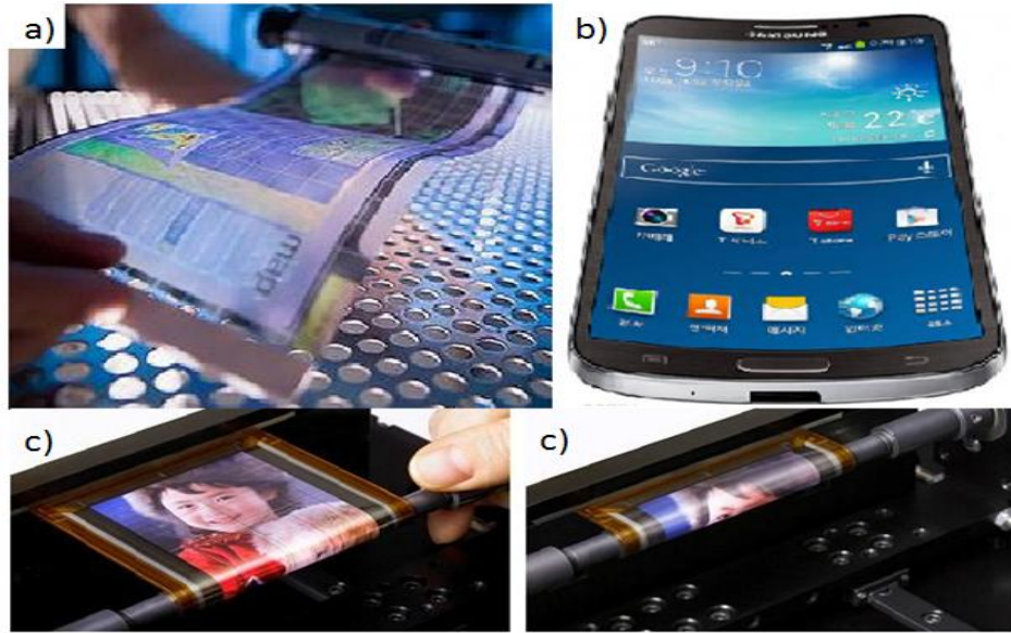
Figure 1.8: Applications of flexible displays. a) Electronic paper by HP and ASU [15]. b) Smart phone by Samsung [16]. c) Rollable screen by Sony [17].
