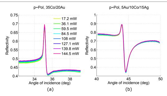
Figure 5.2 – The angular dependence of the linear reflectivity in (a) the sample (20 nm)Au/ (35 nm)Co/ sapphire and (b) the sample of (5 nm)Au/ (10 nm)Co/ (15 nm)Ag/ fused-silica at different pump powers, represented by different colors. The excitation is centered at wavelength 1560 nm and p-polarized.
