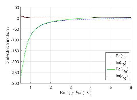
Figure 2.1 – Comparison of the dielectric function of silver estimated by Drude model (dots) and that measured experimentally on a 30 nm silver thin film (solid lines) [74]
