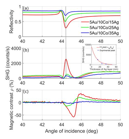
Figure 3.9 – Angular dependence of (a) linear reflectivity at 1560 nm, (b) SHG intensity at 780 nm and (c) transversal nonlinear magnetic contrast  $\rho$  in trilayer (5 nm)Au/(10 nm)Co/(15-25-35 nm)Ag. The SHG peak at 44.5 deg corresponds to the linear SPP( $\omega$ ) mode, confirmed by the dip of linear reflectivity at the same angle.
