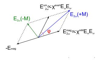
Figure 2.5 – Phasor diagram of the non-magnetic and magnetic SH fields, denoted as  $E_{2\omega}^{nm}$  and  $E_{2\omega}^{mag}$  respectively, and their interference  $E_{2\omega}(\pm M)$ .
