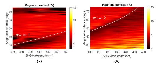
Figure 4.7 – The false-color images of the SH magnetic contrast for (a)  $E_x \parallel p_T$ , where the white line shows the theoretical dispersion for the second-harmonic anomaly  $m_{nl} = -1$ , and (b)  $E_x \parallel p_L$ , where the white line marks the dispersion of  $m_{nl} = -2$ .
