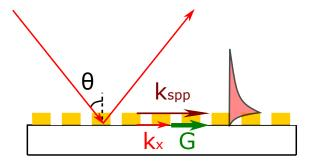
Figure 2.11 – Excitation of SPP by a diffraction grating.
