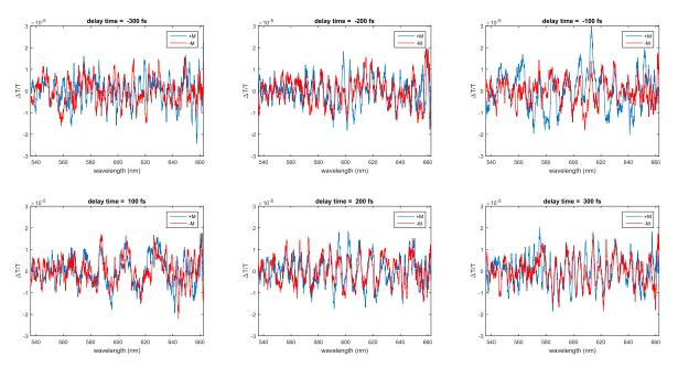
Figure 5.10 – Spectrally-resolved linear cross-correlation of a reference wave with the mSHG signal for opposite directions of the magnetization M (red and blue lines) at different fixed time delays.
