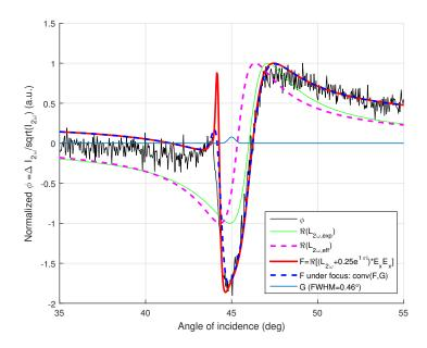
Figure 3.15 – Reverse approach: fit the magnetic contrast  $\phi$  to estimate the Lorentzian function.  $\phi = \frac{dI(\pm M)}{\sqrt{I}}$  (black solid) is well fitted with  $F = \Re\{(b+Ld)\}$  (red solid) in the structure of (5 nm)Au/(10 nm)Co/(25 nm)Ag. The measurement was performed at the fundamental wavelength 1200 nm.
