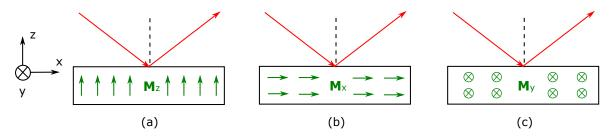
Figure 2.2 – Three configurations of magneto-optical Kerr effects: (a) polar, (b) longitudinal and (c) transversal. Plane of incidence is the xz plane.
