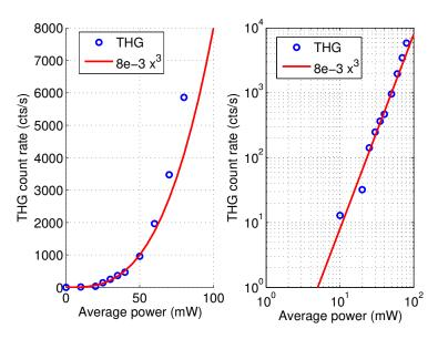
Figure B.1 – Power dependence of the THG in the trilayer (5 nm) Au/(10 nm) Co/(15 nm) Ag at angle of incidence 43.9° in the normal scale (left) and in logarithmic scale (right).
