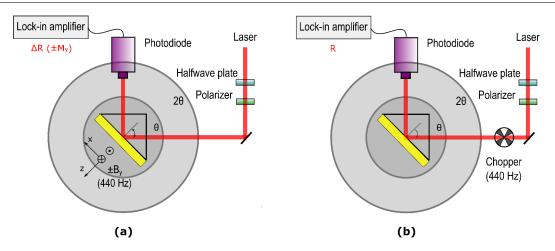
Figure 3.2 – Scheme of a linear magneto-plasmonic setup employing Kretschmann configuration. (a) Measurement of magnetization-induced variations in reflectivity  $\Delta R(\pm M)$ . (b) Measurement of the average reflectivity R. The ratio  $\Delta R/R$  implies the normalized transversal MOKE signal.
