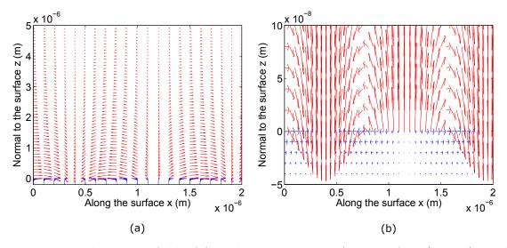
Figure 2.8 – The vector field of SPP localized at gold/air interface (z=0) at the wavelength 1560 nm. The red vectors illustrate SPP field in the air. The blue vectors are SPP in gold. (a) The extension of SPP in both media. The skin depth for electric field is twice higher than the penetration depth of intensity. (b) A zoom-in to the interface shows the flow of electric field.
