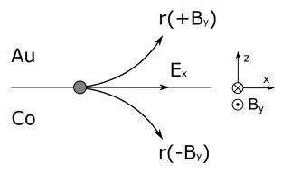
Figure 3.21 – Illustration of a charge at the boundary between two conducting media Co and Au. The trajectory of the moving charge is deflected towards different directions when the external magnetic field is reversed.
