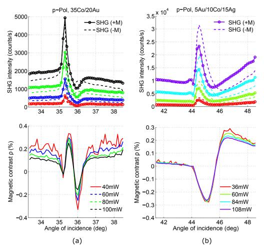
Figure 5.1 – The angular dependence of the mSHG intensity and the SH magnetic contrast  $\rho$  in (a) the bilayer (20 nm)Au/ (35 nm)Co/ sapphire and (b) the trilayer (5 nm)Au/ (10 nm)Co/ (15 nm)Ag/ fused-silica at different pump powers, represented by different colors. The fundamental wavelength in both cases is 1560 nm. In the top row, the dotted lines illustrate the SHG(+M) while the dashed lines are used for SHG(-M).
