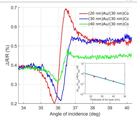
Figure 3.7 – Angular dependence of linear transversal MOKE measured on the bilayer (20-30-40 nm)Au/(30 nm)Co at the wavelength 633 nm.
