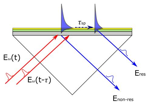
Figure 5.4 – In the Kretschmann configuration, two fundmental pulses, delayed by time  $\tau$ , generate cross-product SH field  $E_{\omega}(t)E_{\omega}(t-\tau)$  at bottom and top interfaces of the multilayer.  $E_{non-res}$  is the SH field at the bottom interface.  $E_{res}$  refers to the coupling of SH polarization at the top interface and the radiative SPP(2 $\omega$ ). The propagation of SPP along the metal/air interface cause the delayed arrival of the resonant pulse.
