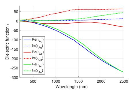
Figure 2.7 – The real and imaginary parts of the dielectric functions of silver (blue), gold (green) [74] and cobalt (red) [94], the three metals used extensively in this work.
