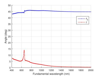
Figure 3.16 – Dispersion of the Lorentzian function is shown via  $\theta_0(\lambda)$  (blue) and  $\Gamma(\lambda)$  (red).
