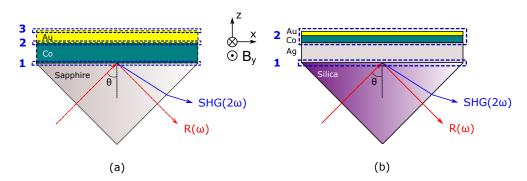
Figure 3.1 – Kretschmann configuration applied for the metal/ferromagnet multilayers (a) Bilayer structure of Au/Co deposited on sapphire. (b) Trilayer structure of Au/Co/Ag deposited on fused-silica. The dashed rectangles mark the interfaces where SH emission is considered in the later simulation.
