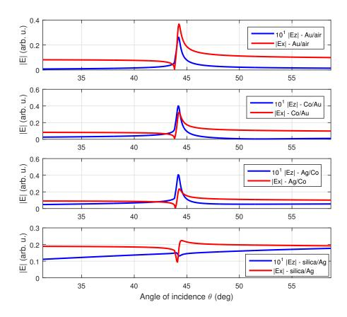
Figure 3.12 – Angular dependence of electric field |E| components of p-polarized incident light, calculated at each interface using MTM method for the structure (25 nm)Ag/(10 nm)Co/(5 nm)Au doposited on fused-silica.
