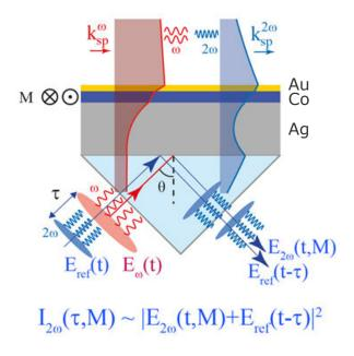
Figure 5.8 – The mSHG cross-correlation on the Kretschmann configuration.
