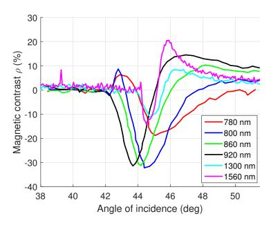
Figure 3.17 – The angular dependence of the conventional magnetic contrast  $\rho$  is broadened at short fundamental wavelengths. The graph combines the data from Ref. [6] (780-920 nm) and the data measured in this work (1300-1560 nm) for the sample of (5nm)Au/(10nm)Co/(25nm)Ag.
