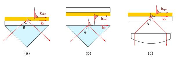
Figure 2.10 – Different geometries where SPP is excited by prism coupling: (a) conventional Kretschmann configuration (b) Otto configuration (c) modified Krestchmann configuration.
