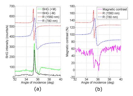
Figure 3.8 – (a) Angular dependence of SH output from the bilayer of (20 nm)Au/(30 nm)Co measured at two different magnetizations (green and black solid lines). (b) The angular dependence of the SHG magnetic contrast (magenta solid line). The linear reflectivity (arbitrary unit) at fundamental (1560 nm) and SHG (780 nm) wavelengths are shown in (a) and (b) as dashed lines in order to mark the angles of incidence where  $SPP(\omega)$  and  $SPP(2\omega)$  are excited in the linear configuration.
