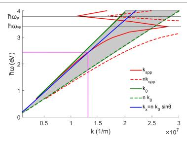
Figure 2.9 – Dispersion relations of  $k_{spp}$  at silver/air interface (red solid line),  $nk_{spp}$  at silver/substrate interface (red dashed line), light line  $k_0$  in the air (green solid line), light line  $nk_0$  in the substrate (green dashed line) and the inplane wavevector  $k_x$  at the angle of incidence  $\theta = 47$  deg (blue line). Magenta lines mark the coupling between the incident  $k_x$  and the  $k_{spp}$  at silver/air interface.
