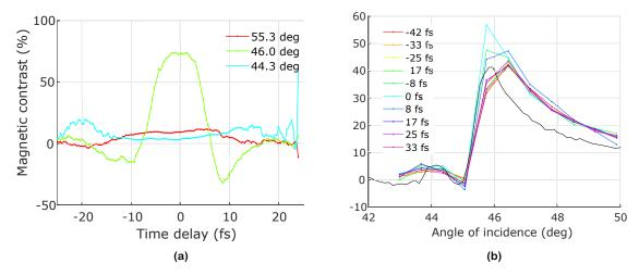
Figure 5.7 – Time-resolved second-harmonic magnetic contrast  $\rho$  of the trilayer (5 nm)Au/(10 nm)Co/(15 nm)Ag.
