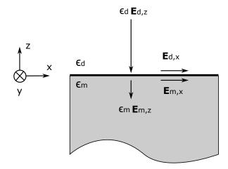
Figure 2.6 – The boundary conditions in the case of p-polarized electromagnetic fields at the interface between metal  $(\epsilon_m)$  and dielectric  $(\epsilon_d)$ .
