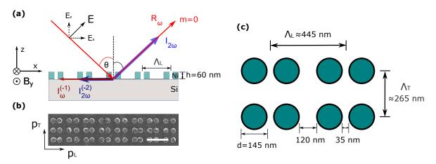
Figure 4.2 – (a) Schematic for the co-excitation of linear and nonlinear Wood's anomalies, denoted as  $I_{\omega}^{(-1)}$  and  $I_{2\omega}^{(-2)}$  respectively, in an array of nickel nanodimers. An external magnetic field is applied perpendicular to the plane of incidence. (b) Scanning electron microscopy image of the nickel nanodimers. The scale bar is 600 nm long. (c) Dimensions of the two-dimensional nanodisks array.
