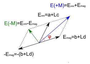
Figure 3.11 – The phasor diagram of non-magnetic and magnetic SHG fields, respectively  $E_{nm}$  and  $E_{mag}$ , taking account the non-resonant (a,b) resonant (c,d) SH components. Zero magnetic contrast, i.e. E(+M) = E(-M), happens when the phase difference is  $\varphi = \frac{\pi}{2}$
