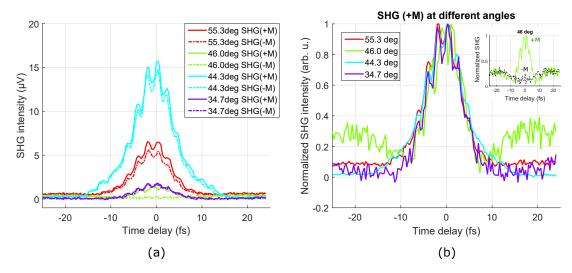
Figure 5.6 – (a) Intensity auto-correlation in the layer (5 nm)Au/(10 nm)Co/(15 nm)Ag employing the Kretschmann configuration. Each color represents for a different angle of incidence. The solid and dashed lines are the signals for +M and -M, respectively. (b) The intensity auto-correlation of the SHG (+M) pulses at different angles of incidence are normalized to unity. The inset shows the normalized intensity at angle  $46^{\circ}$  for opposite magnetizations.
