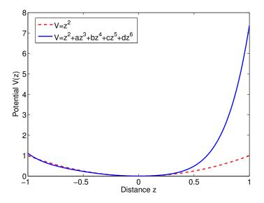
Figure 2.3 – Illustrations of the harmonic potential (red dashed line) and the power expansion of the potential (blue solid line). For large positive z, the blue line deviates from the parabolic curve and approaches the case of a potential wall.
