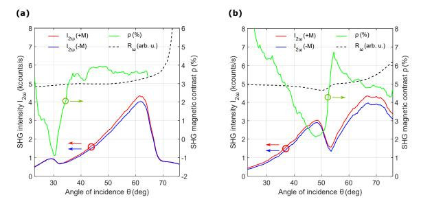
Figure 4.4 – The angular dependence of the linear reflectivity  $R_{\omega}$  (dashed black), the SH intensity  $I_{2\omega}(\pm M)$  for the two opposite directions of magnetization (solid red and blue), and the SHG magnetic contrast  $\rho$  (solid green) at the fundamental wavelength of 820 nm, measured for the case of (a)  $E_x \parallel p_T$  and (b)  $E_x \parallel p_L$ .
