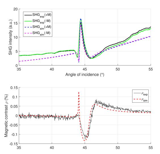
Figure 3.14 – Forward approach: (a) Simulated curves (dashed lines) are fitted with the experimental mSHG( $\pm M$ ) (solid lines) measured for the structure (5 nm)Au/ (10 nm)Co/ (25 nm)Ag excited at fundamental wavelength 1200 nm. (b) Comparison of the experimental (black) and simulated (red) magnetic contrasts. In the simulation, only one dominant  $\chi^{(2)}$ -component is considered at each interface, referring to Eq. 3.23.
