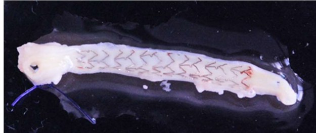
Figure 64. Photograph of a stented porcine coronary artery. The luminal side is exposed by cutting the artery longitudinally after explantation. The stent struts are clearly visible to the naked eye.
