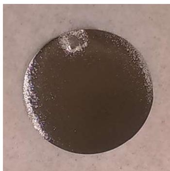
**Figure 25. Photograph of a CoCr disk after excessively intensive electropolishing (two 2-minute cycles at 9.4A).** The surface appears mirror-bright, but the edges of the sample are visibly etched. The marks at the top of the image were produced by the crocodile clip that held the sample during the electropolishing process.
