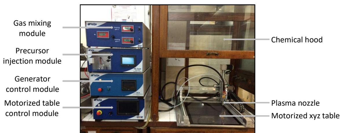
**Figure 21. Photograph of the atmospheric-pressure plasma reactor.**
