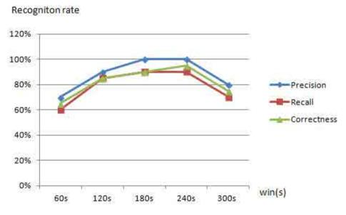
Figure A.6 Precision, recall, and correctness of the method using conflict resolution for different time window *win*
