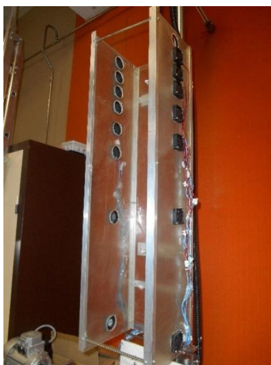
Figure 97. Arrangement of fan arrays in cooling chamber
