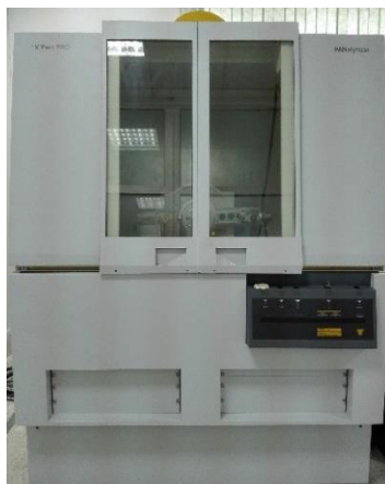
Figure 39. XRD used for analytical analysis of polymers
