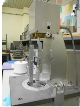
Figure 50. KES - Single hair stiffness tester
