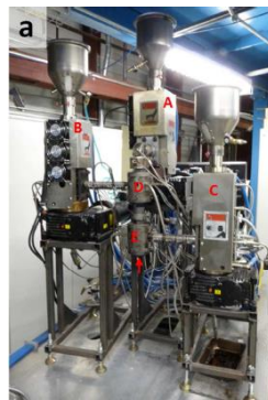
Figure 18. Melt extrusion used for the development of three layered coaxial composite filament
