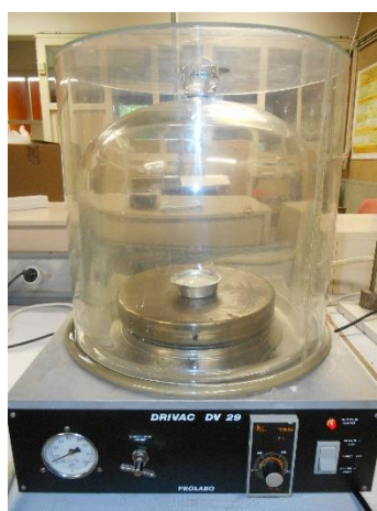
Figure 35. Desiccator for conditioning
