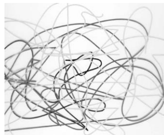
Figure 7. Diagrammatic representation of molecular chain arrangement in molten polymer
