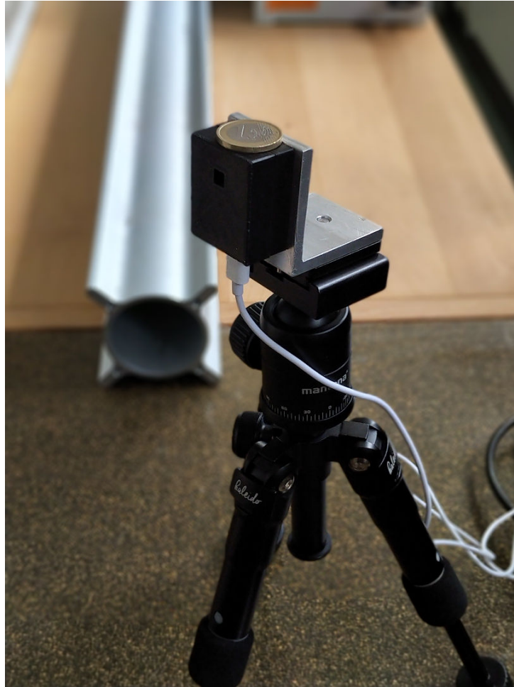
Figure 2.16: Small uncooled IR camera with 3D-printed case. A coin of 1€ is placed at the top as a scale factor.
