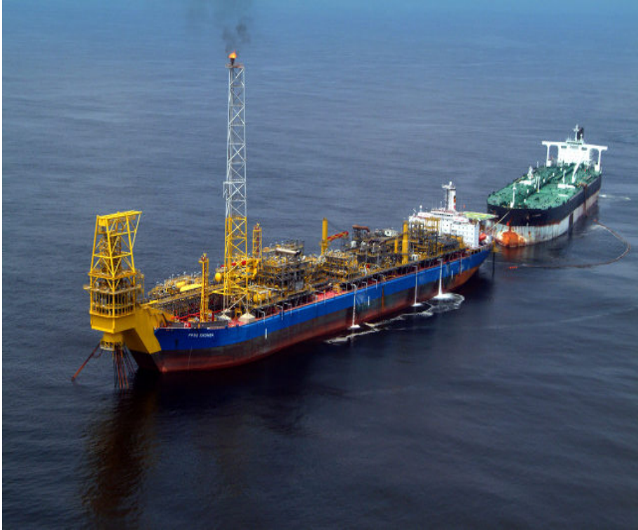
Figure 4 – Tandem offloading operation between a FPSO and a shuttle tanker 8
