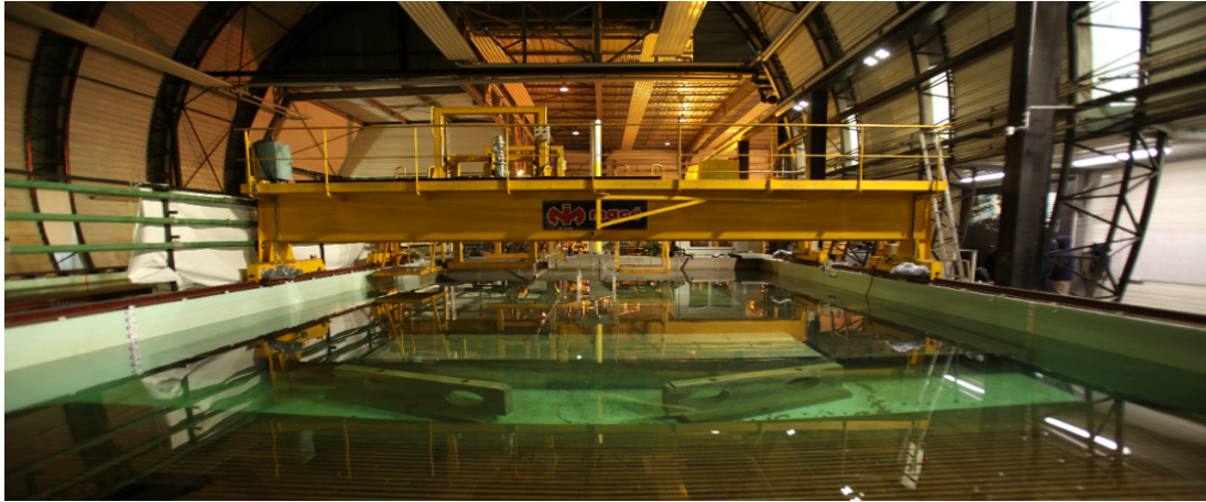
Figure VI.2 – Shallow water basin of Ecole Centrale de Nantes
