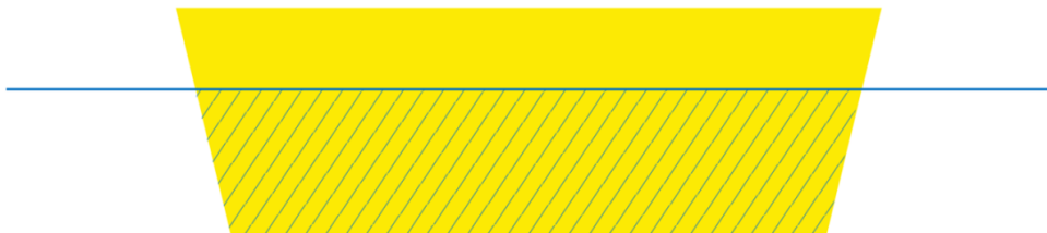
Figure III.4 – Linear model of a floating body (yellow) in waves at their mean elevation (solid blue line) and its wetted surface (hatched area)
