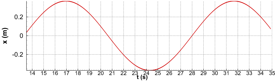
Figure III.27 – Prescribed harmonic motion of Body 2 for Case 1
