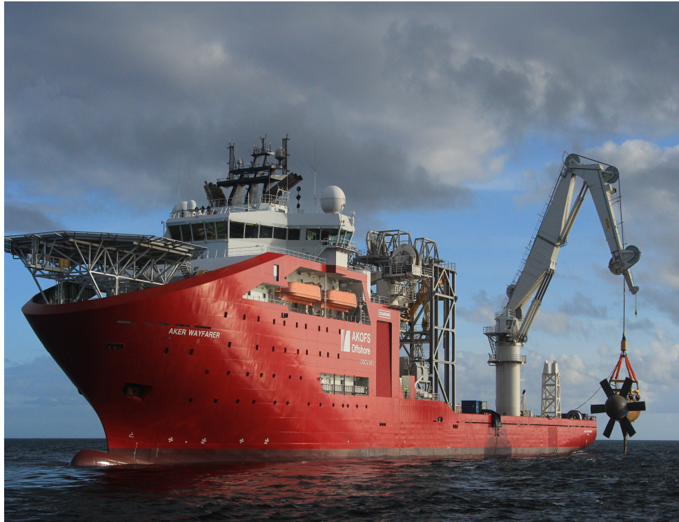
Figure 10 – Lifting operation of the Sabella D10 tidal turbine 14
