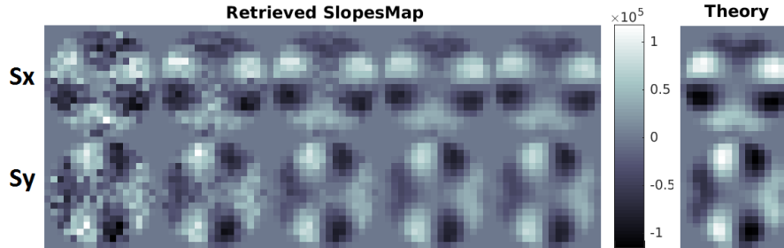
(d) Slopes Map estimation for 250,500,1000,3000 and 5000 iterations with a mode amplitude of 5 nm
