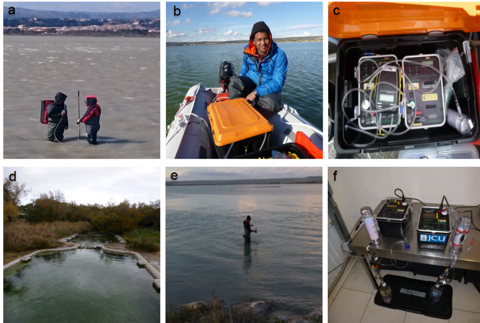
Figure 2.2| Sampling campaign in La Palme lagoon. (a) Porewater sampling using a direct-push, shielded-screen well-point piezometer, (b) radon and salinity mapping, (c) two RAD7 monitors connected in parallel, (d) karstic groundwater spring, (e) radon sampling in the lagoon with submersible pump, and (f) counting of radon samples.
