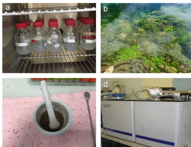
Figure 3.2 | (a) Reduction / diffusion method for measurement of the \delta^{15}\text{N} of \text{NO}_3^- and DIN, (b) macrophyte samples in karstic spring, (c) grounded macrophyte samples for stable isotope analyses and (d) stable isotope analyses on elemental analyzer mass spectrometer Integra CN Sercon.
