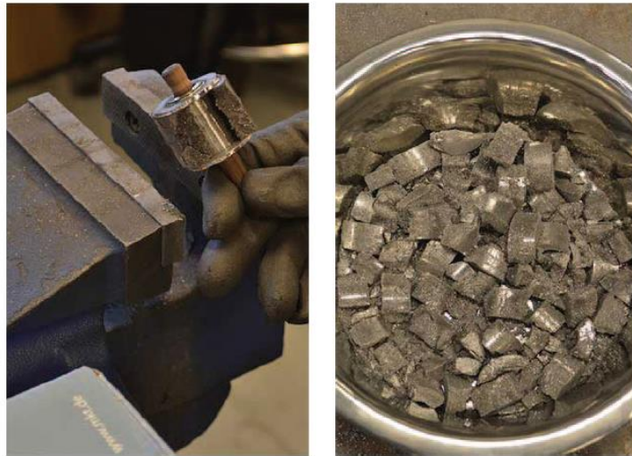
Fig. 46 Left: The cutting cross section of IP magnet for recycling; right: magnet chunk collected for further crushing process [73]
