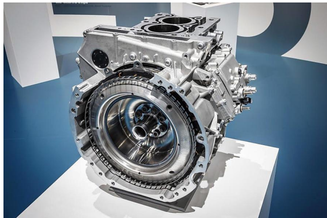
Fig. 38 A prototype of P1 mild hybrid system and its e-machine made by Mercedes [26]
