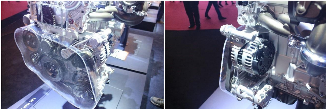
Fig. 37 A prototype of P0 belt drive system (left) and its coupled e-machine (right), filmed by author
