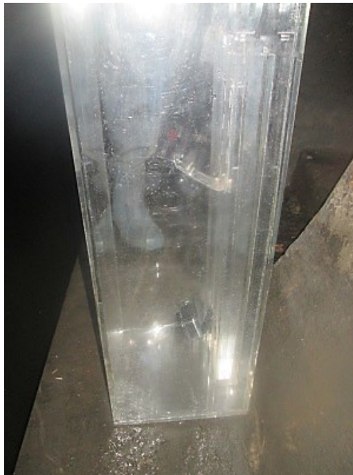
Fig. 3.18 Camera placed in a hermetic Plexiglas box to be placed inside the channel wall.
