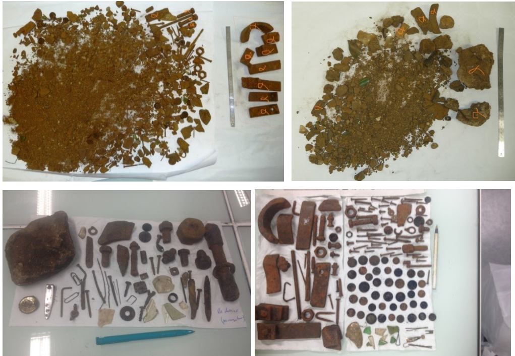
Fig. 4.1 Example of samples containing atypical particles that were finally eliminated from the samples (marked particles).
