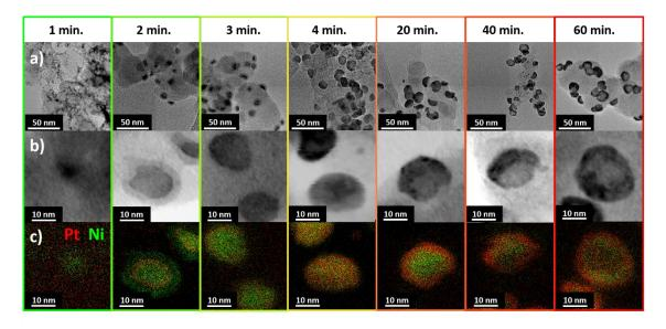
**Figure 3.1**: Time-sequenced formation and growth of hollow PtNi/C nanoparticles by electron and X-ray based techniques. (a) Conventional, (b) scanning transmission electron microscopy images and (c) X-EDS elemental maps of the different nanostructures forming during the synthesis of hollow PtNi/C NPs.
