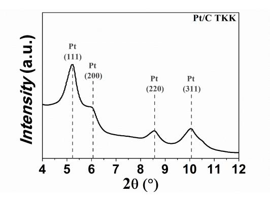
Figure A1.1: Synchrotron WAXS pattern of the reference Pt/C TKK in ex-situ configuration.
