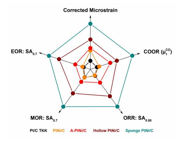
**Figure 4.14**: Spider graph summarizing the different key properties of the different electrocatalysts from this study, showing the similar trends between increasing defects content (corrected microstrain), COOR activity ( $\mu_1^{CO}$ ), ORR activity (SA measured at 0.95 V *vs.* RHE), MOR activity (SA measured at 0.7 V *vs.* RHE) and EOR activity (SA measured at 0.7 V *vs.* RHE). All SAs corrected from ohmic drop, only the SA for ORR is corrected from diffusion.
