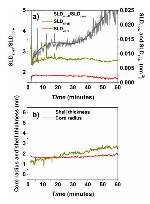
**Figure 3.5:** Morphological characterization of the different nanostructures forming the synthesis of hollow PtNi/C nanoparticles. Variation of the parameters extracted from the fitting of the SAXS data: (a) scattering light density of the core (SLD<sub>core</sub>), of the shell ((SLD<sub>shell</sub>) and their ratio, (b) core radius and shell thickness. The solid line in (a) is a  $5^{\text{th}}$  order polynomial fit of the SLD<sub>shell</sub>/SLD<sub>core</sub> ratio.
