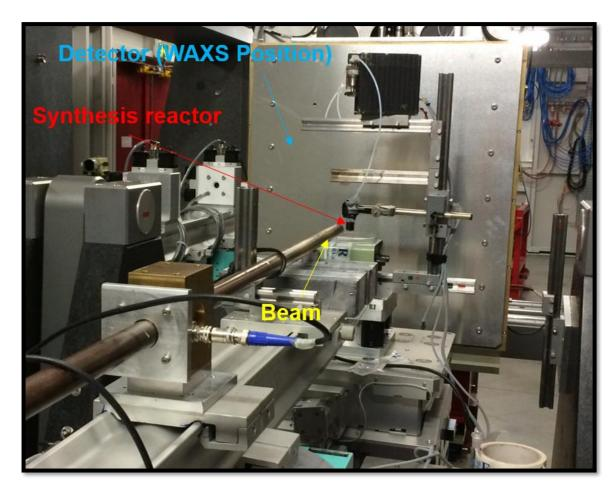
Figure A1.2: Picture of the Operando Synchrotron WAXS setup at the ID31 beamline, ESRF (November 2015).
