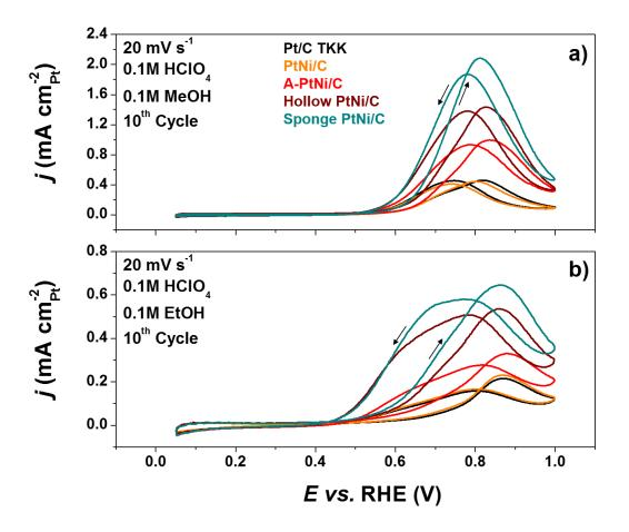
**Figure 4.13**: 10<sup>th</sup> cyclic voltammogram obtained in 0.1 M HClO<sub>4</sub> containing (a) 0.1 M methanol, (b) 0.1 M ethanol. Potential sweep rate: 20 mV s<sup>-1</sup>,  $T = 25 \pm 1$  °C and Pt loading: 20  $\mu$ gPt cm<sup>-2</sup>geo. The voltammograms were recorded after keeping the electrode potential 15 min at 0.1 V *vs*. RHE.  $T = 25 \pm 1$  °C.
