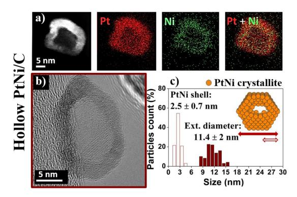
**Figure 4.2.** (a) High angle annular dark field scanning transmission electron microscopy (HAADF-STEM) image and X-EDS elemental maps, (b) TEM, particle size distribution and (c) graphical representation of hollow PtNi/C electrocatalysts. The particle size distribution was built by measuring the maximum Feret diameter of the outer metal shell and of the inner core on more than 200 isolated (*i.e.* not-agglomerated) nanoparticles.
