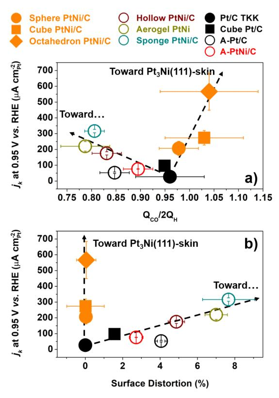
**Figure 5.18**: Relationship between the ORR specific activity measured at E = 0.95 V vs. RHE and both electrochemical (a) and physical (b) markers for the density of structural defects for the different electrocatalysts evaluated in this study.
