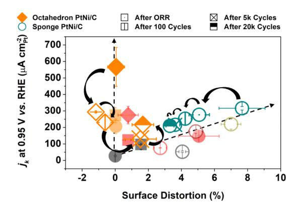
**Figure 5.31**: Relationship between the ORR specific activity measured at E=0.95 V vs. RHE and the Surface Distortion for the electrocatalysts evaluated in this section. The initial trend introduced in **Figure 5.18** is superposed for the sake of comparison. Transparent data points correspond to **Figure 5.18** and **Figure 5.26b** while opaque symbols are related to Octahedron and Sponge PtNi/C catalysts before and after potential cycling between 0.6 and 1.0 V vs. RHE at T=80 °C.
