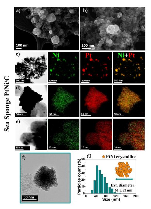
**Figure 4.3:** (a-b) SEM images; (c-e) STEM images and X-EDS elemental maps, (f) TEM; (g) particle size distribution and graphical representation of the 'sea sponge' PtNi/C electrocatalyst synthesized in this study. The particle size distribution was built by measuring the diameter of more than 200 aggregates. (b) shows the presence of opened porosities.
