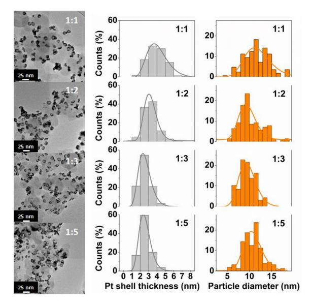
**Figure 3.6**: TEM images and histograms of the Pt-rich shell thickness and of the outer diameter of the hollow PtNi/C nanoparticles. The Pt:Ni stoichiometry in the initial metal salt precursor solution is indicated in the top right-hand side corner of individual histograms/images. From Ref. <sup>136</sup>.
