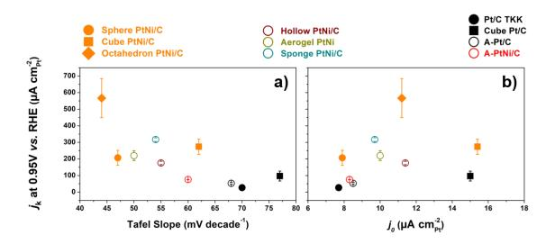
**Figure 5.14**: Relationship between the ORR specific activity measured at E=0.95 V vs. RHE and the Tafel slope (a) or the exchange current density  $j_0$  for the different electrocatalysts from this study.
