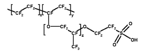
**Figure 1.11**: PFSA membrane structure. For Nafion <sup>®</sup>: x = 6-10; y = z = 1.
