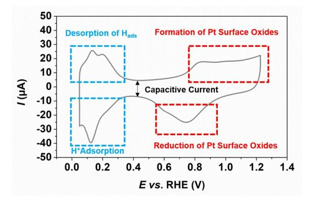
Figure A1.7: Base cyclic voltammogram recorded in Ar-saturated 0.1 M HClO<sub>4</sub> electrolyte of the Sponge PtNi/C nanoparticles at a sweep rate of 20 mV s<sup>-1</sup>. The different regions of interest are highlighted in colored squares and labelled.
