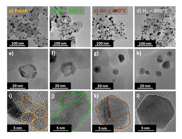
**Figure 3.10**: TEM (a-h) and HRTEM (i-l) images of the as-synthetized PtNi/C nanoparticles (a-d) and after thermal annealing at 400 °C under different gas atmospheres: (e-f). In (i-l), the boundaries between the individual PtNi nanocrystallites are highlighted in colour. From Ref. <sup>143</sup>.
