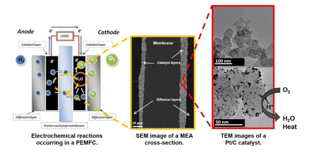
**Figure 1.9**: Components of a PEMFC single cell: schematic (left); scanning electron microscopy (SEM) image of the MEA (middle) and transmission electron microscopy (TEM) images of a commercial Pt/C catalyst (right).
