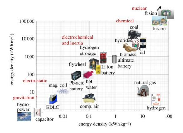
Figure 1.7: Volumetric versus gravimetric energy density of the most important energy carriers. From Ref <sup>16</sup>.
