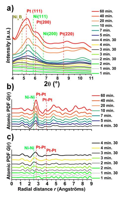
**Figure 3.4**: Structural characterization of the different nanostructures forming the synthesis of hollow PtNi/C nanoparticles. (a) High-energy WAXS patterns (the vertical dashed lines indicate the reflections of pure metallic Pt and Ni), (b, c) experimental atomic pair distribution functions.
