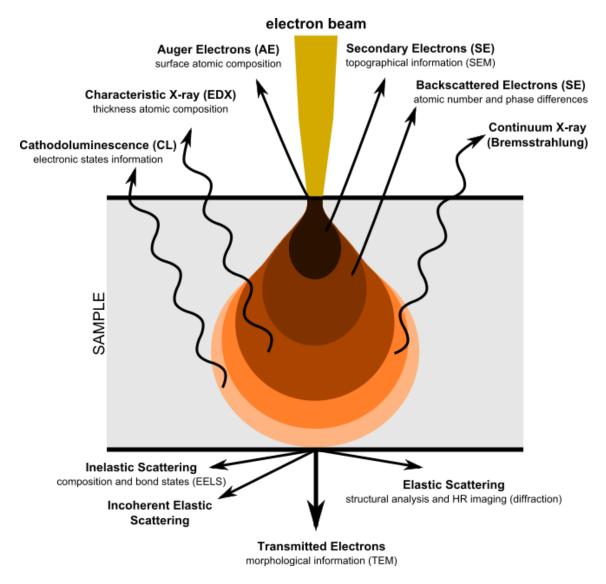
**Figure A1.9**: Diagram illustrating the phenomena resulting from the interaction of highly energy electrons with matter. From Ref <sup>247</sup>.
