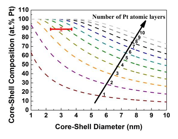
**Figure 4.5**: Relation between the chemical composition and the diameter of the core@shell nanoparticles established from the model of Montejano-Carrizales et al.  $^{167,168}$ . The red symbol is the intersection of the composition of the coreshell catalyst measured by X-EDS and the particle size measured by TEM. According to the model, the Ni@Pt/C catalyst features a 4.5 ± 1 layers thick Pt shell.
