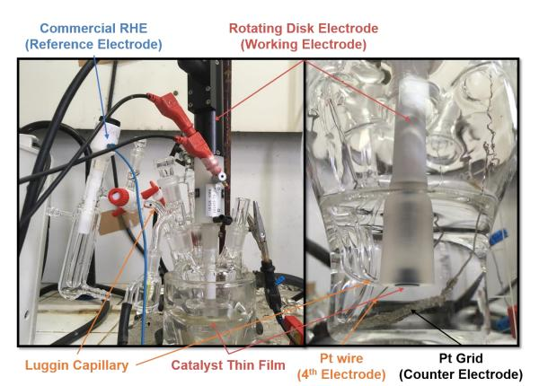
Figure A1.6: Pictures of the electrochemical four-electrode setup used in this manuscript.
