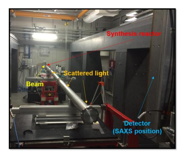
Figure A1.3: Picture of the Operando Synchrotron SAXS setup at the ID31 beamline, ESRF (November 2015).
