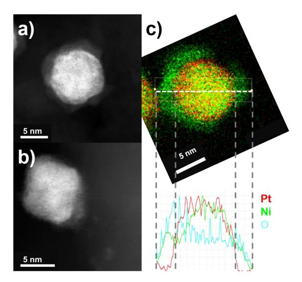
**Figure 5.4**: Evidence of a Ni oxides phase. HRSTEM-HAADF images of (a) Sphere PtNi/C; (b) Octahedron PtNi/C showing the presence of a lighter (than PtNi) phase on the surface of the nanoparticles composing these samples. (c) X-EDS elemental map and linear scan crossing a spherical PtNi nanoparticle, the extra surface phase is composed of Ni and O.
