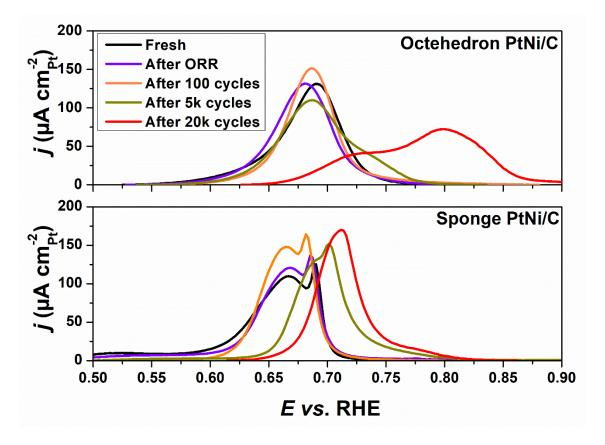
**Figure 5.28**: CO<sub>ads</sub> stripping voltammograms recorded under Ar-saturated 0.1 M HClO<sub>4</sub> electrolyte at v = 20 mV s<sup>-1</sup> for the Octahedron and Sponge PtNi/C before and after two consecutive ORR electrochemical characterizations and a different number of potential cycles.
