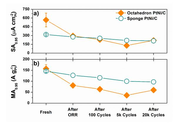
**Figure 5.27**: Variations of the specific (a) and the mass (b) activity for the ORR measured at E= 0.95 V vs. RHE for both Octahedron and Sponge PtNi/C electrocatalysts, before and after potential cycling between 0.6 and 1.0 V vs. RHE at T = 80 °C. The ORR activities were determined after correction for Ohmic losses and mass-transport in O<sub>2</sub>-saturated 0.1 M HClO<sub>4</sub> at a potential sweep rate of 5 mV s<sup>-1</sup> and a revolution rate of  $\omega$  = 1600 rpm
