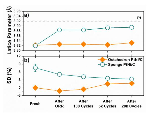
**Figure 5.30**: Evolution of the lattice parameter (a) and Surface Distortion (b) for both Octahedron and Sponge PtNi/C electrocatalysts, before and after a various amount of 50 mV s<sup>-1</sup> potential cycles between 0.6 and 1.0 V vs. RHE at T= 80 °C.
