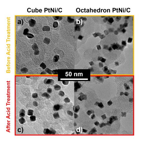
Figure 5.21: TEM images of the facetted nanoparticles (Cube PtNi/C and Octahedron PtNi/C) before and after acidic treatment, showing an overall conservation of the particle shape.
