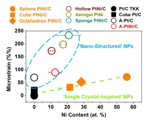
**Figure 5.5**: Microstrain *vs*. Ni content for the electrocatalysts evaluated in this study. The plot shows an almost linear variation for the'single crystal' inspire nanoparticles, indicating a contribution of Ni atoms to the microstrain. The cyan star symbol represents the theoretical position of an isolated monocrystalline PtNi nanoparticle featuring 15 at. % Ni, based on the microstrain-Ni content relationship revealed by this plot.
