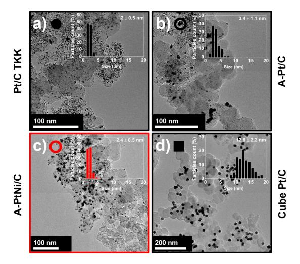
**Figure 5.2**: TEM images, associated symbol and particle size distributions of the reference catalysts of this study (a) Pt/C TKK; (b) A-Pt/C; (c) A-PtNi/C and (d) Cube Pt/C.
