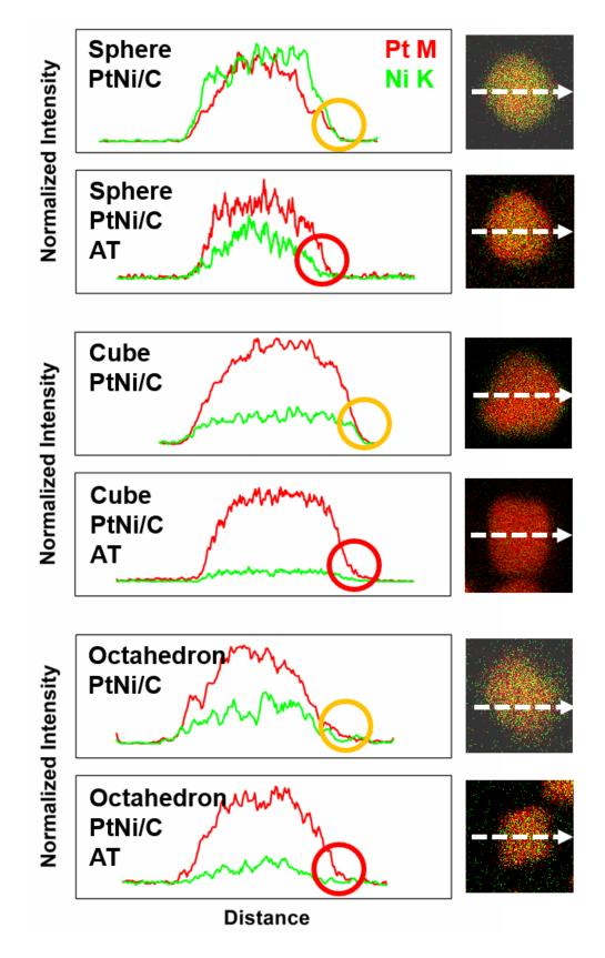
**Figure 5.19**: STEM-X-EDS compositional line profiles and elemental maps of the 'single crystal inspired' samples before and after acidic treatment in  $1M H_2SO_4$ . The STEM-X-EDS profiles are normalized to the elemental scattering factors, allowing a direct reading of the thickness -projected composition through the intensity ratios. The circles highlight the surface Pt:Ni stoichiometry changes during the acidic treatments.
