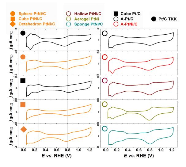
**Figure 5.15**: Base voltammograms measured on the electrocatalysts evaluated in this Chapter. The measurements were conducted in Ar-saturated 0.1 M HClO<sub>4</sub> at a potential sweep rate of 20 mV s<sup>-1</sup>. The currents were normalized by the ECSA measured *via*  $CO_{ads}$  stripping experiments.
