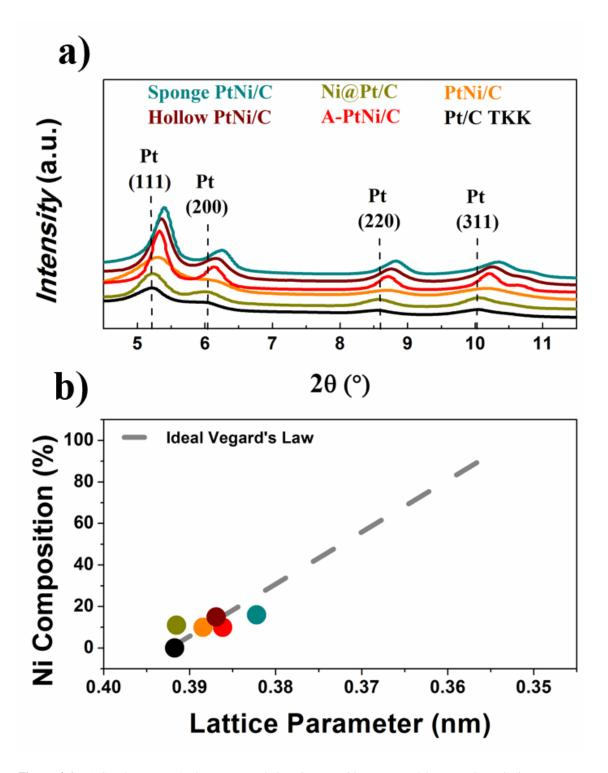
**Figure 4.6**: (a) Synchrotron WAXS patterns and (b) Ni composition measured by X-EDS *vs.* lattice parameter calculated from Rietveld refinement of the WAXS patterns for the synthetized bimetallic catalysts and of the reference Pt/C TKK material. The chemical composition predicted by the Vegard's law is represented as a dotted line in (b).
