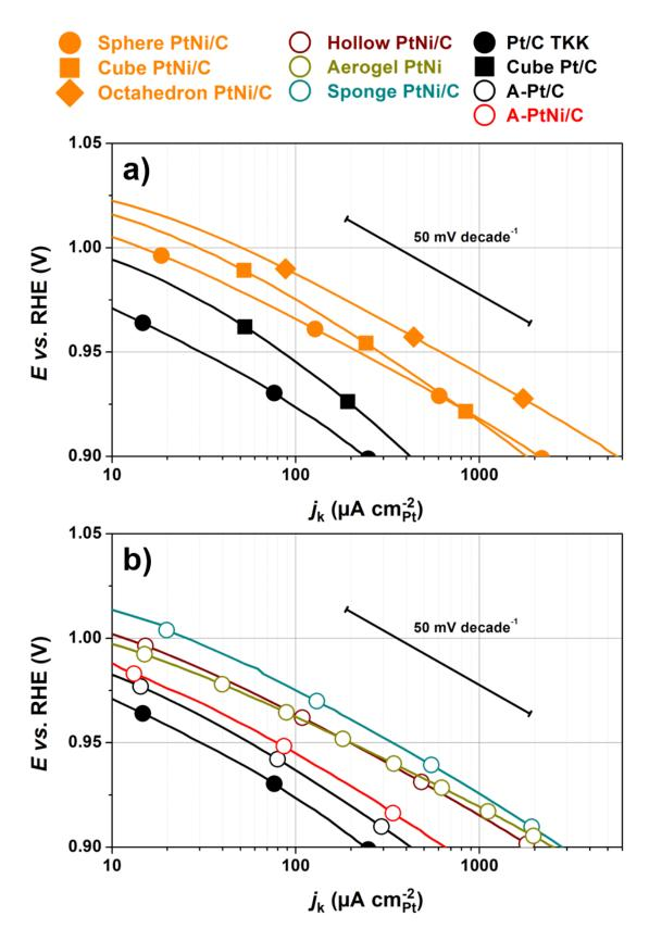
**Figure 5.12**: Tafel plots obtained from the steady-state I-E curves measured at  $\omega = 1600$  rpm after correction for ohmic losses and diffusion in O<sub>2</sub>-saturated 0.1 M HClO<sub>4</sub> at a potential sweep rate of 5 mV s<sup>-1</sup>.
