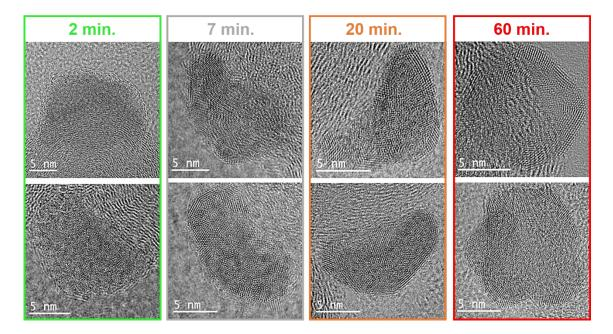
Figure 3.2: HRTEM images of the different nanostructures forming during the synthesis of hollow PtNi/C nanoparticles.
