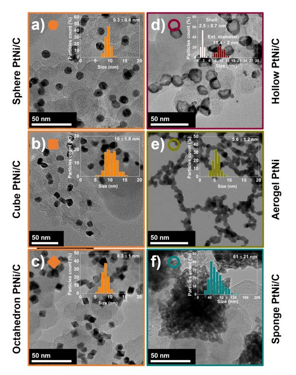
**Figure 5.1:** TEM images, associated symbol and particle size distributions of the main catalysts of this study (a) Sphere PtNi/C; (b) Cube PtNi/C; (c) Octahedron PtNi/C; (d) Hollow PtNi/C; (e) Aerogel PtNi and (f) Sponge PtNi/C.
