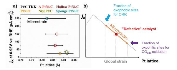
**Figure 4.11**: (a) Relationship between the ORR specific activity measured at E = 0.95 V vs. RHE and the Pt lattice parameter for the different electrocatalysts from this study. According to its definition, the microstrain is used as the error bar for the Pt lattice determination from Rietveld refinement of WAXS patterns; (b) schematic explaining the role of microstrain (compared to global strain) for both COOR and ORR in the admitted ORR activity-Pt lattice volcano plot.
