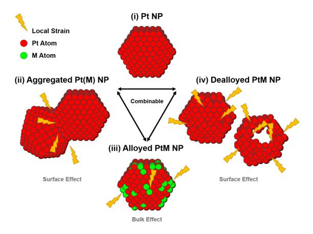
**Figure 5.6**: Possible sources of microstrain in bimetallic PtM nanoparticles (NPs). While slight or no microstrain can be found in monocrystalline pure Pt NPs, (i) the value of microstrain can rise due to NP aggregation in the presence of grain boundaries, (ii) inhomogeneous PtM alloy solution, (iii) catalysts produced by dealloying (iv). Unlike aggregation and dealloying which occur on the surface of the crystallites, inhomogeneous PtM solid solution affects the whole nanoparticle bulk.
