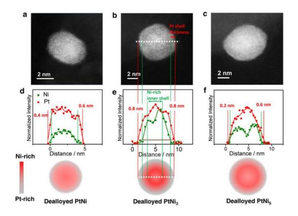
**Figure 2.7**: High resolution HAADF-STEM images of dealloyed PtNi (a),  $PtNi_3$  (b) and  $PtNi_5$  NPs (c), and EELS line compositional profiles (d– f) across the NPs, respectively. From Reference <sup>89</sup>.
