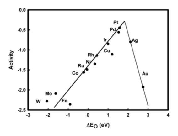
**Figure 2.1**: Trend in calculated oxygen reduction activity (arbitrary units) plotted as a function of the calculated oxygen binding energy for different metals. From Ref. <sup>45</sup>
