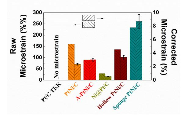
Figure 4.7. Values of raw microstrain (left scale) and microstrain corrected from surface effect ('Corrected Microstrain', see right scale) for the catalysts evaluated in this study.
