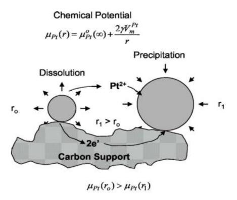
**Figure 1.16**: Ostwald ripening: dissolution of small particle with higher chemical potential, and precipitation on the larger ones. Cations transport occurs in liquid phase while electrons are transported by the conductive catalyst support (here carbon). From Reference <sup>54</sup>.
