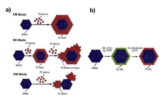
**Figure 2.6**: (a): schematic illustration of three different growth modes; (b): Schematic illustration of the synthesis of Pt mono-layer (ML) on metal nanoparticles using UPD followed by a redox replacement reaction. From Reference <sup>87</sup>.
