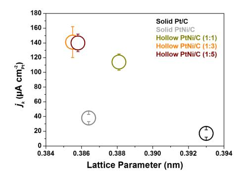
**Figure 3.9**: ORR kinetic current measured at E = 0.95 V vs. RHE vs. lattice parameter for the different electrocatalysts investigated in Ref. <sup>136</sup>. The measurements were conducted in O<sub>2</sub>-saturated 0.1 M HClO<sub>4</sub> at a potential sweep rate v = 0.005 V s<sup>-1</sup>. Other conditions:  $T = 25 \pm 1$  °C, Pt loading = 8.0 µg. Lattice parameter extracted from XRD patterns.
