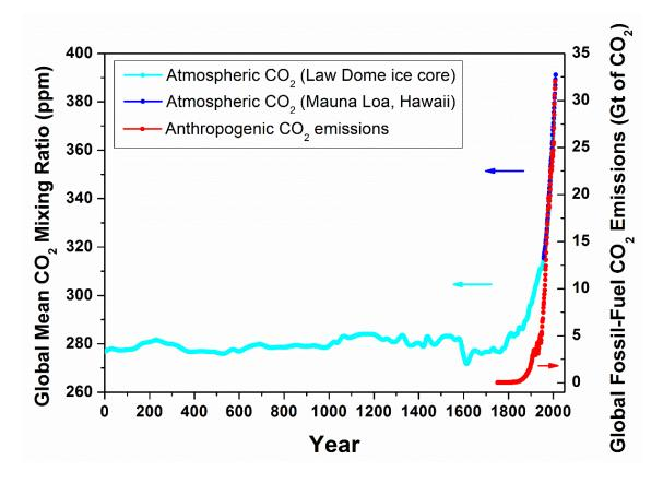
**Figure 1.2**: Correlation between increasing global CO<sub>2</sub> concentration in the atmosphere (from Law Dome ice core analysis <sup>3</sup> plotted in cyan, followed by direct atmospheric measurement in Mauna Loa, Hawaii <sup>4</sup> plotted in blue) and the anthropogenic CO<sub>2</sub> emissions from fossil fuel combustion estimates <sup>5</sup> plotted in red).
