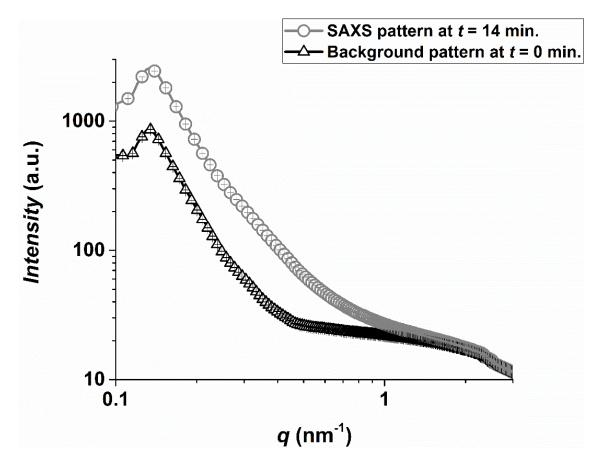
**Figure A1.4**: Measured SAXS pattern at t = 0 min and t = 14 min. Black curve: the last SAXS pattern taken before the beginning of the synthesis, which was used as a background. Grey curve: the SAXS curve measured at t = 14 min before the background subtraction. The error bar is the standard deviation
