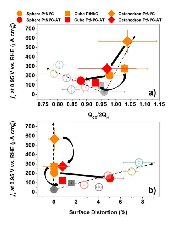
**Figure 5.26**: Relationship between the ORR specific activity measured at E= 0.95 V vs. RHE and both electrochemical (a) and physical (b) markers for the electrocatalysts evaluated in this section. The initial trend introduced in **Figure 5.18** is superposed for the sake of comparison. Transparent data points correspond to **Figure 5.18** while opaque symbols are related to the 'single crystal inspired' catalysts before (orange) and after (red) acidic treatment.
