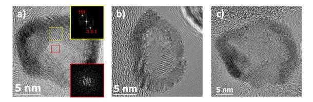
**Figure 3.7**: HRTEM images of hollow PtNi/C nanoparticles (initial Pt:Ni stoichiometry of 1:3). The FT patterns taken in different zones and showed in insert of picture (a) and confirm the presence of nanopores > 1 nm. From Ref. <sup>136</sup>.
