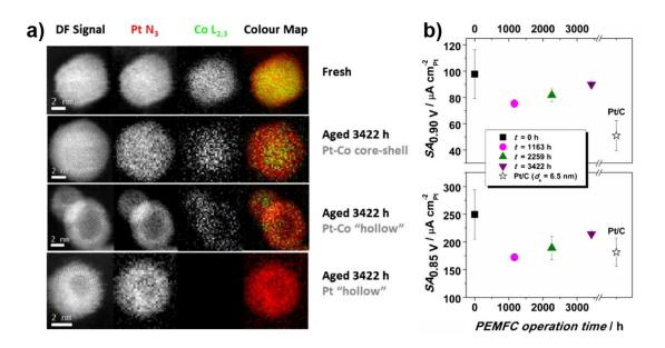
**Figure 2.9**: (a) HAADF-STEM and EELS elemental maps of a Pt<sub>3</sub>Co catalyst before and after aging under PEMFC system, and (b) SA *vs.* cycling time of this Pt<sub>3</sub>Co catalyst in comparison with a commercial Pt/C. Adapted from Ref <sup>67</sup>.
