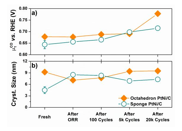
**Figure 5.29**: Variation of both  $\mu_1^{CO}$  (a) and crystallite sze (b) for both Octahedron and Sponge PtNi/C electrocatalysts, before and after potential cycling between 0.6 and 1.0 V *vs.* RHE at T = 80 °C.
