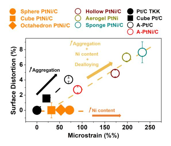
**Figure 5.8**: Surface distortion *vs.* microstrain for the different electrocatalysts used in this study. After deconvolution from the Ni contribution and crystallite size, it may be observed that high microstrain values do not necessarily imply surface distortion (this strongly depends on the structure and the chemical composition of the electrocatalysts).
