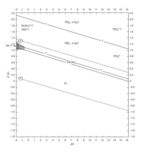
Figure 1.15: Pourbaix diagram of Platinum in water at 25°C. E (V vs. RHE) vs. pH
