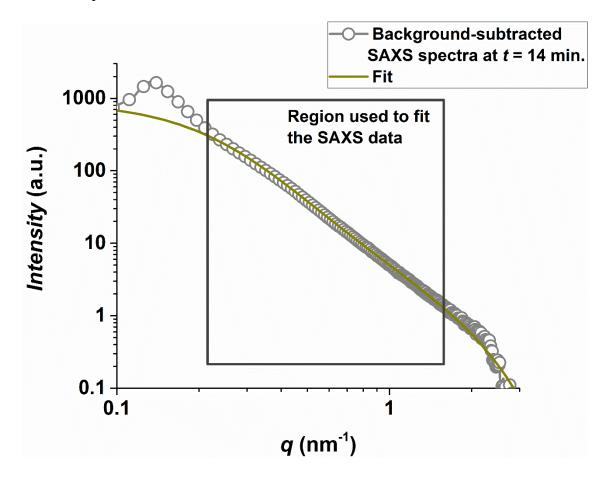
Figure A1.5: Example of a fit of SAXS pattern. Grey squares: the background-corrected SAXS pattern at t = 14 min. Dark yellow curve: the fit using the core/shell NP model described in the main text.
