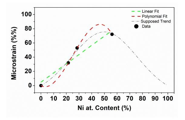
**Figure 5.7**: Possible descriptions of the effect of the Ni at. % on the value of microstrain. Both the linear and the polynomial fit give reasonable agreement but the polynomial fit was chosen as it naturally suggests the existence a maximal Ni contribution to the microstrain (around 50 at. %, supposed trend), which makes physical sense.
