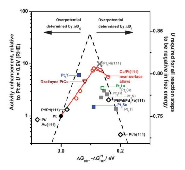
**Figure 2.2:** Volcano plot showing the rate of the oxygen reduction reaction on Pt-based alloys as a function of the calculated oxygen adsorption energy relative to Pt. From Ref. <sup>69</sup>.
