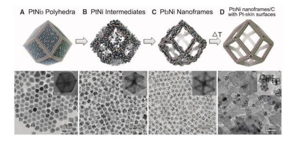
**Figure 2.11**: Schematic illustrations and corresponding TEM images of the samples obtained at four representative stages during the evolution process from polyhedra to nanoframes. Initial  $PtNi_3$  polyhedra (a); PtNI intermediates (b); final hollow  $Pt_3Ni$  nanoframes with Pt(111)-skin-like surface dispersed on high surface carbon. From Ref. <sup>125</sup>.
