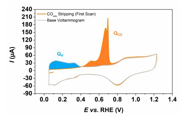
**Figure A1.7**: CO<sub>ads</sub> stripping cyclic voltammograms recorded in Ar-saturated 0.1 M HClO<sub>4</sub> electrolyte of the Sponge PtNi/C nanoparticles at a sweep rate of 20 mV s<sup>-1</sup>. The different regions of interest are highlighted and labelled.
