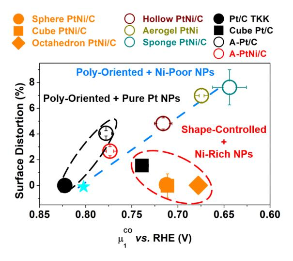
**Figure 5.11**: Surface Distortion *vs.*  $\mu_1^{CO}$  for the electrocatalysts evaluated in this study. As the SD does not take account the bulk Ni content, this plot allows isolating the contribution from the surface disorder. The cyan star symbol represents the theoretical position of an isolated monocrystalline 15 at. % Ni PtNi nanoparticle based on the theoretical value of  $\mu_1^{CO}$  extracted from **Figure 5.10**.
