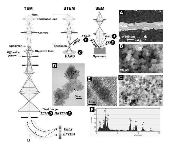
**Figure A1.10**: Scheme of SEM and TEM with examples of images of MEA in (a) SEM in BSE mode, (b) FEG-SEM in SE mode, (c) FEG-SEM-STEM of an ultramicrotomed MEA cross-section, (d) TEM and (e) HRTEM; (f) X-EDS microanalyses. From Ref. <sup>248</sup>.
