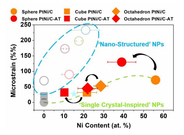
**Figure 5.20**: Microstrain *vs*. Ni content for the electrocatalysts evaluated in this section superposed on the initial trend introduced **Figure 5.5**. Transparent data points correspond to **Figure 5.5**, while opaque symbols are related to the 'single crystal inspired' catalysts before (orange) and after (red) acidic treatment. The green dashed line corresponds to the microstrain-Ni at. % relationship as fitted **Figure 5.7** and considered in this study.
