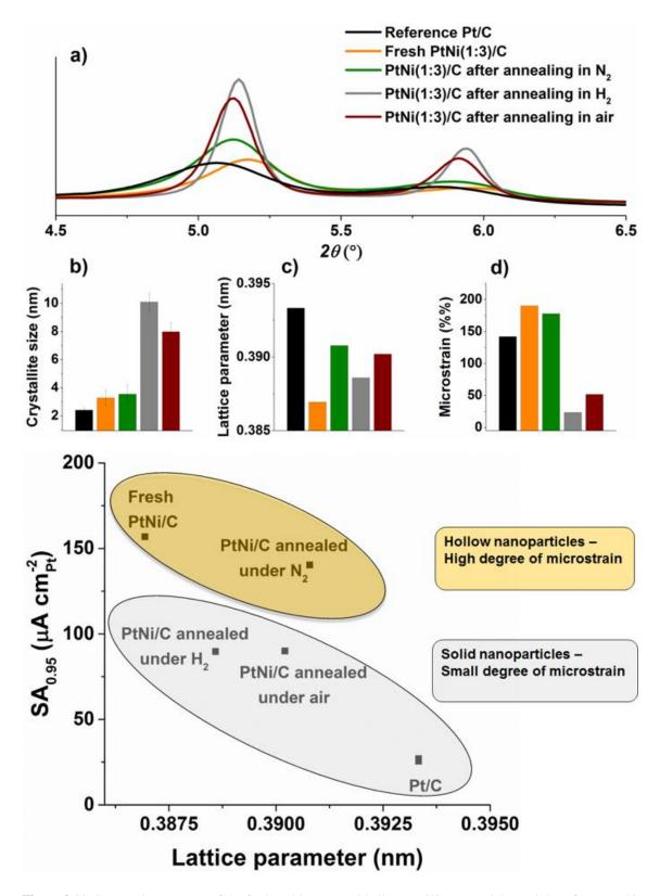
**Figure 3.11**: Structural parameters of the fresh and heat-treated hollow PtNi/C nanoparticles and the reference Pt/C material used in this study: (a) synchrotron XRD patterns; (b) average crystallite size; (c) lattice parameter; (d) microstrain estimated by Rietveld analysis of the WAXS patterns, and (e) ORR specific activity measured at 0.95 V *vs.* RHE compared with the lattice parameter for the different electrocatalysts. Adapted from Ref. <sup>143</sup>.
