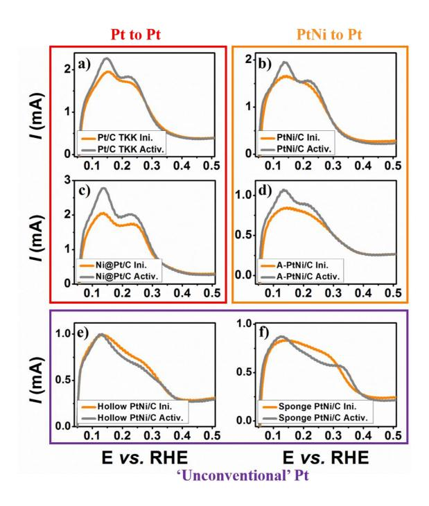
**Figure 4.8.** Comparison of the H<sub>upd</sub> desorption region before (1<sup>st</sup> scan) and after (50<sup>th</sup> scan) electrochemical activation for (a) the reference Pt/C TKK, (b) PtNi/C, (c) Ni@Pt/C, (d) A-PtNi/C, (e) hollow PtNi/C, and (f) 'sea-sponge' PtNi/C (f) catalysts. Ar-saturated 0.1 M HClO<sub>4</sub>;  $\nu = 500$  mV s<sup>-1</sup>;  $T = 25 \pm 1$  °C; no rotation of the electrode; Pt loading: 20 µgPt cm<sup>-2</sup><sub>ge0</sub>.
