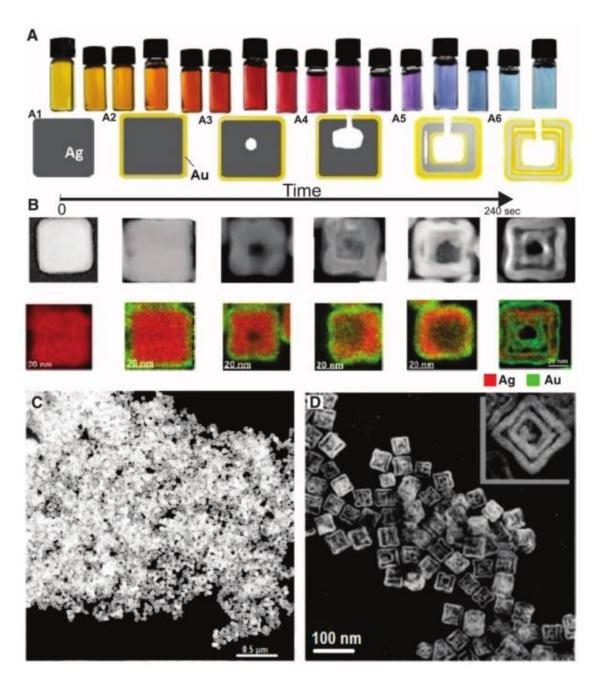
**Figure 2.10**: Optical and morphological evolution of AuAg double-walled nanoboxes (a); HAADF- STEM images and X-EDS maps for the different stages of evolution indicated in (a) (b); TEM images of AuAg double-walled nanoboxes, showing large yield production and the double-walled morphology. From Ref. <sup>113</sup>.
