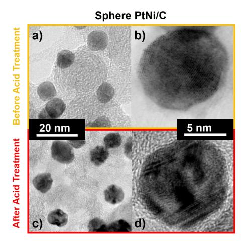
**Figure 5.22**: TEM (a, c) and HRTEM (b, d) images of the Sphere PtNi/C nanoparticles before and after acidic treatment showing the apparition of porosity.
