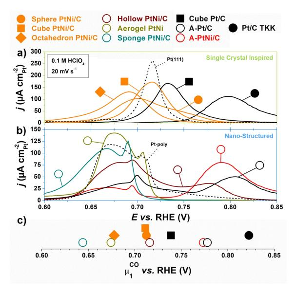
**Figure 5.9**: Background-subtracted CO<sub>ads</sub> stripping voltammograms recorded in Ar-dearated 0.1 M HClO<sub>4</sub> electrolyte at a potential sweep rate of 20 mV s<sup>-1</sup> on (a) 'single crystal' inspired and (b) 'nanostructured' electrocatalysts evaluated in this study. Dotted lines represent CO<sub>ads</sub> stripping of extended Pt surfaces, Pt(111) in (a) and Pt-poly in (b). (c) Position of the average  $\mu_1^{CO}$  for each catalyst.
