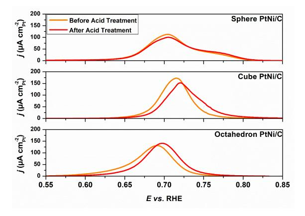
**Figure 5.23**: CO<sub>ads</sub> stripping voltammograms recorded under Ar-saturated 0.1 M HClO<sub>4</sub> electrolyte at v = 20 mV s<sup>-1</sup> for the 'single crystal inspired' electrocatalysts before and after acidic treatment.
