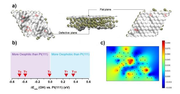
**Figure 4.12**: (a) views of the two surfaces formed on 5-layer Pt(111) slab after introduction of 40% atomic vacancies and relaxation using the VASP code; (b) OH adsorption energies relative to Pt(111) for selected catalytic sites and (c) map of the inner deformation of the surface. In b) purple and blue regions on the plot show the more oxophobic and less oxophobic catalytic sites than Pt(111) respectively. Adapted from <sup>197</sup>.
