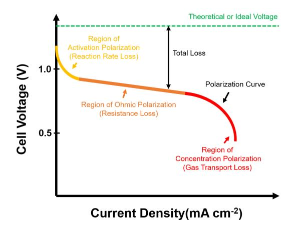
Figure 1.10: Ideal and practical fuel cell I-V (voltage vs. current) characteristics.
