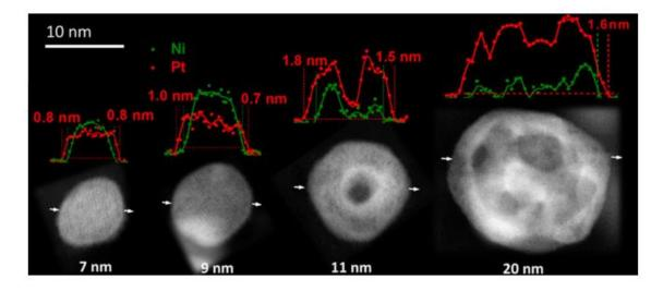
**Figure 2.8:** HAADF-STEM images and the corresponded EELS line-scan profiles of NPs with different sizes in airdealloyed PtNi<sub>3</sub> catalyst after 10,000 cycles of stability test between 0.6 and 1 V vs. RHE. Particles larger than *ca*. 10 nm steadily showed the formation of nanoporosity and, consequently lower Ni content as well as larger Pt shell thickness after the accelerated stress test. From <sup>94</sup>.
