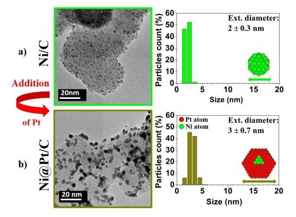
**Figure 4.4:** TEM images, particle size distributions and graphical representations (insert) of the (a) Ni/C template and (b) Ni-core@Pt-shell/C nanoparticles prepared *via* two sequential polyol syntheses. The particle size distributions of each catalyst were built by measuring the diameter of more than 200 isolated (*i.e.* not-agglomerated) nanoparticles.
