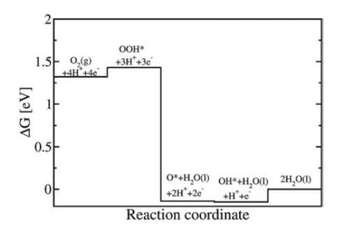
**Figure 1.14**: Free energy diagram for the 4 ORR 'direct pathway' steps at 0.9 V *vs.* RHE on Pt(111). The overall reaction decreases in free energy, but 1<sup>st</sup> and 4<sup>th</sup> steps show positive free energy changes. From Ref. <sup>46</sup>.
