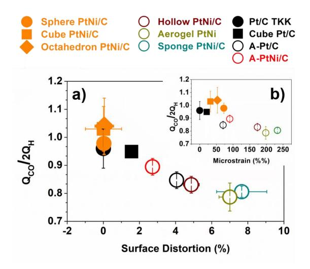
**Figure 5.17**: Surface disorder determined *via* the  $Q_{CO}/2Q_H$  ratio *vs.* structural disorder derived from XRD via the Microstrain, with correction from the Ni content and crystallite size 'Surface Distortion' (a); and without correction (b).
