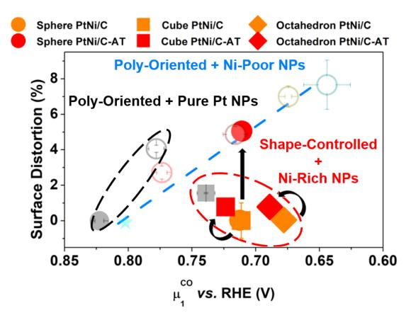
**Figure 5.25**: Surface Distortion *vs.*  $\mu_1^{CO}$  for the electrocatalysts evaluated in this section. The initial trend introduced in **Figure 5.10** is superposed for the sake of comparison. Transparent data points correspond to **Figure 5.10** while opaque symbols are related to the 'single crystal inspired' catalysts before (orange) and after (red) acidic treatment.
