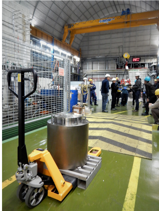
Figure 2.14: The tungsten alloy shield at LNGS during a source handling test.
