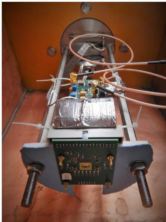
Figure 11.1: The detector on its mounting structure. The detector board is screwed onto a plastic plate that is attached to two rods, which are fixed on the flange in the back. Between the detector board and the plastic is a thermally conductive pad to improve the passive cooling of the detector. Behind the detector board is the bias board. Both are connected with a shielded flat cable. The detector voltage, the ASIC voltage and the digital communication are sent through the two feedthroughs in the flange in the back. The analog pulse heights are sent through the two coaxial cables that connect to another feedthrough on the right (not pictured).
