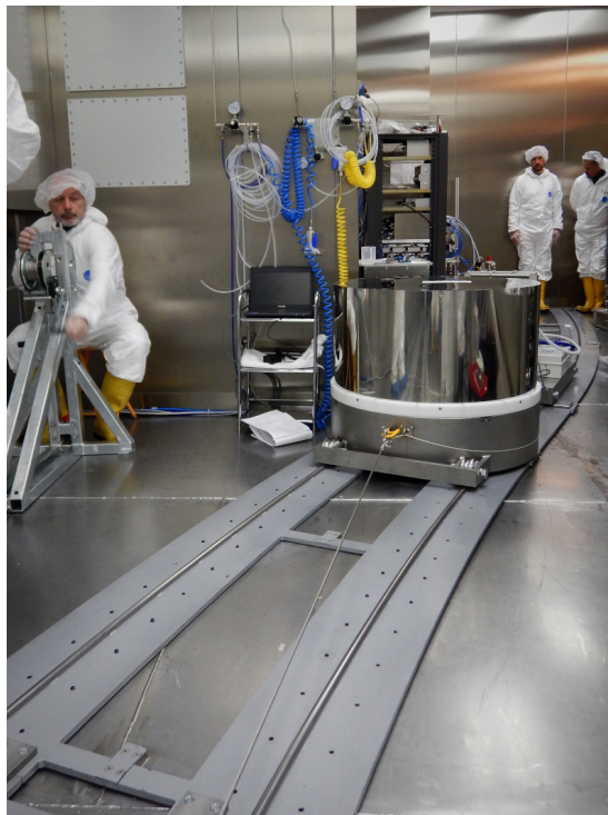
Figure 6.1: The calorimeter is moved into the pit without the vacuum chamber lid, but a protective cover during the ISPRA test (see section 5.4.1). To ensure that the source and the calorimeter are not damaged by the humidity in the pit, dried air is pumped in.
