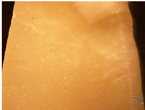
Figure V-5 Example of surface dirtiness and rugosity after use of a teflon spray
