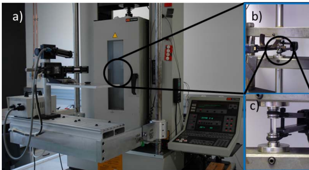
Figure V-7 a) Uniaxial tensile machine b) Uniaxial sample positioned in the machine with longitudinal and axial extensometers c) uniaxial sample (transparent polymer) with longitudinal extensometer
