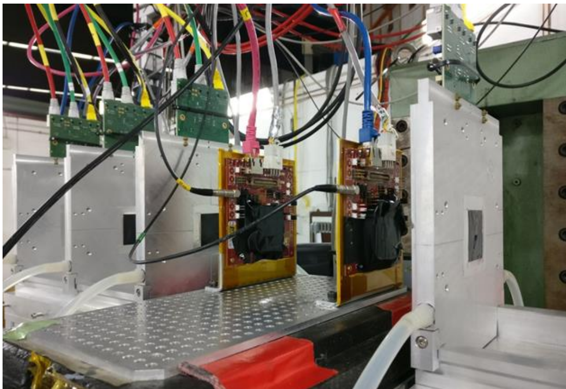
Figure 6.4 – A picture of EUDET telescope. The two DUTs and telescope planes enclosed in aluminum frames are shown. The attached rubber tubes are used for pumping cooling water through the frames. On top of the frames one can see the readout boards. At the bottom an aluminum board with a grid of M5 threaded holes with 1 \text{ cm} pitch is provided for mounting the DUTs by using L-shaped metallic holders.
