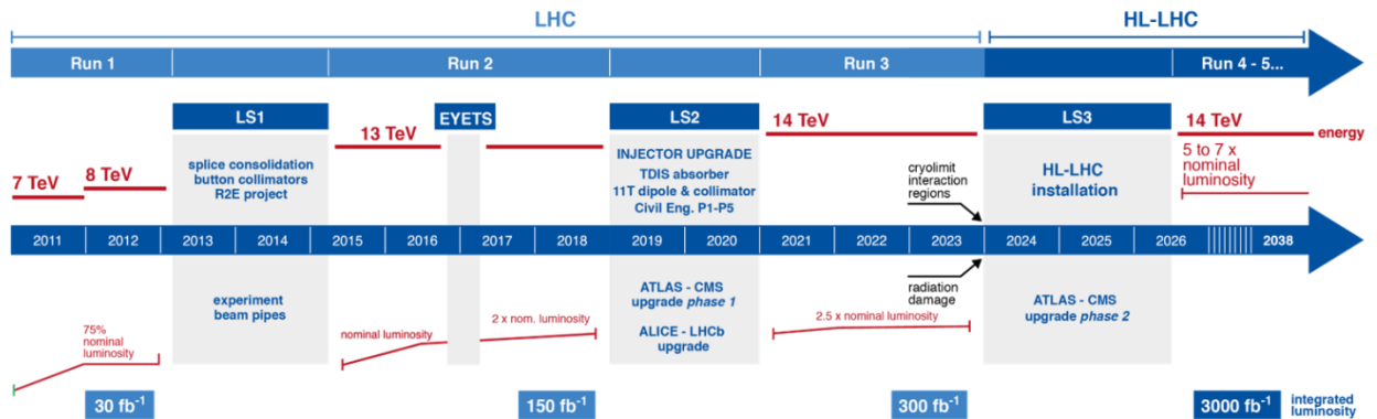
Figure 3.1 – The LHC baseline plan for the upcoming decade in terms of collision energy (upper line) and luminosity (lower lines). [50]
