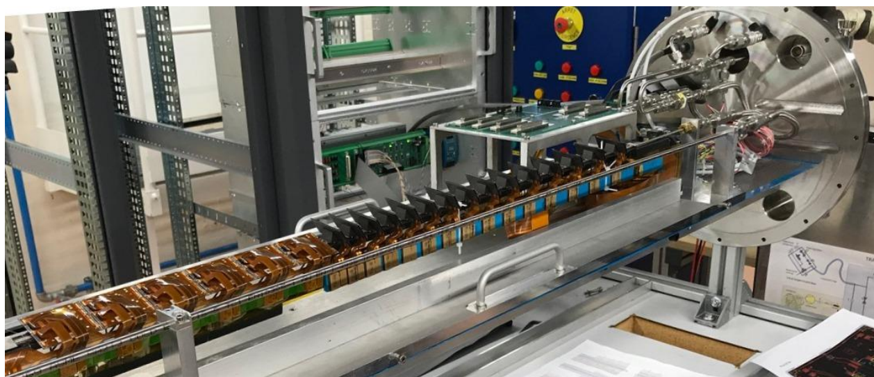
Figure 3.18 – Picture of the long thermal demonstrator with the thermal doublet heater modules assembled in the Paris cluster and installed in the inclined section.
