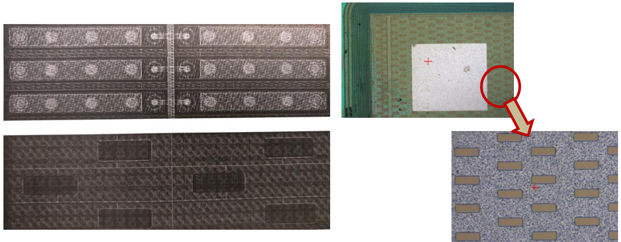
Figure 8.2 – The sensor design with openings in backside metallization. The aluminum layer, which can prevent almost completely the infrared photons penetration through the bulk, is partially removed. Each pixel has a rectangular opening as shown on the left picture.
