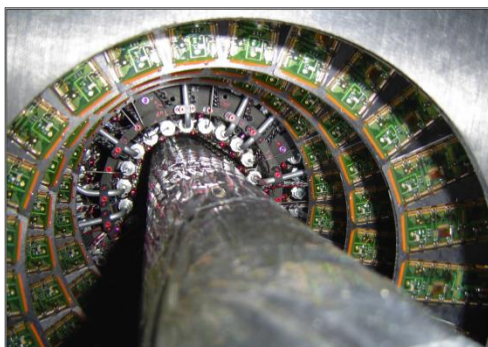
Figure 3.2 - (a) Photograph of the ATLAS pixel layers and the beam pipe before the IBL insertion.
