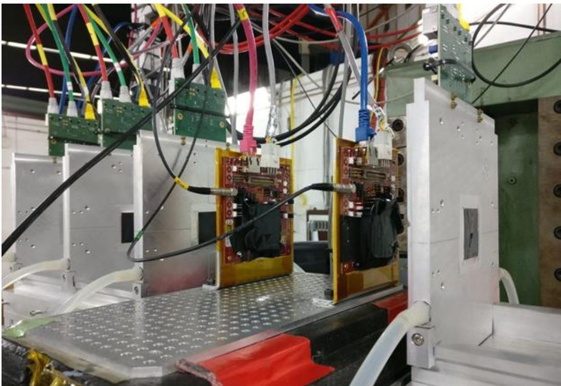
Figure 6.4 – A picture of EUDET telescope. The two DUTs and telescope planes enclosed in aluminum frames are shown. The attached rubber tubes are used for pumping cooling water through the frames. On top of the frames one can see the readout boards. At the bottom an aluminum board with a grid of M5 threaded holes with 1 \text{ cm} pitch is provided for mounting the DUTs by using L-shaped metallic holders.
