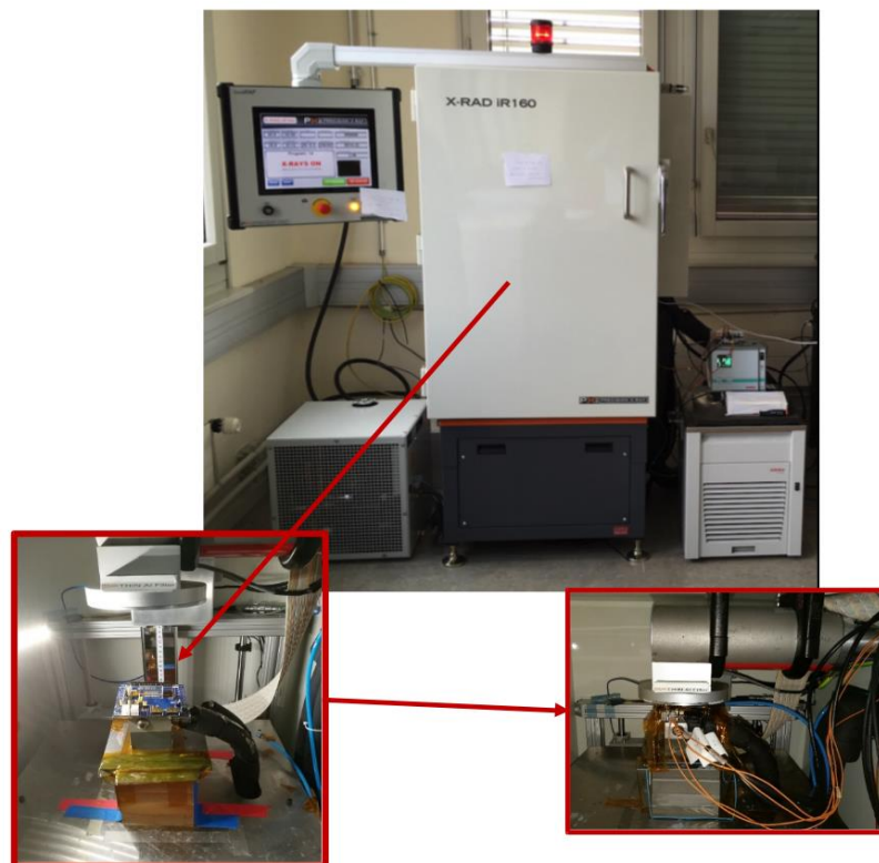
Figure 7.16 – X-RAD iR160 machine for cell irradiation and biological research.
