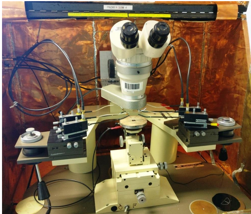
Figure 5.18 – The probe station set-up used for four probes method measurements.
