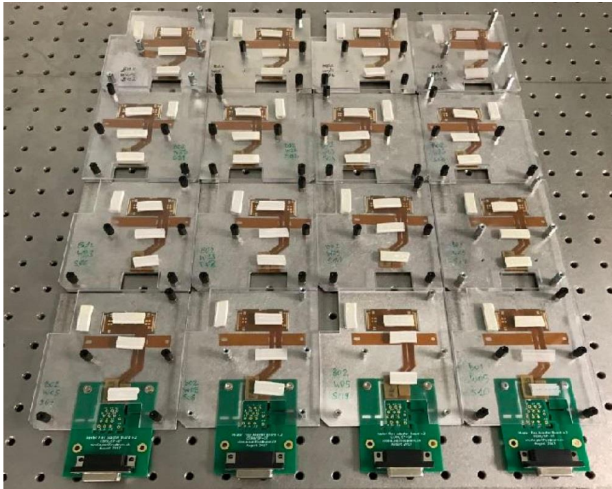
Figure 3.16 – The assemblies in the transport boxes. In the bottom line the assemblies are connected to the card to read-out used during the calibration in the climate chamber.
