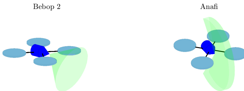
FIGURE 5.10 – Simplified representations of the feasible directions of recording of the Bebop 2 and the ANAFI
